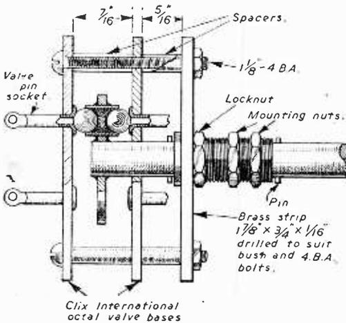
Main details of a rotary switch.
