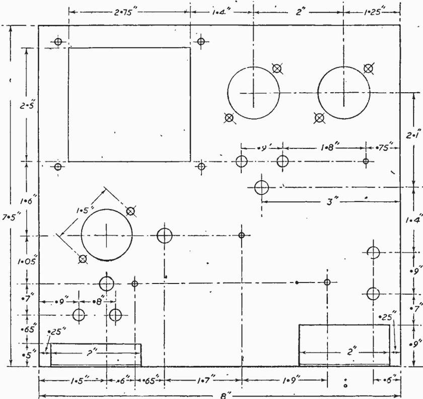
Fig. 6.—Drilling and cutting dimensions of the chassis.
