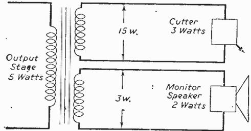
Fig. 3 (b).—Recording cutter and monitor are fed from individual windings, each taking a fixed percentage of output power (see text).
