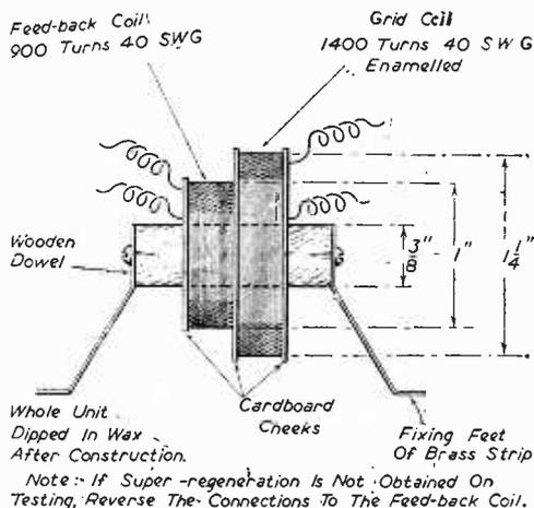
Fig. 7.—Full details of the quench coil.
