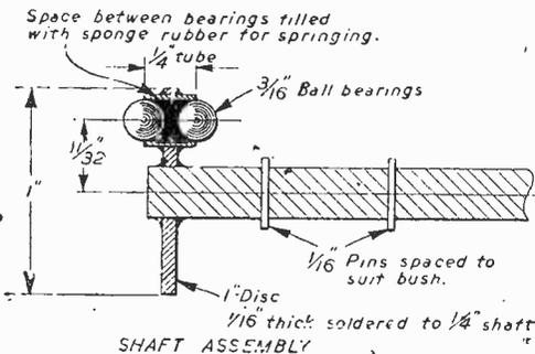
How the rotating contact is built up for the rotary switch.
