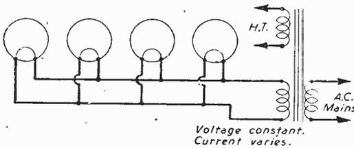
Fig. 1.—This is the normal A.C. heater-fed arrangement.
