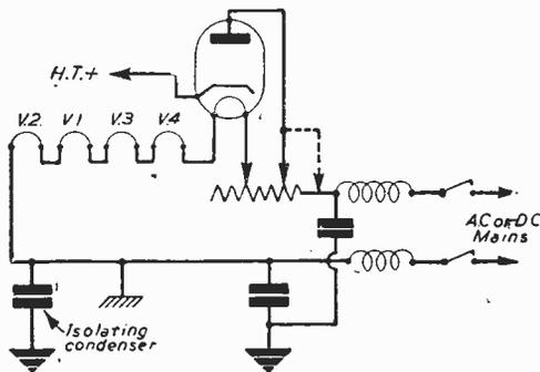
Fig. 4.—A more detailed circuit for A.C. or D.C. mains supplies showing the inclusion of H.F. filtering arrangements.
