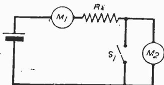
Circuit arrangement for measuring meter resistance.
