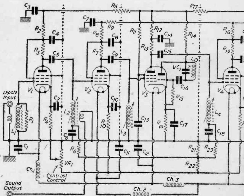
Fig. 1.—Theoretical circuit of the vision unit. A 1
