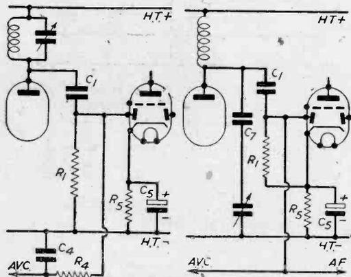
Fig. 8.—Typical A.V.C. diode circuit.
