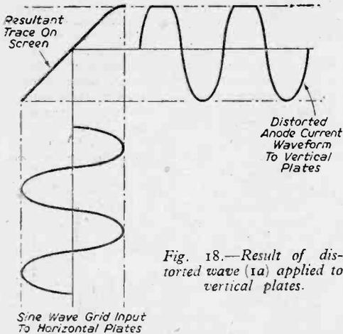
Fig. 18.—Result of distorted wave ( $I_a$ ) applied to vertical plates.
