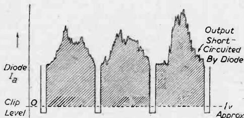
Fig. 2.—How the picture impulses are shortened and the negative pulses obtained.
