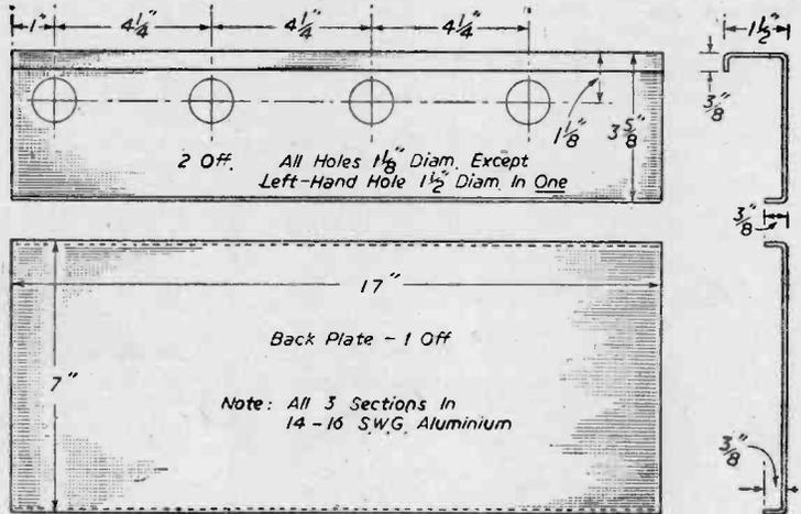
Fig. 3.—General details of the vision chassis sections.
