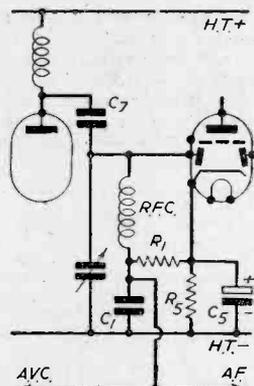
Fig. 10.—Modification of the circuit of Fig. 9 to include series-fed diode detector.
