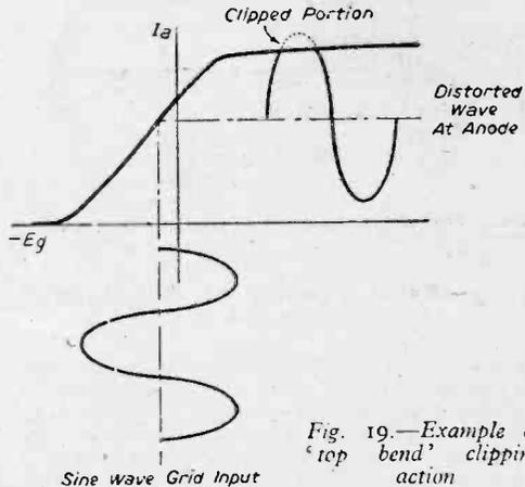
Fig. 19.—Example of 'top bend' clipping action
