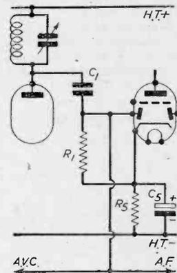
Fig. 7.—A shunt-fed diode detector connected in the anode circuit of an R.F. amplifier.
