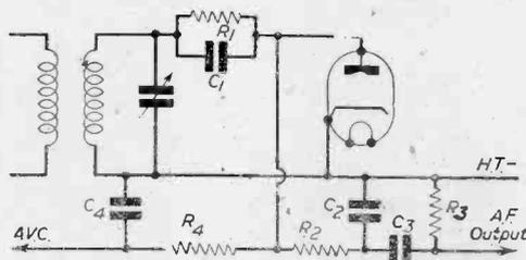
Fig. 3.—Practical circuit for a series-fed diode detector using a separate diode valve. Component values for high-quality M.W. reception are:  $R_1$ ,  $100k\Omega$ ,  $R_2$ ,  $50k\Omega$ ,  $R_3$ ,  $0.5M\Omega$ ,  $R_4$ ,  $1M\Omega$ ,  $C_1$ ,  $100pF$ ,  $C_2$ ,  $100pF$ ,  $C_3$ ,  $0.01\mu F$ ,  $C_4$ ,  $0.1\mu F$ .
