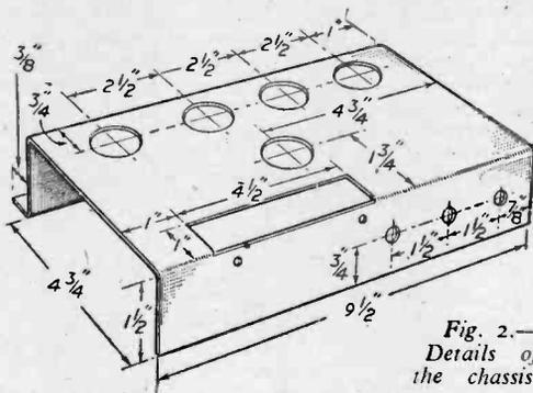
Fig. 2.—Details of the chassis.
