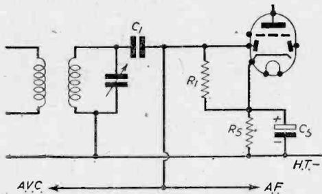
Fig. 5.—Practical circuit for a shunt-fed diode detector, using a double-diode-triode. Component values are the same as before and the circuit arrangement under the earth line is the same as in Figs. 3 and 4.
