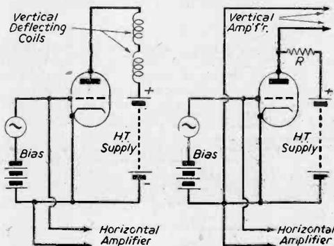
Fig. 16.—On the left (A) circuit for obtaining  $E_g|I_a$  curves when magnetic deflection is used, and at B (right) the modification required for electrostatic deflection.
