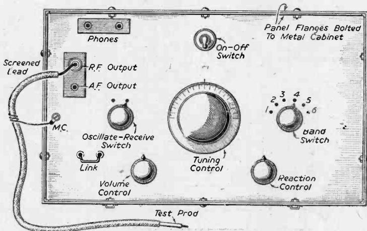
Fig. 7.—Panel layout and identity of the various controls.
