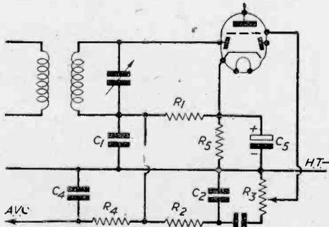
Fig. 4.—Practical circuit for a series-fed diode detector, using a double-diode-triode. Component values are given in the table in Fig. 3.
