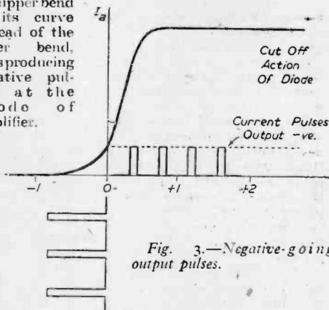
Fig. 3.—Negative-going output pulses.
