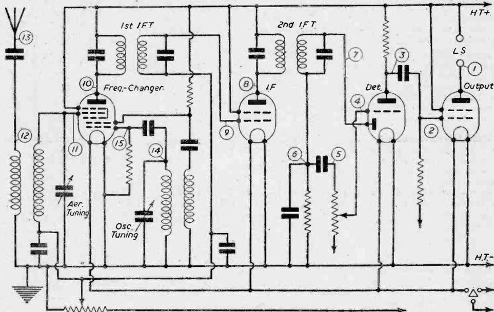
Fig. 8.—Testing points in a standard superhet. 1-6 are A.F., 7-10 I.F., 11-13 R.F. and 14-15 oscillator.
