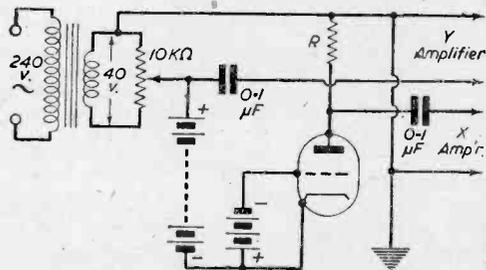
Fig. 22.—Circuit for taking  $I_a/E_a$  curves,
