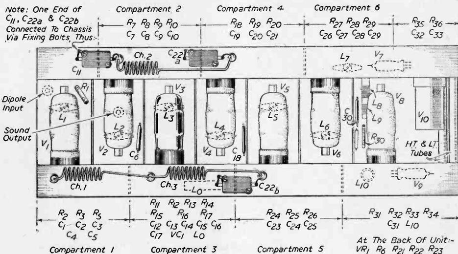
Fig. 2.—Chassis layout showing components wired in the separate compartments.
