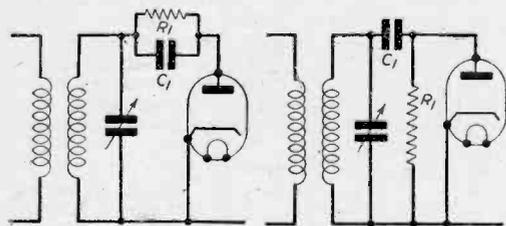
Fig. 1.—Fundamental circuit of series-fed diode detector.
