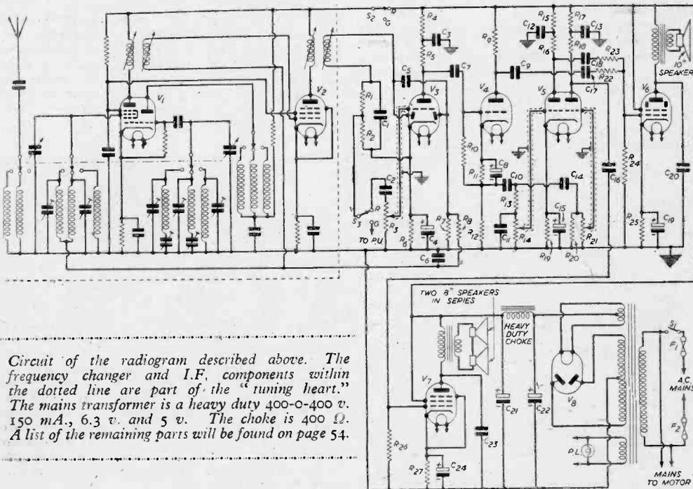
Circuit of the radiogram described above. The frequency changer and I.F. components within the dotted line are part of the "tuning heart." The mains transformer is a heavy duty 400-0-400 v. 150 mA., 6.3 v. and 5 v. The choke is 400 Ω. A list of the remaining parts will be found on page 54.
