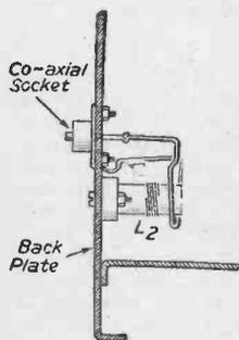
Fig. 6.—The sound pick-up loop wound over L2.
