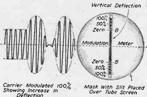
Fig. 15.—Method of masking tube and obtaining modulation indications.
