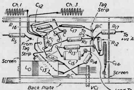
Fig. 4.—Layout of the frequency-changer stage. In this illustration the parts appear more spaced out than they are in practice.
