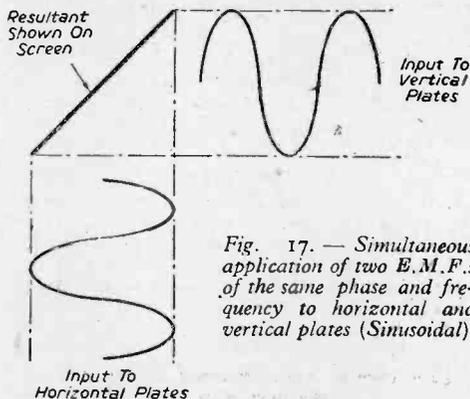
Fig. 17.— Simultaneous application of two E.M.F.s of the same phase and frequency to horizontal and vertical plates (Sinusoidal).
