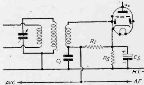
Fig. 6.—Practical circuit for a series-fed diode detector, using a double-diode-triode in which the tuning capacitor may be earthed.
