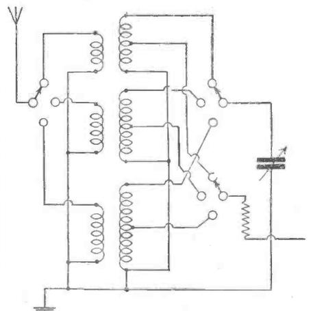
Fig. 2.—How to arrange wave-change switching
