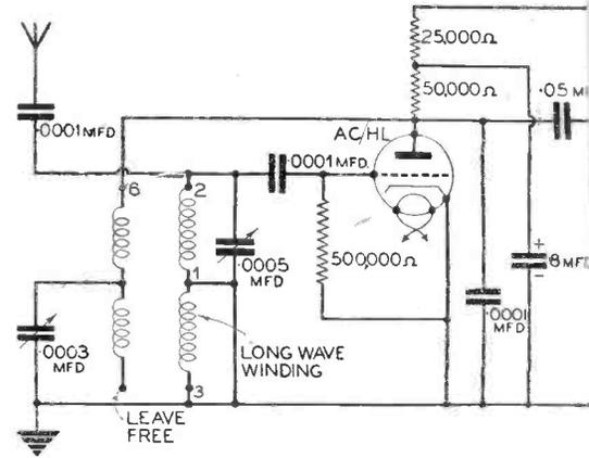
Fig. 2.—Circuit diagram of a suggested detector unit for use with the amplifier.
