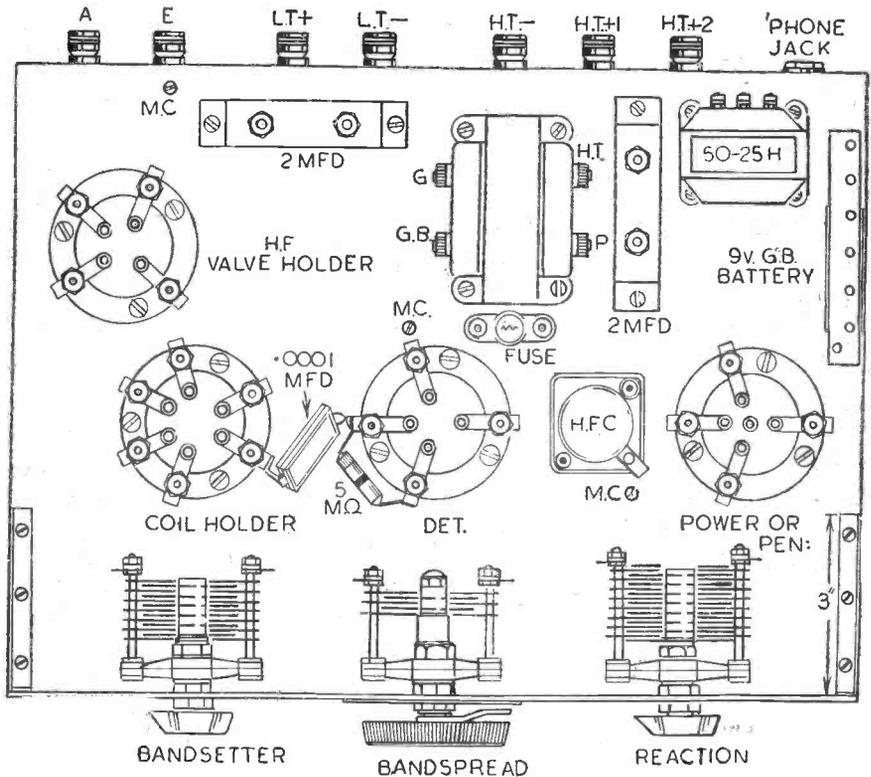
Fig. 3.—Diagram showing layout of chassis components.
