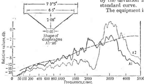
Fig. 2.—Comparison of diaphragms A1 and A2.
