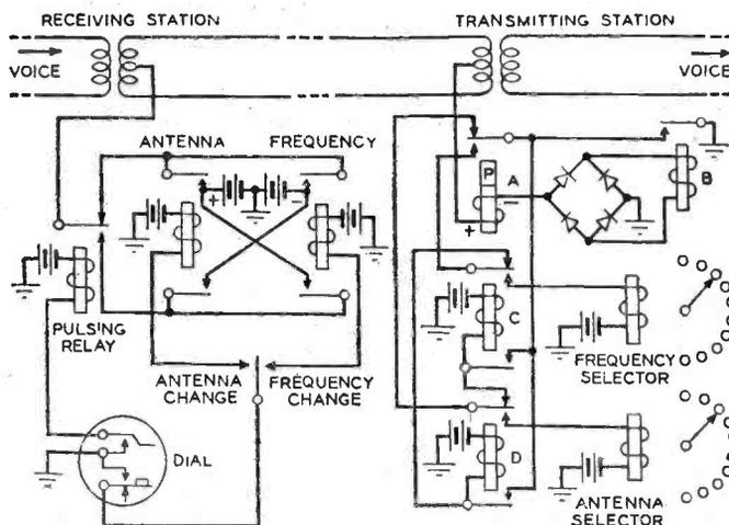
Fig. 2.—Simplex dialing circuit used for selecting frequencies and aerials at Miami.
