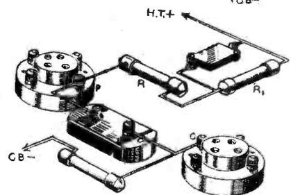
Fig. 3.—A bass booster for an R.C. coupled circuit.
