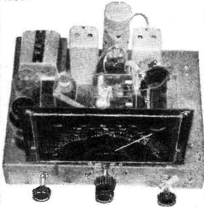
**MODEL AW38.** 8-valve All-wave Super-heterodyne chassis. This All-wave Radiogram chassis has resistance capacity coupled push-pull output capable of handling 6 watts, and gives good quality reproduction on both radio and gramophone, for an economical price of 8 gns. Plus 5% war increase.
