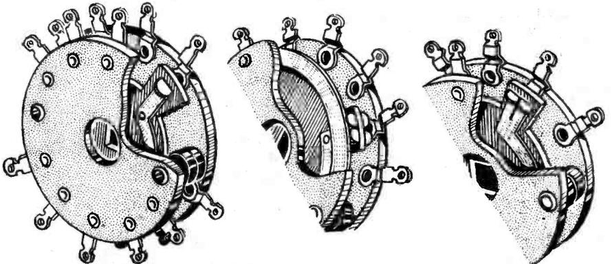
Fig. 11.—How the rotary switches (Fig. 9) are designed. Three different patterns are shown.
