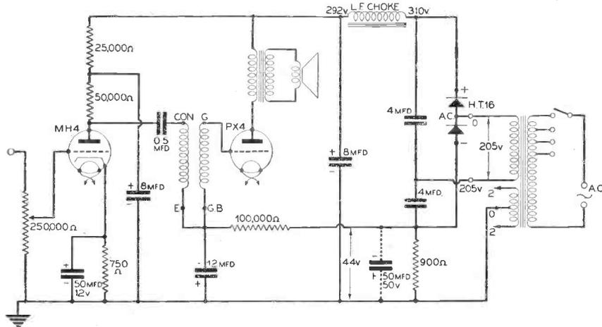
Fig. 1.—Theoretical circuit diagram of the amplifier.
