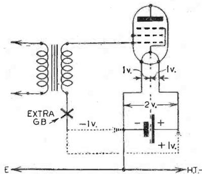
Fig. 1.—It is possible to use the voltage drop across the filament to provide a small amount of bias—although not half the L.T. voltage.
