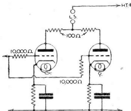
*It is sometimes satisfactory to replace a large output valve by two similar smaller valves in parallel. They should be decoupled, and this diagram shows how this can be done adequately.*
