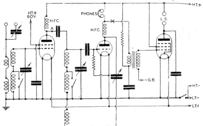
Fig. 2.—Points for checking in a standard 3-valve circuit.
