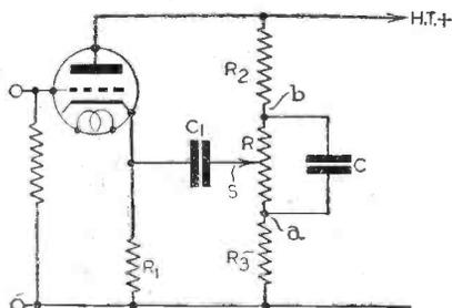
Fig. 11.—A single-stage amplifier circuit in which bass boost is provided.
