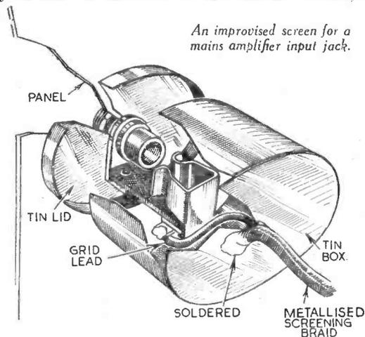
An improvised screen for a mains amplifier input jack.
