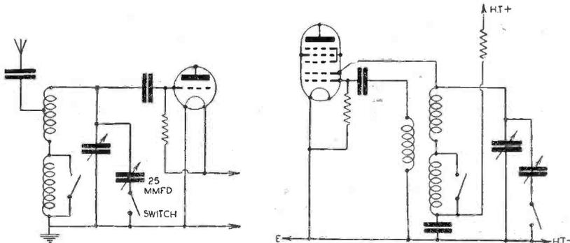
Fig. 1.—Band-spread tuning can be applied to most receivers by connecting a 25mmfd. condenser in series with an on/off switch, across the principal tuning condenser. This will, of course, affect dial readings on short waves.
