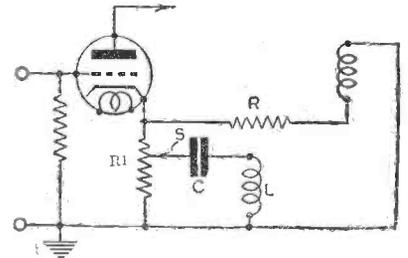
Fig. 8.—In this circuit the cathode resistance is provided with a sliding contact.
