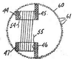
Fig. 3.—Arrangement of the end of the frame aerial windings.
