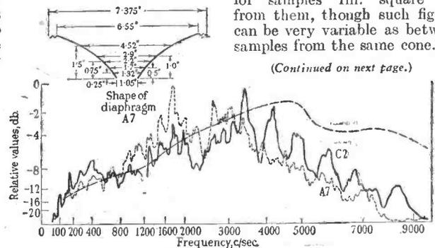
Fig. 5.—Comparison of diaphragms C2 and A7.
