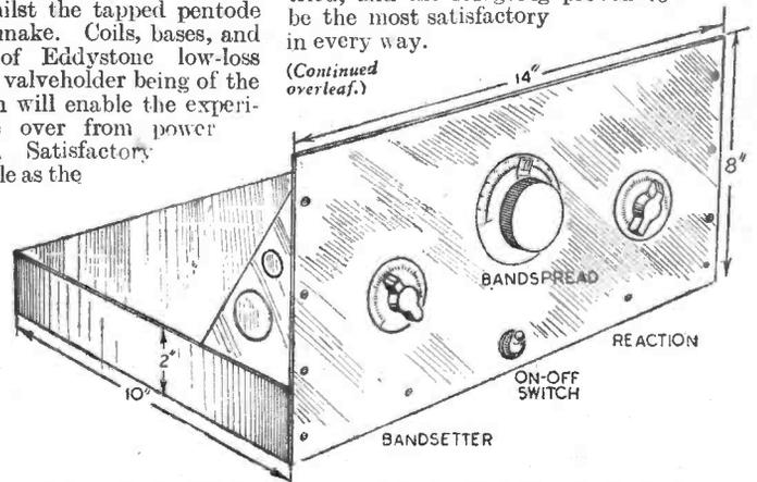
Fig. 2.—Chassis and panel assembly, showing the layout of panel components.
