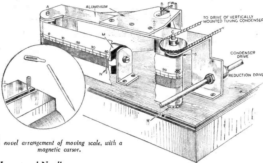
A novel arrangement of moving scale, with a magnetic cursor.
