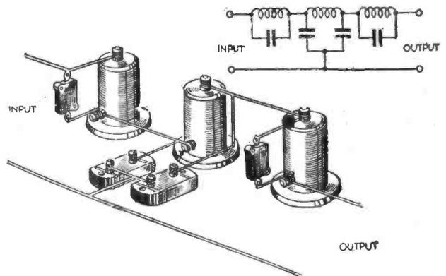
Fig. 9.—One arrangement of gramophone scratch filter.
