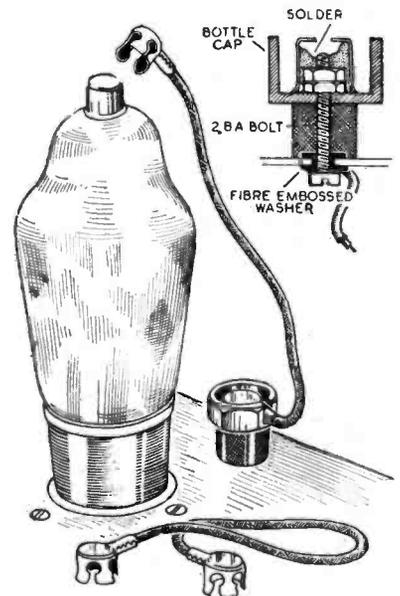
A method of ensuring safety for T.C. connections.
