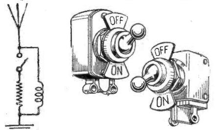
Fig. 5.—A "local-distance" switch and the circuit arrangement.
