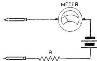
Fig. 1.—Circuit of a test meter showing range-increasing resistance R.
