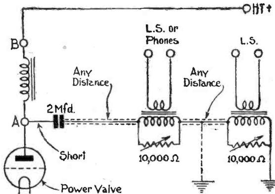
Fig. 2.—Adding a loudspeaker (or loudspeakers) to any receiver—particularly those without built-in units.
