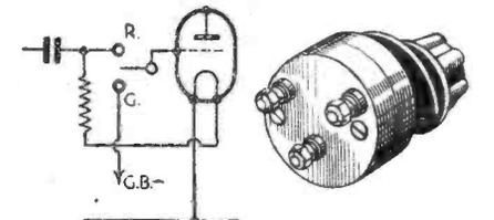
Fig. 8.—A single-pole change-over switch for radio-gram switching.
