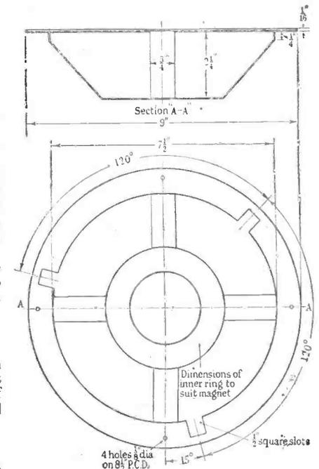
Fig. 7.—Suggested construction of the speaker frame.
