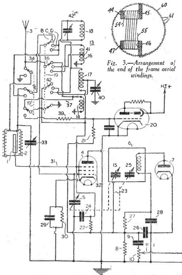
Fig. 1.—Circuit of part of a receiver incorporating the frame aerial.
