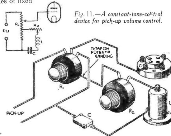
Fig. 11.—A constant-tone-control device for pick-up volume control.
