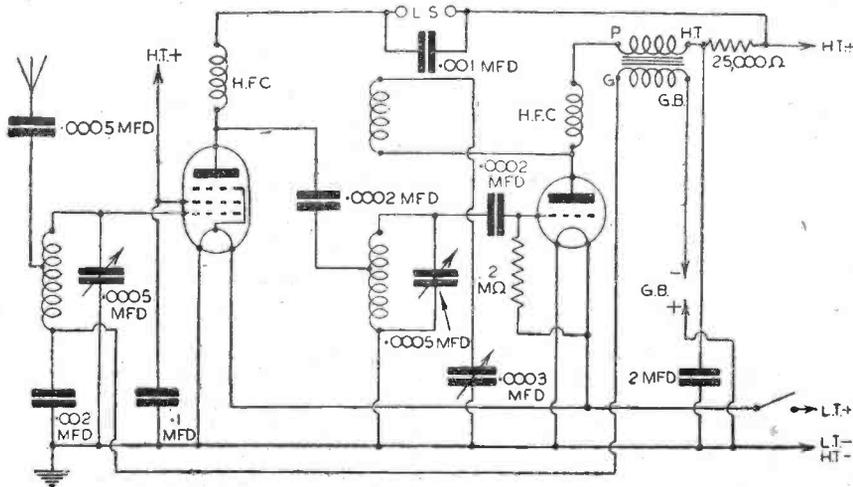
Fig. 3.—A modern version of an old-type reflex circuit, using a triode detector.
