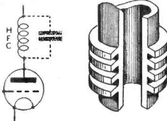
Figs. 1 and 3.—Self-capacity can be likened to a small condenser across the winding, as shown on the left. A typical slotted former often used for the winding of the L.W. section is shown on the right.
