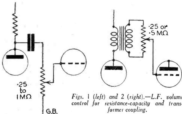
Figs. 1 (left) and 2 (right).—L.F. volume control for resistance-capacity and transformer coupling.
