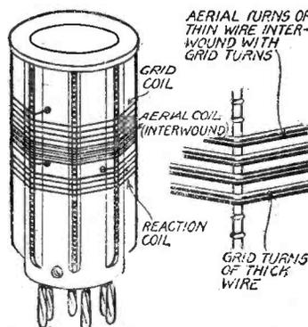
A modern type of S.W. coil showing aerial, grid and reaction windings.
