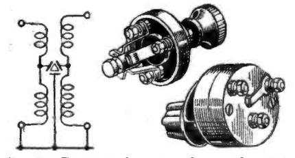
Fig. 2.—For wave-change switching, a three-point switch is often employed.
