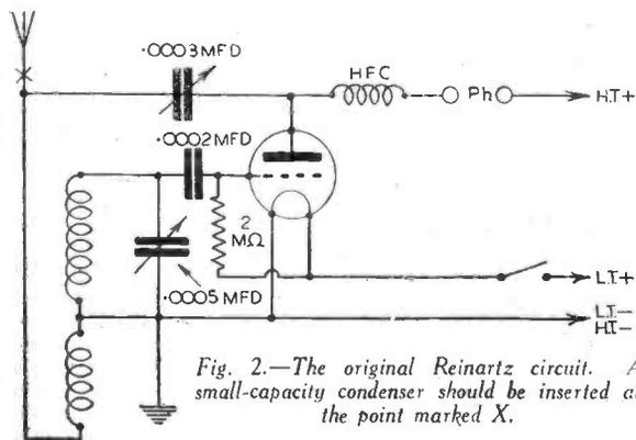
Fig. 2.—The original Reinartz circuit. A small-capacity condenser should be inserted at the point marked X.
