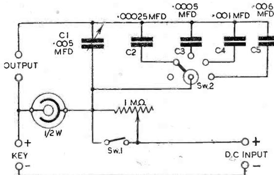
Fig. 1.—Wiring diagram of the simple Neon-tube test unit. Either batteries or external power pack may be applied.
