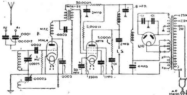
Fig. 1.—Theoretical circuit diagram of the A.C. Two-valver.
