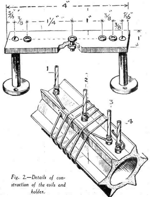
Fig. 2.—Details of construction of the coils and holder.
