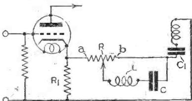
Fig. 7.—Series connection for the counter coupling.
