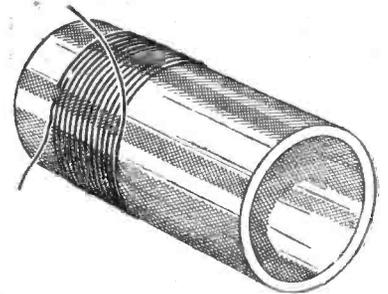
Fig. 2.—An example of single layer solenoid winding not difficult to construct.
