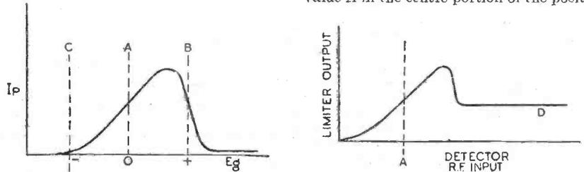
Fig. 2 and 3.—Control grid potential-anode current characteristics, and limiter output curve respectively.
