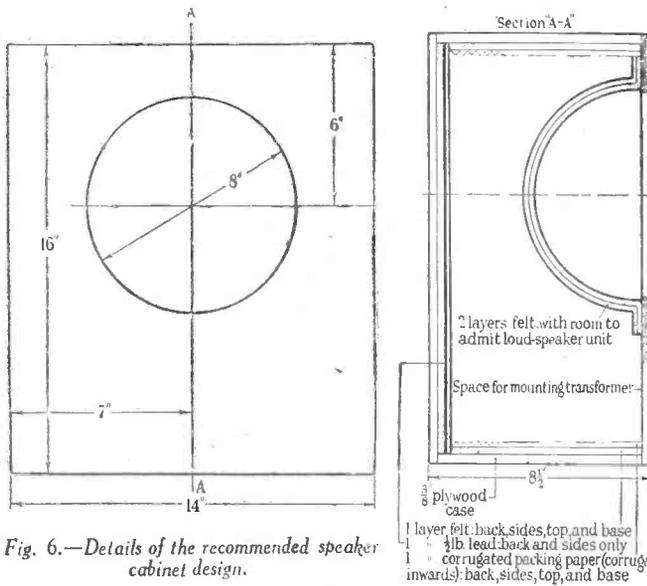
Fig. 6.—Details of the recommended speaker cabinet design.
