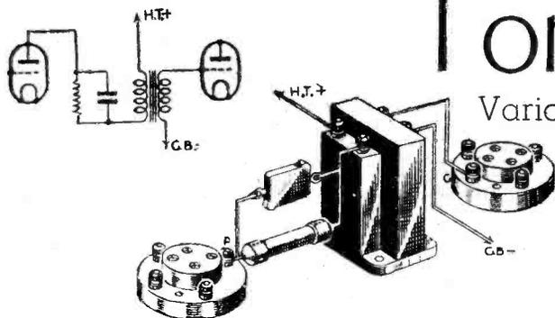
Fig. 1.—A device for cutting bass in a transformer-coupled amplifier.
