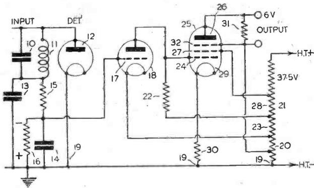
Fig. 1.—A circuit incorporating a tuned input and a limiter arrangement as described in the text.
