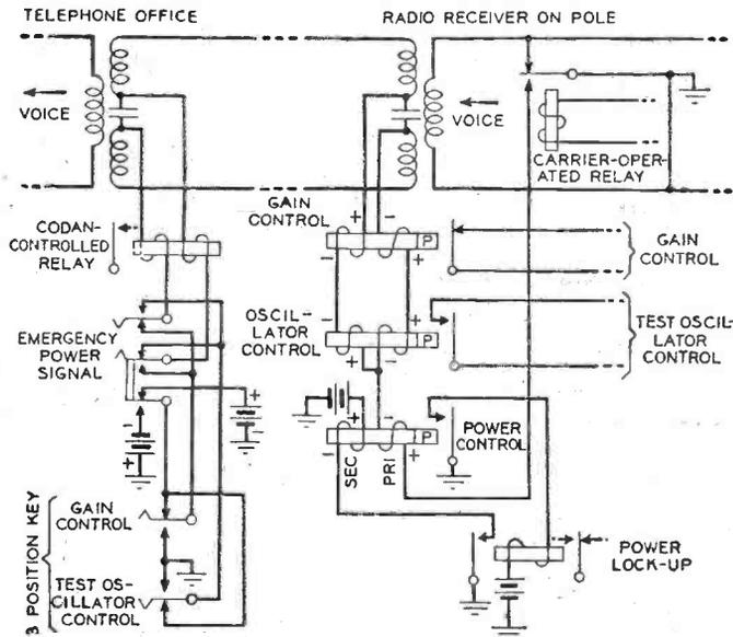
Fig. 3.—Control circuit for 223A radio receiving equipment.
