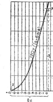
Fig. 2.—The anode-current grid-volts curve mentioned in the article. Note cut-off point and the effect of negative bias.
