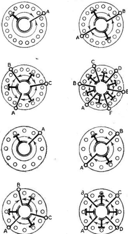
Fig. 12.—Connections available for the type of switch shown in Fig. 10.
