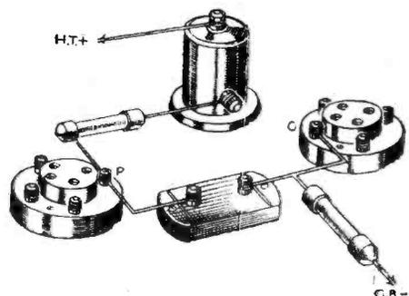
Fig. 4.—The arrangement for a simple treble booster.
