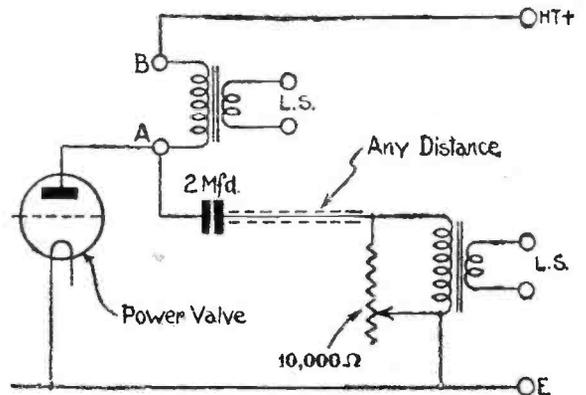
Fig. 1.—Circuit diagram showing how an additional loudspeaker can be added to a commercial set with built-in speaker.
