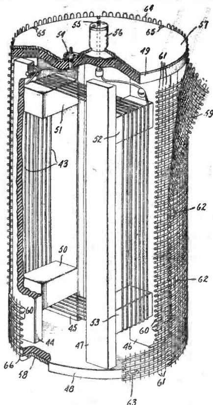
Fig. 2.—Constructional details of the frame aerial.
