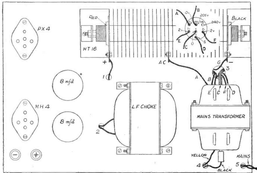
Inset on the metal rectifier are the code connections for the transformer end plate.
