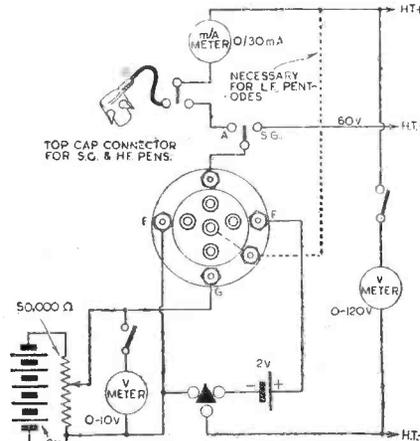
Fig. 1.—A suggested circuit for a simple valve tester. Refinements can be added to suit requirements.
