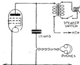
Fig. 2.—A satisfactory method of connecting 'phones and fitting a speaker cut-out switch.
