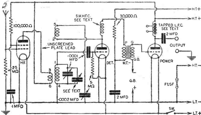
Fig. 1.—Theoretical circuit diagram of the three-valve receiver described in the text.
