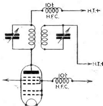
*Small, 10-turn H.F. stopper chokes will often prevent instability when wired in the anode and/or screening grid circuit of a frequency changer or H.F. pentode.*
