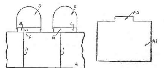
Figs. 1 and 2.—Screening boxes, and detail of screening partition.
