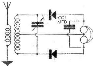
Fig. 4.—One of many full-wave-detector circuits which were tried with little success.
