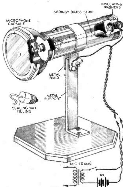
An old torch case is utilised for making this microphone.
