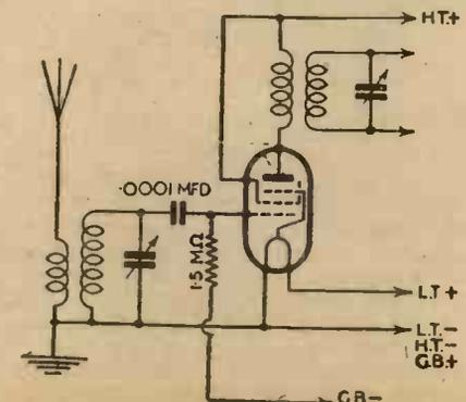
Fig. 5.—Improved circuit for variable-mu control.
