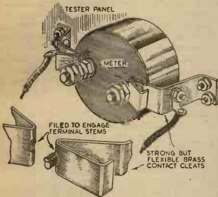
A meter holder which allows for the quick removal of the instrument, when necessary.
