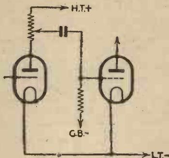
Fig. 9.—L.F. volume control by variable anode resistance.
