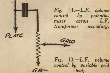
Fig. 10.—L.F. volume control by variable grid leak.
