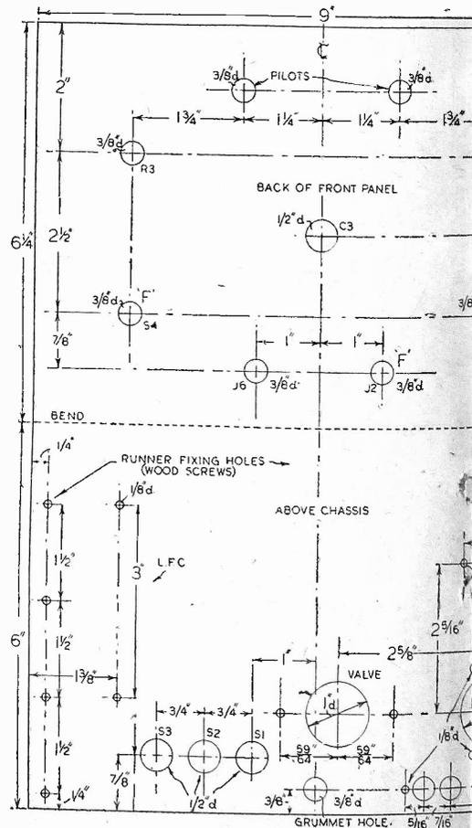
Fig. 4.—Drilling dimensions of the chassis
