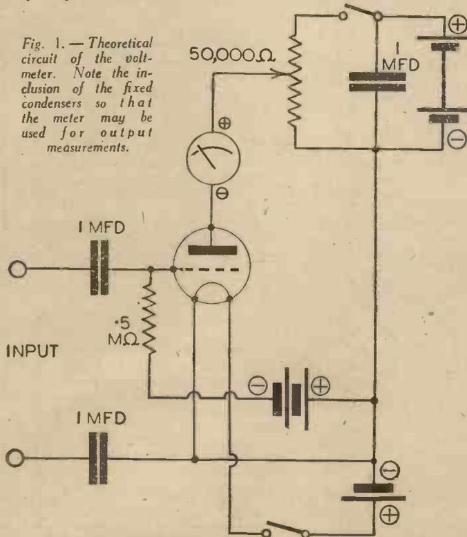
sufficient in many cases. The exact value may be found on trial with the particular valve you decide to use. In order to adjust the H.T. and obtain a suitable zero-setting
