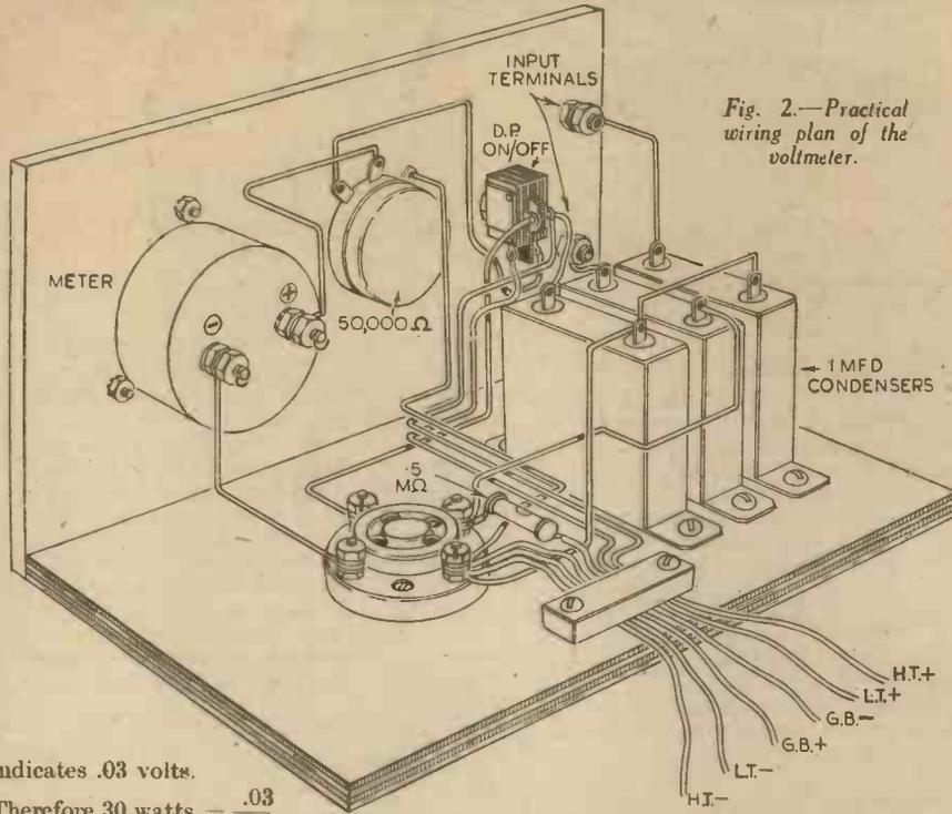
Fig. 2.—Practical wiring plan of the voltmeter.
