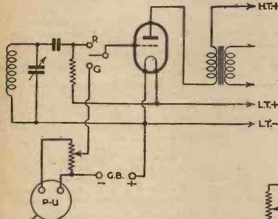
Fig. 8.—Volume control for pick-up in radiogram combination.
