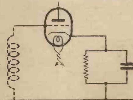
Fig. 6.—Automatic bias is obtained by a resistance and condenser in the cathode lead.
