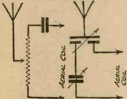
Fig. 1 (Left).—Using a potentiometer form of input control. As an alternative, the arm of the potentiometer may be joined to earth, instead of one end, thus providing a resistance control. Fig. 2 (Right).—A "capacity" potentiometer or differential condenser as input control.
