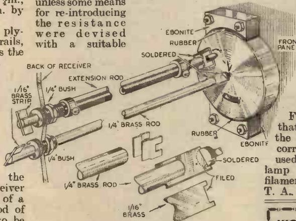
Extension controls for a time-piece fitted to a radio set.
