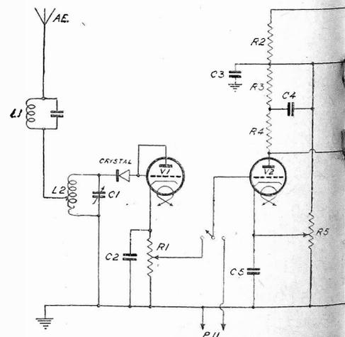
Fig. 2.—Complete circuit diagram of the receiver system.
