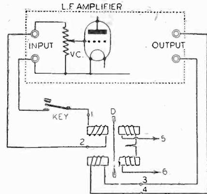
Fig. 4.—Circuit diagram showing the use of the oscillator and keying system.
