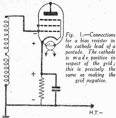
Fig. 1.—Connections for a bias resistor in the cathode lead of a pentode. The cathode is made positive in respect of the grid; this is precisely the same as making the grid negative.
