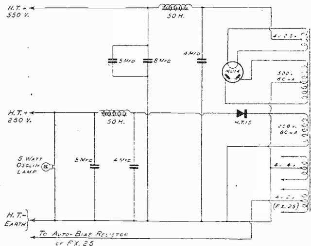
Fig. 3.—Mains section of the receiver, showing the separate H.T. feeds.
