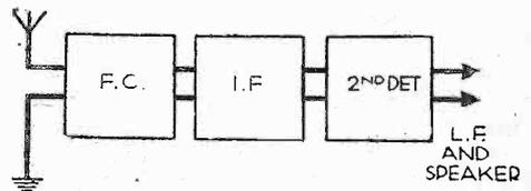
Fig. 2.—Essential parts of a superhet, where rectangles are used to indicate the stages.
