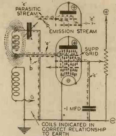
Fig. 2.—Diagram showing the path of electrons in the suppressor-grid system of reaction.
