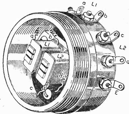
Fig. 2.—How the earpiece was split up and provided with terminals in a further stage of development.
