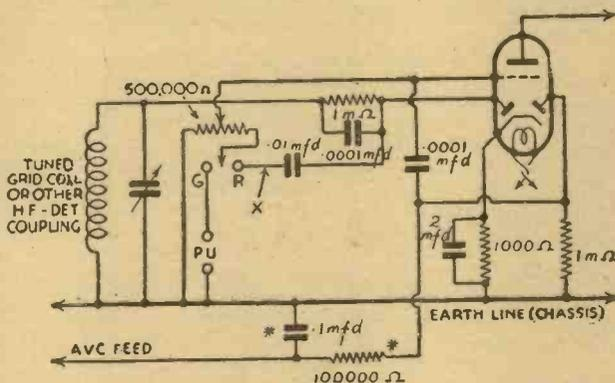
Fig. 2.—The double-diode-triode, arranged for A.V.C. with delay in a "straight" receiver, and fitted for reproducing gramophone records. A filter may be required at "x" in sets inclined to instability. Components marked \* are liable to modification.
