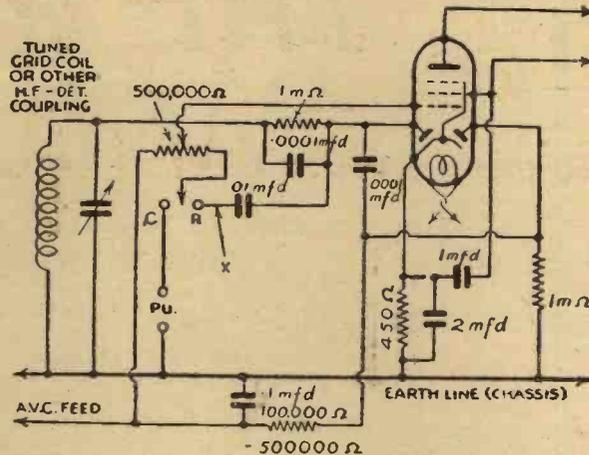
Fig. 5.—The double-diode-pentode for corrected and delayed A.V.C. with the addition of gramophone switch and terminals. Connections to anode and extra grid are normal. An H.F. filter may be desirable at "x" in some cases.
