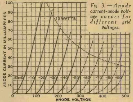
Fig. 3.—Anode current-anode voltage curves for different grid voltages.
