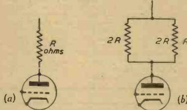
Fig. 1.—Showing the division of power in the anode circuit by two loads in parallel.
