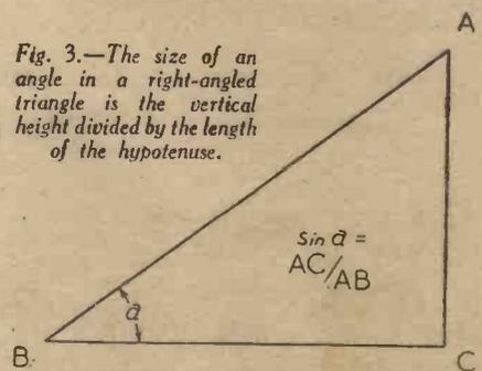
Fig. 3.—The size of an angle in a right-angled triangle is the vertical height divided by the length of the hypotenuse.
