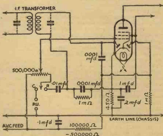
Fig. 4.—A pick-up added to the double-diode-pentode, arranged for delayed and corrected A.V.C. in a superhet. Connections to anode and extra grid are normal and not changed by the addition of the pick-up.
