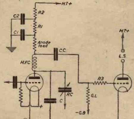
Fig. 6.—With resistance-capacity coupling, care must be taken to see that R3 is wired in the correct position relative to the G.L.
