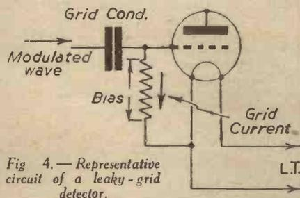
Fig. 4.—Representative circuit of a leaky-grid detector.
