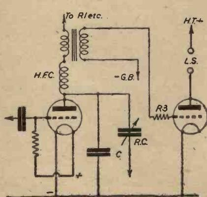
Fig. 5.—Showing the position of the grid H.F. stopper resistance R3 in a transformer-coupled stage.
