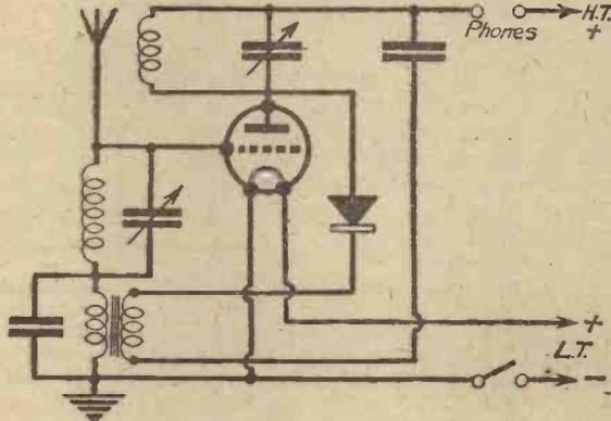
Fig. 4.—An early form of valve-crystal reflex circuit.
