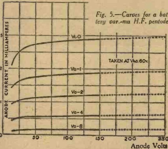
Fig. 5.—Curves for a battery var.-mu H.F. pentode.
