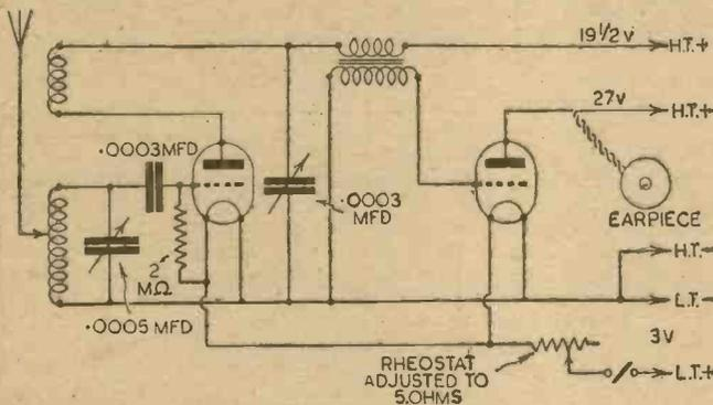
Fig. 1.—Theoretical circuit diagram of the simple midget portable described in the text.
