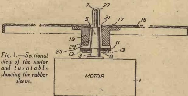
Fig. 1.—Sectional view of the motor and turntable showing the rubber sleeve.
