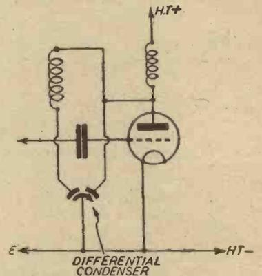
Fig. 2.—A fairly uniform anode-to-earth capacity is obtained by using a differential reaction condenser.
