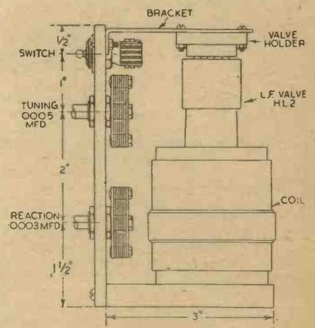
Fig. 3.—Side view, showing valve-holder bracket which supports the L.F. valve within the coil.
