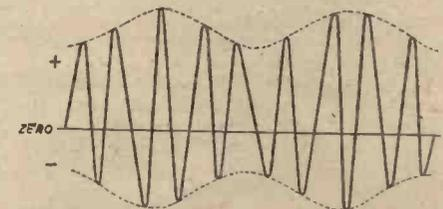
Fig. 8.—This shows the output from a detector by a method of detection which displaces the zero voltage line so that the negative amplitude of the output is 50 per cent. of the positive (refer to Fig. 4).
