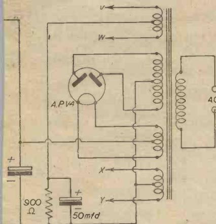
main section using a valve rectifier.
