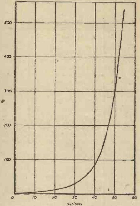
Fig. 1.—Graph showing the gain or loss ratios in relation to decibel equivalents.
