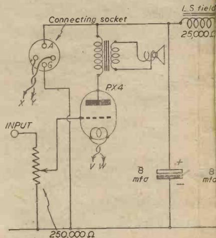
Fig. 5.—Alternative amplifier and power section.
