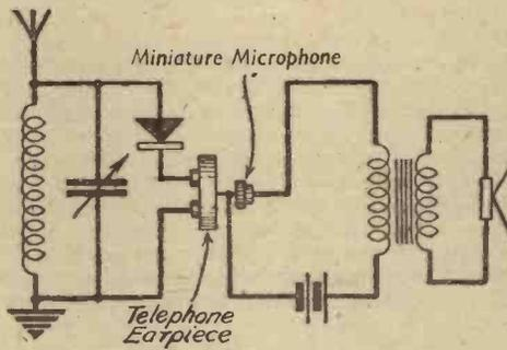
Fig. 3.—The arrangement of a microphone amplifier for operating a loudspeaker from a crystal set.
