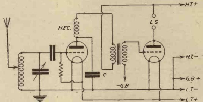
Fig. 2 (Above).—H.F. choke and by-pass condenser have been added to restrict the flow of H.F.
