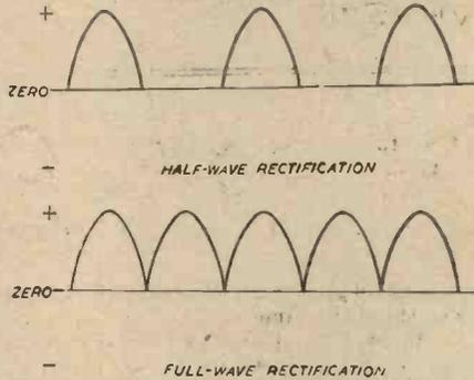
Figs. 1 and 2.—These curves show the effect of half-wave and full-wave rectification.
