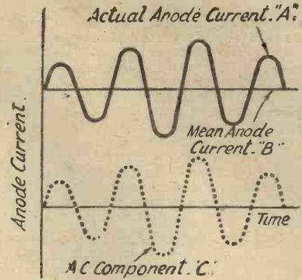
Fig. 3.—The steady or mean output current with the alternating component superimposed.
