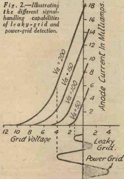
Fig. 2.—Illustrating the different signal-handling capabilities of leaky-grid and power-grid detection.
