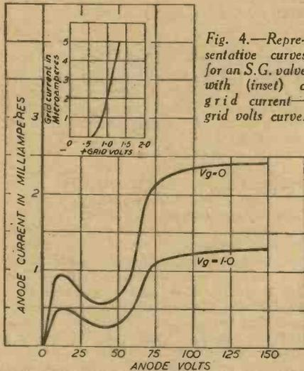
Fig. 4.—Representative curves for an S.G. valve with (inset) a grid current—grid volts curve.
