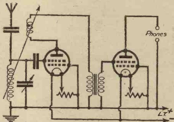
Fig. 8 (right).—Circuit of a two-valve set—L.F. high-tension-less receiver.
