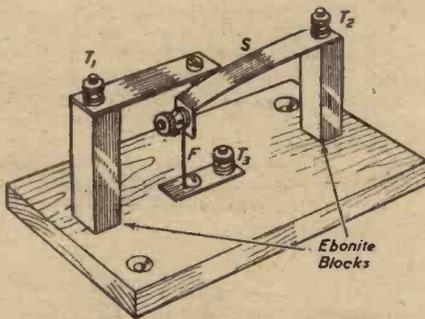
A novel switching arrangement for emergency lighting.
