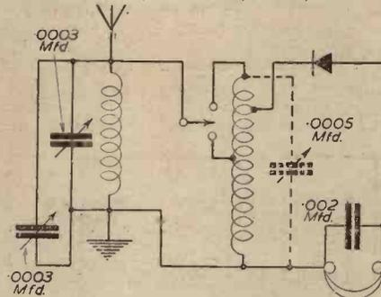
Circuit diagram of Mr. A. S. Long's crystal set. Wave Trap Coil; 60 turns 30 S.W.G. enamelled copper wire on a former 1½in. diameter. Aerial Detector Coil; 76 turns of 30 S.W.G. enamelled copper wire on a former 2½in. diameter. Crystal tap at 10 turns. Aerial tap at 40 turns. Variable condensers preferably ganged, .0003 or .0005 mfd. The .0005 tuning condenser is not required, as in the 150 mile circuit, the wave-trap serves the same purpose.
