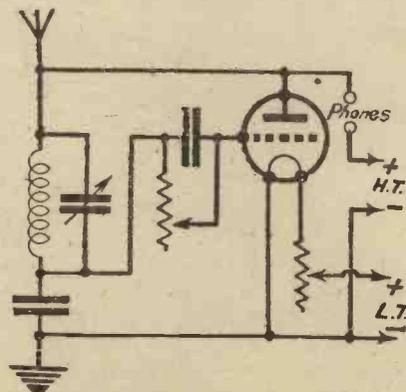
Fig. 9.—The Ultra-Audion, a tricky but interesting single-valve "super" circuit.
