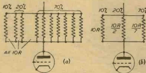
Fig. 2.—Unequal distribution of power obtained by grouping load resistances.
