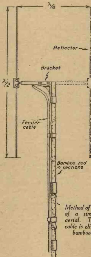
*Method of construction of a simple dipole aerial. The feeder cable is clipped to the bamboo support.*
