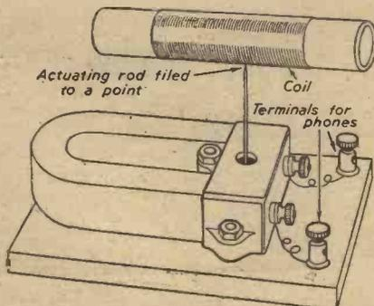
An improvised counter for fine coil windings.
