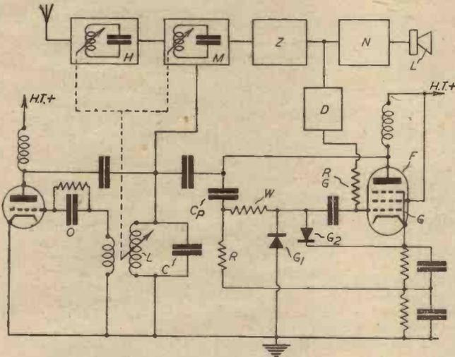
Fig. 1. (Left).—A usual arrangement of the pull-in tuning circuit.
