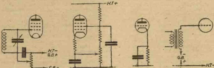
Fig. 2.—Alternative methods of biasing mains and battery H.F. and L.F. valves.
