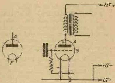
The electrode arrangements for the diode (left) and the triode (right) are shown here.
