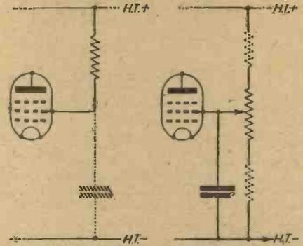
Fig. 1.—Alternative methods of feeding the screen-grid of a pentode valve.
