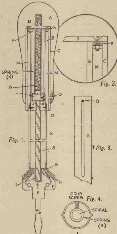
Sectional view and details of a spiral screwdriver.
