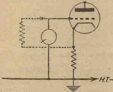
Fig. 2.—Normal connections for a pick-up in an indirectly-heated valve. If a detector, the grid leak is connected as shown by the broken lines.
