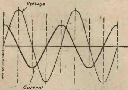
Fig. 4.—In an A.C. circuit containing a series capacity, the current "leads" the voltage by 90°.
