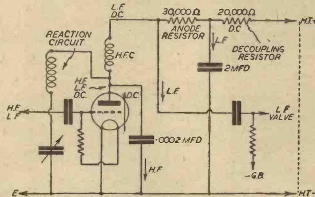
Fig. 1.—The anode circuit of a triode detector, with R.C.C. coupling, affords a good example of combined D.C., H.F., and L.F. currents.
