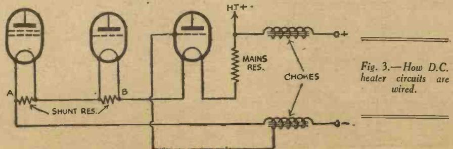
Fig. 3.—How D.C. heater circuits are wired.
