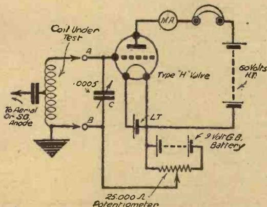
A simple method of comparing the efficiency of coils.
