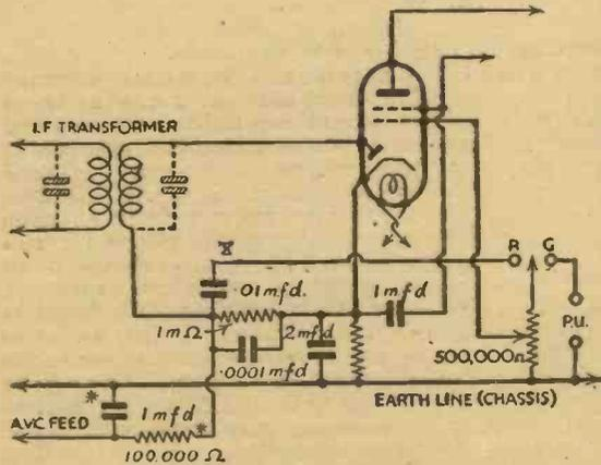
Fig. 3.—The single-diode-tetrode for A.V.C. and gramophone reproduction. The arrangement shown is suitable for use in a superhet. Connections to anode and screen are normal. An H.F. filter may be necessary at "x" in certain circuits. Components marked \* are liable to modification. Value of bias resistor varies widely with different makes of valve. That recommended by valve maker should be used.
