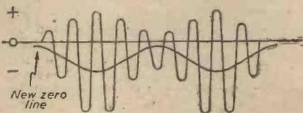
Fig. 5.—After detection by a leaky-grid "detector," the curve shown in Fig. 3, is modified to the form shown above. Thus the "mean" (corresponding to the modulation) is able to affect the anode circuit.
