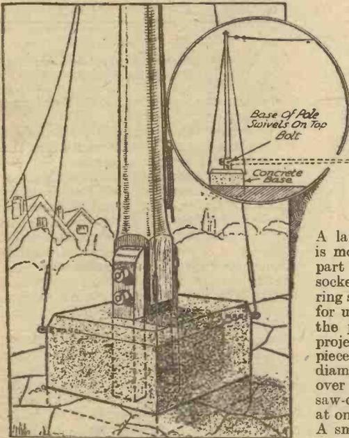
Method of mounting an aerial in a concrete block—the mast supports could project through the underside of the block and into the ground for some distance.—S. PARKER (Pinner).
