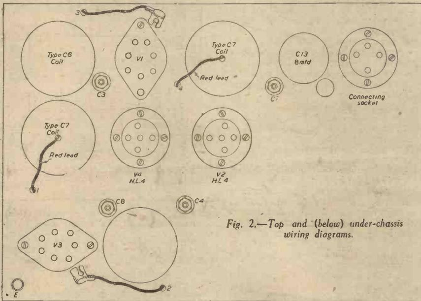
Fig. 2.—Top and (below) under-chassis wiring diagrams.
