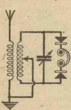
Fig. 2.—A crystal receiver using full-wave rectification.
