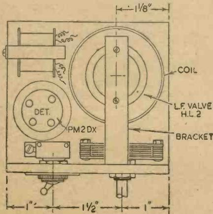
Fig. 2.—Plan view, showing lay-out of coil, valve-holders, and transformer.
