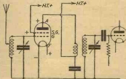
Note how the second grid is inserted in the S.G. valve.
