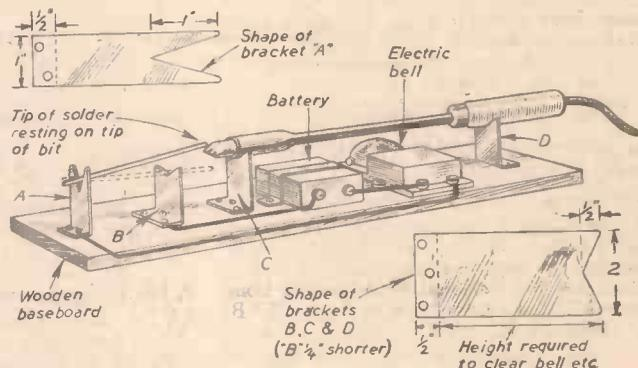
Details of the automatic switch for an electric soldering iron.
