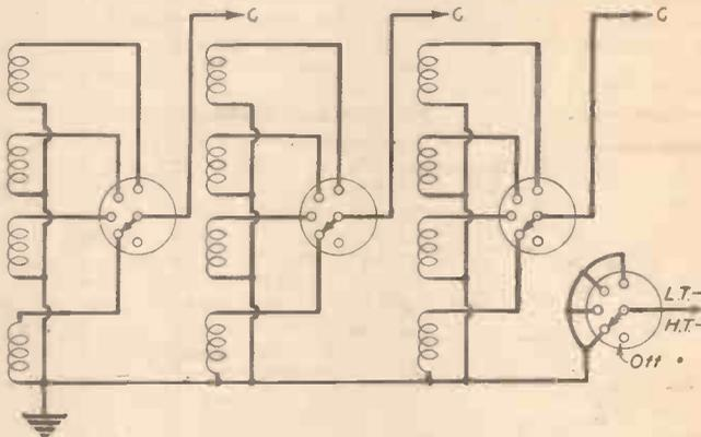
Fig. 5.—Four five-way rotary switches for on-off and wave-change switching in a four-range receiver with three tuning circuits. Various slightly-modified types of switch may be used, but separate units are to be preferred if the coils are not close together.
