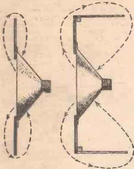
Fig. 1.—Showing the path taken by the surrounding air when movement of the cone takes place.
