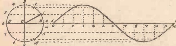
Fig. 2.—How to draw a curve representing harmonic motion. This is called a sine curve and is one of the two most important in wireless.
