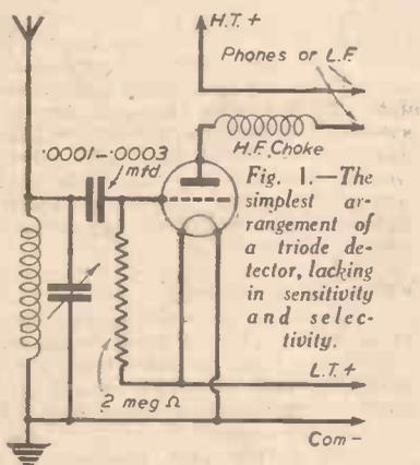
Fig. 1.—The simplest arrangement of a triode detector, lacking in sensitivity and selectivity.
