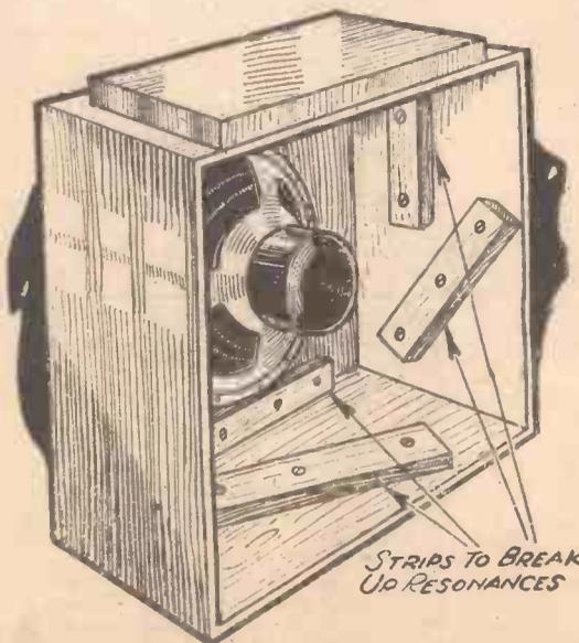
Fig. 2.—A simple method of overcoming box and cabinet resonances. The number and length of strips will depend on cabinet construction.
