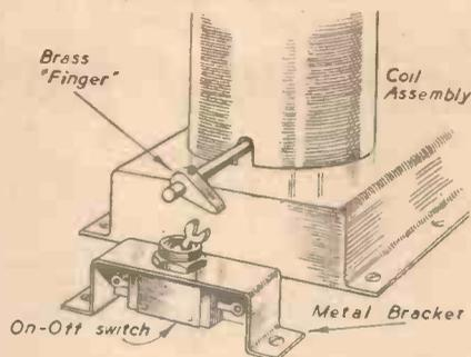
Fig. 4.—A method of operating a toggle on-off (battery or mains) switch from the spindle of built-in wave-change switches.
