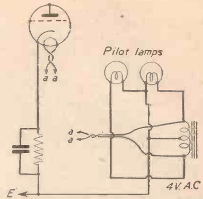
Fig. 2.—Small 3.5-volt flashlamp bulbs, used as pilot lights, may be wired as shown above. If they were merely in series, failure of either bulb would cause both lights to go out.
