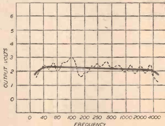
Fig. 2.—Response curve. The real curve will be as shown by the broken line, but this is generally levelled off and represented as shown by the heavy line.
