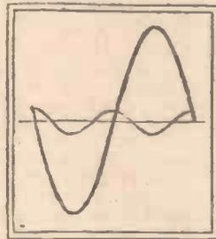
Fig. 3.—Sine curve representing simple harmonic motion together with another curve representing the second harmonic.
