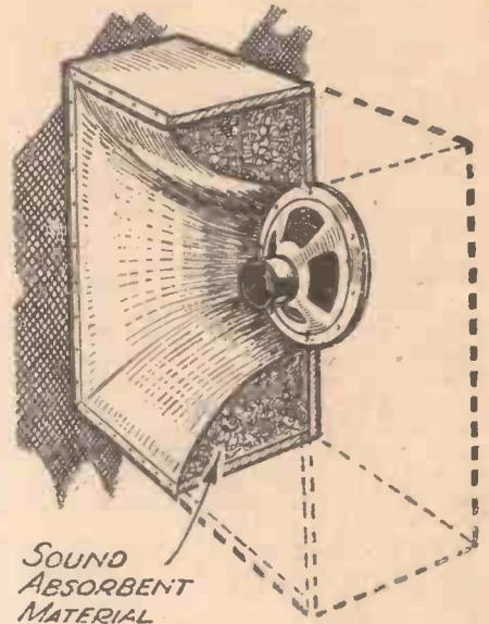
Fig. 3.—One of the best arrangements, provided care is taken with the actual packing and shaping of the absorbent material.
