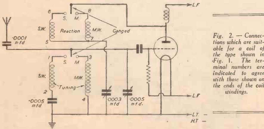
Fig. 2.—Connections which are suitable for a coil of the type shown in Fig. 1. The terminal numbers are indicated to agree with those shown on the ends of the coil windings.
