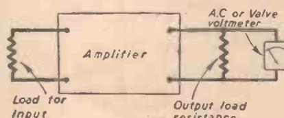
Fig. 3.—Set-up of equipment for measuring the noise level of an amplifier.
