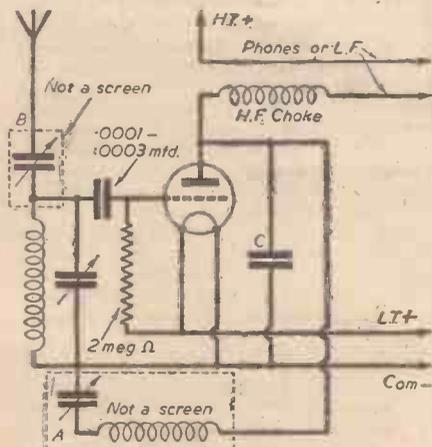
Fig. 2.—A more familiar and likewise more efficient one-valve circuit.
