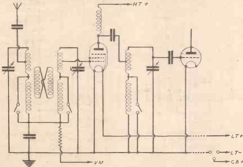
Fig. 1.—A simple H.F. arrangement with band-pass where three wave-change switches are used.
