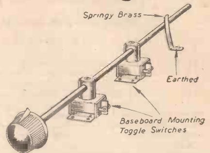
Fig. 2.—How baseboard-mounting toggle switches can be used for a circuit of the type shown in Fig. 1. Only two of the three switches are shown, but any number could be ganged together.
