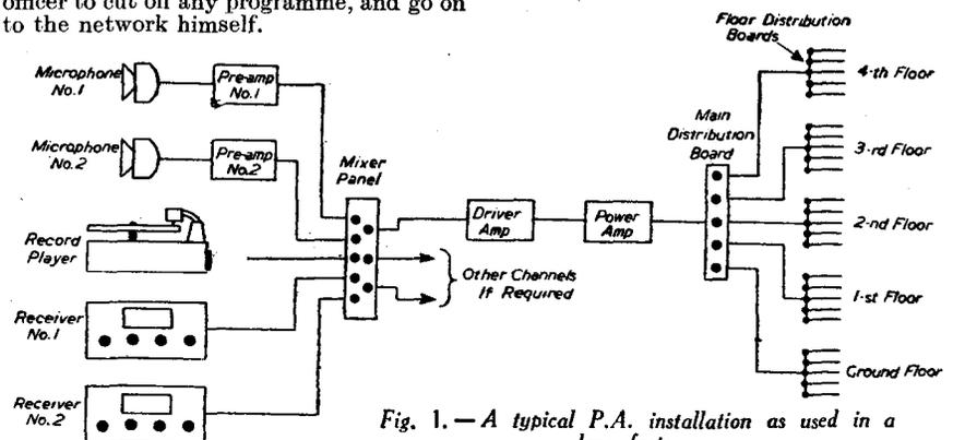
Fig. 1. - A typical P.A. installation as used in a large factory.
