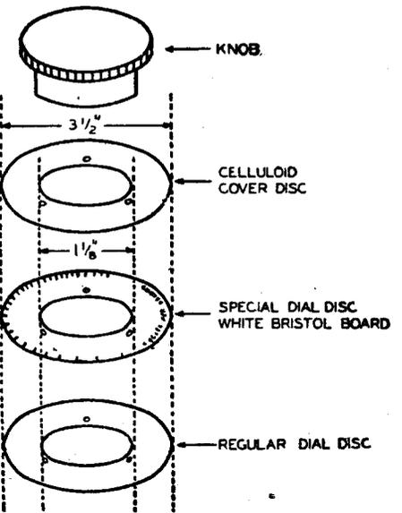
Fig. 6.—Method of making a direct-reading dial.
