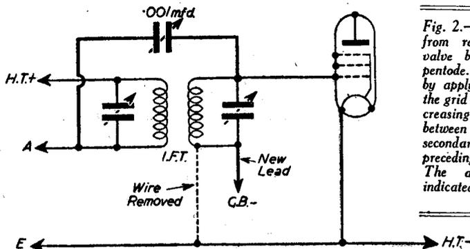
Fig. 2.—I.F. instability resulted from replacing an old S.G. valve by a new V.M. H.F. pentode. Stability was restored by applying a negative bias to the grid of the valve and increasing the degree of coupling between the primary and secondary windings of the preceding I.F. transformer. The alterations made are indicated by heavy lines in this diagram.
