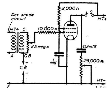
Fig. 1.—The circuit arrangement for an efficient transformer-fed tetrode output circuit suitable for about 500 mW. output.
