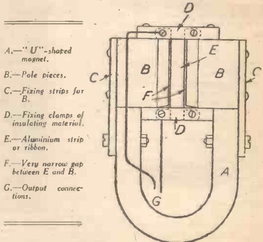
Fig. 2.—Details of a ribbon microphone.
