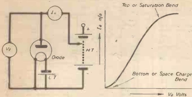
Fig. 13.—The  $I_a/V_a$  characteristic curve of a diode.
