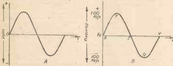
Fig. 1.—A illustrates the AF voltage plotted against time. B illustrates the corresponding variation in carrier frequency plotted against time.
