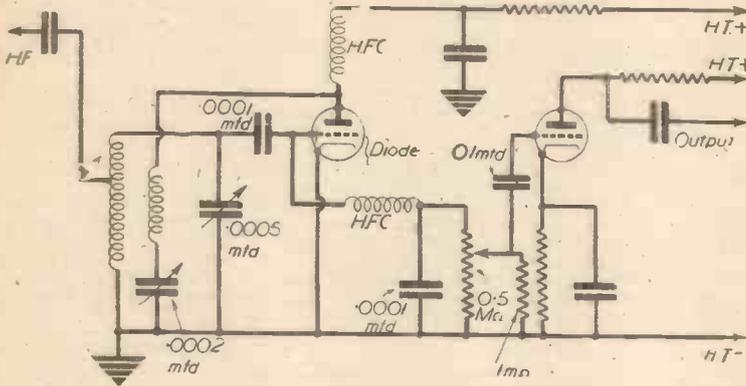
Fig. 3.—A triode used as a combined diode detector and oscillator. It is shown followed by a triode L.F. amplifier.
