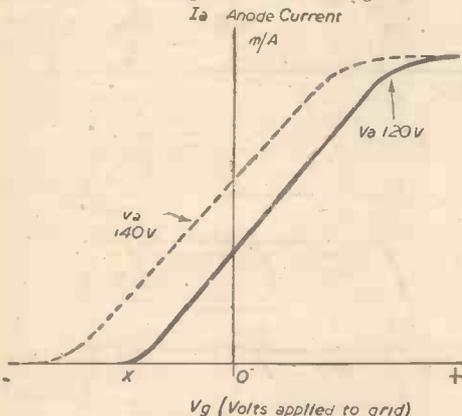
Fig. 18.—A typical Ia/Vg characteristic curve of a triode.
