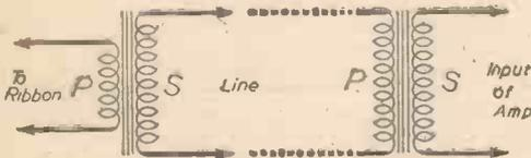
Fig. 6.—Matching of a ribbon microphone.
