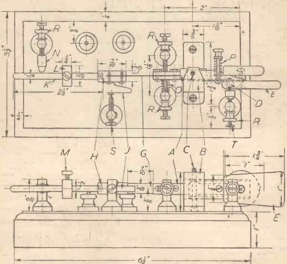
Fig. 3.—Plan and side elevation of the "bug" key described in the text.
