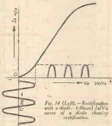
Fig. 14 (Left).—Rectification with a diode. (Above)  $I_a/V_a$  curve of a diode showing rectification.
