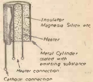
Fig. 11.—An indirectly heated cathode.
