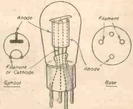
Fig. 12.—A diode valve and its component parts.
