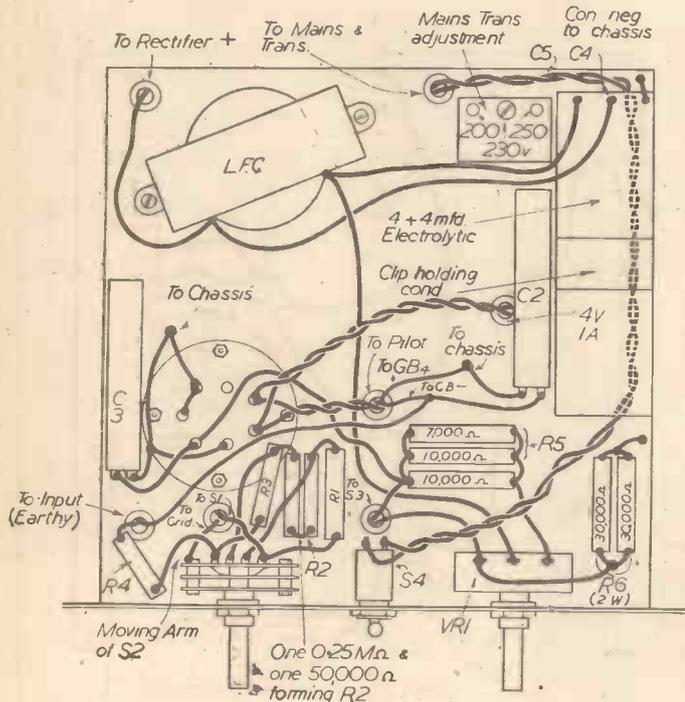
Fig. 3.—Under chassis layout and wiring.
