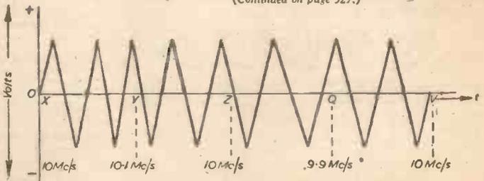
Fig. 2.—Variation of carrier frequency on modulation. This graph is another form of the graph shown in Fig. 1B, and the points X, Y, etc., correspond on the two graphs.
