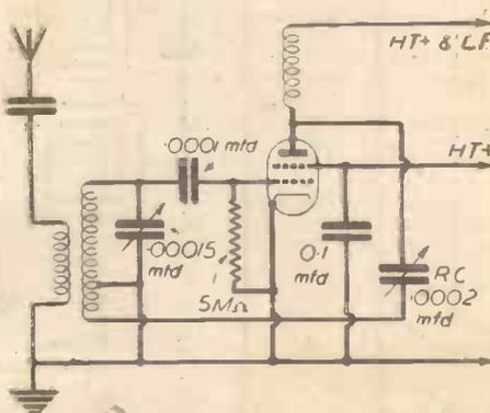
Fig. 2.—A tetrode valve used in a conventional Reinartz reaction circuit.
