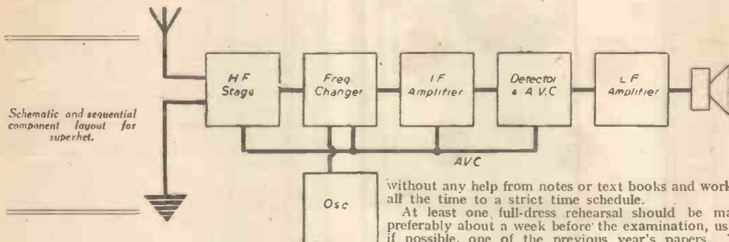
Schematic and sequential component layout for superhet.
