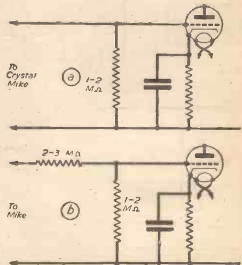
Fig. 8.—Connections for crystal microphones.
