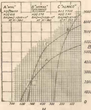
Fig. 3.—Graph showing the comparative magnetic fluxes of Nial, Hymax and Alnico.
