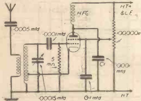
Fig. 1.—Outline circuit of a cathode-coupled regenerative detector. It should be compared with the circuit shown in Fig. 2. Values shown are applicable to a short-wave receiver.
