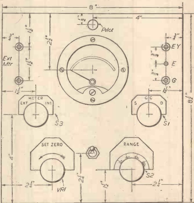
Fig. 4.—Panel layout and drilling measurements.
