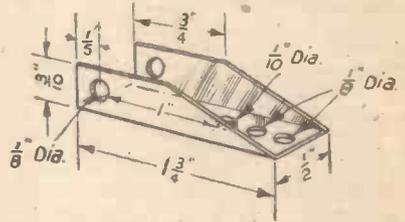
Fig. 2.—Details of metal bracket.
