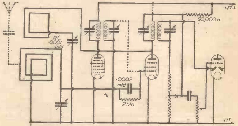
Fig. 4.—This skeleton circuit of the first three valves in a typical portable battery superhet shows how the set can be modified for use as a Det.-L.F.-output receiver in the event of failure of the frequency-changer. Broken lines indicate leads which are to be removed; available aerial-earth connections are also shown in broken lines.
