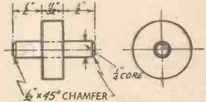
Fig. 4.—Details of Alnico bobbins.
