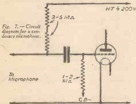
Fig. 7.—Circuit diagram for a condenser microphone.
