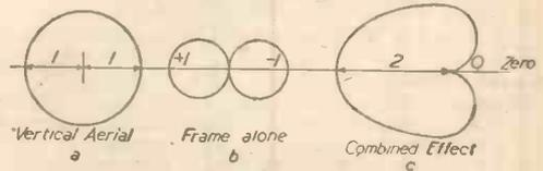
Fig. 3.—Principle of the cardioid response curve.
