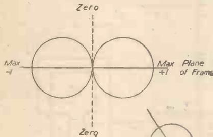
Fig. 1 (Above).—Diagram illustrating the response of a frame aerial.
