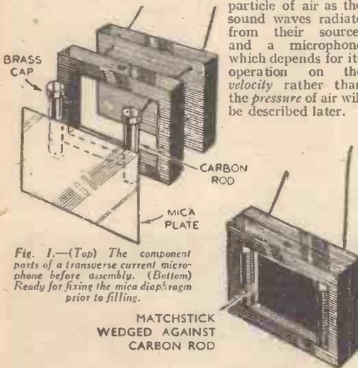
Fig. 1.—(Top) The component parts of a transverse current microphone before assembly. (Bottom) Ready for fixing the mica diaphragm prior to filling.
