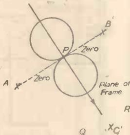
Fig. 2.—Indicating positions of frame aerial for separating three stations.
