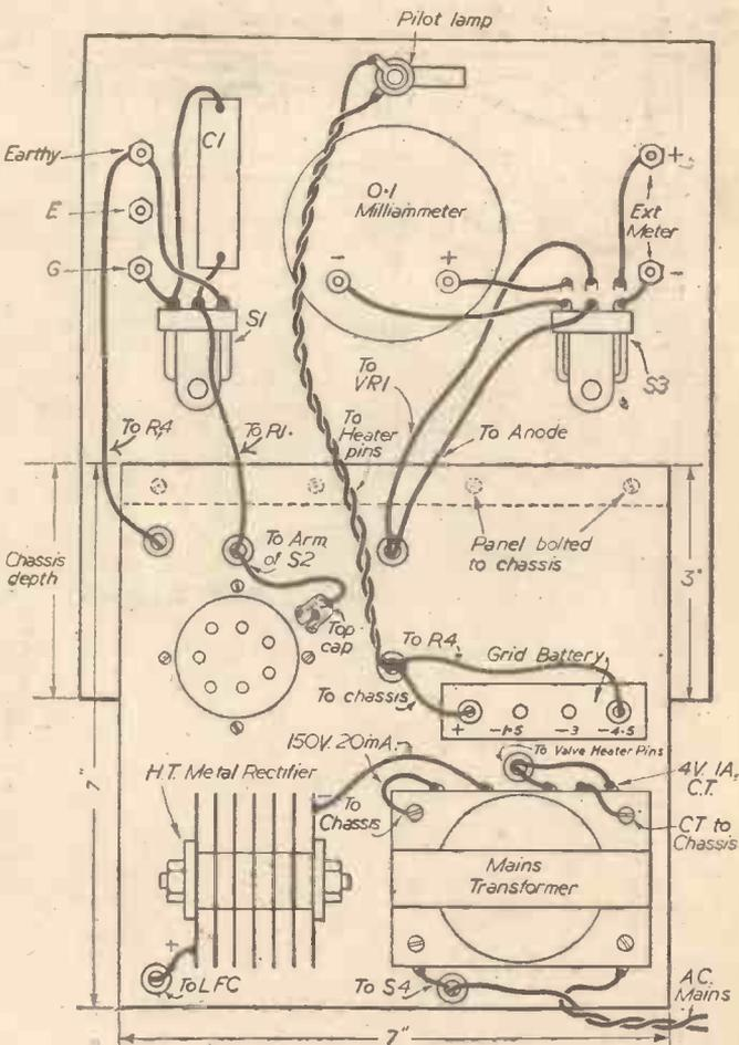
Fig. 2.—Panel and top of chassis layout and wiring diagram.
