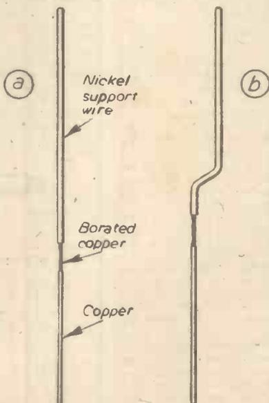
Fig. 2 (a).—Straight foot-wire. (b) Cranked foot-wire.
