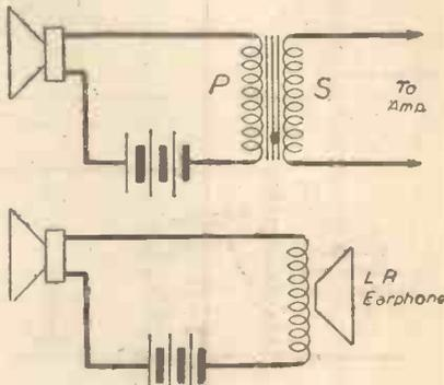
Fig. 4.—Connections for carbon microphones.
