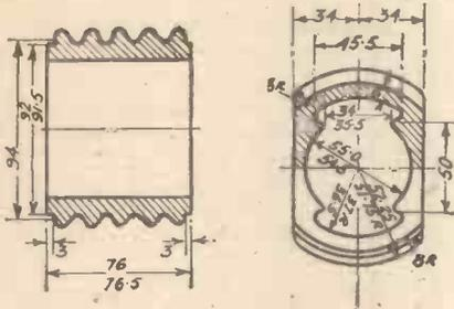
Fig. 1.—The design of a cast field magnet.
