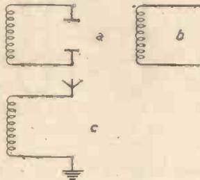
Fig. 10.—The open oscillatory circuit.
