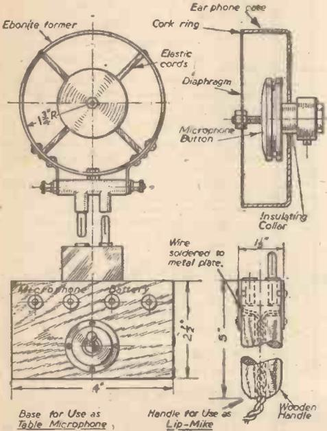
A novel microphone constructed from spare parts.
