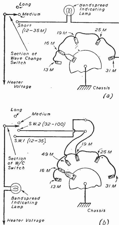
Fig. 23.—(a) and (b). Various methods of connecting the fixed contacts and bandspread indicating lamps to obtain different effects.
