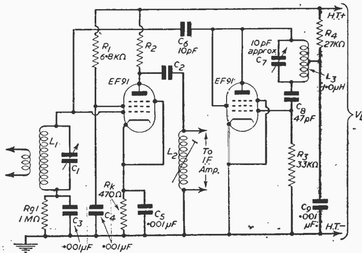
Fig. 1.—Typical television mixer circuit.
