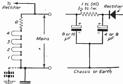
Fig. 1 (left).—Normal arrangement of heaters for A.C. or D.C. supply. Fig. 2 (right).—H.T. smoothing at its simplest.
