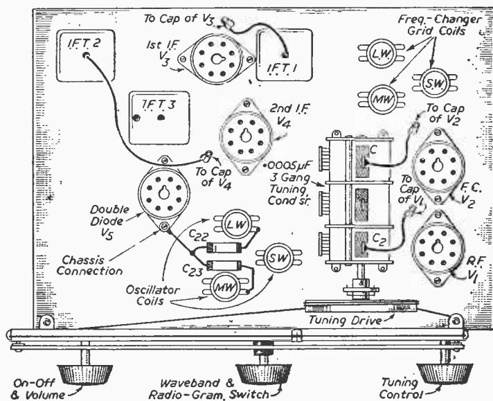
Fig. 2.—Chassis layout of the receiver section.
