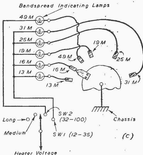
Fig. 23.—(c). Further method of connecting the contacts.
