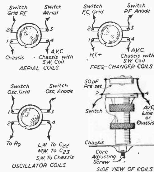
Fig. 4.—Coil connection details.
