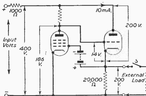
Fig. 3.—A high-gain pentode added to the circuit of Fig. 2.
