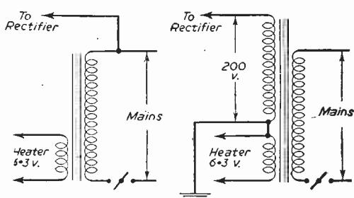
Fig. 3 (left).—Using a transformer for the heater supply. Fig. 4 (right).—Isolating the receiver from the mains by a single transformer.
