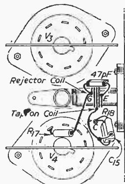
Fig. 3.—Actual position of the rejector coil on the chassis side runner.
