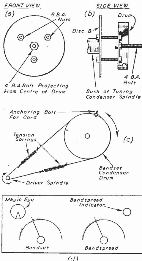
Fig. 22.—(a) and (b). How a drum for a cord drive may be fitted to the handset tuning condenser. (c) A spring is fitted to both sides of the cord drive to avoid strain (see text). (d) Suggested dial layout for the unit.
