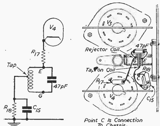
Fig. 2.—Position of the rejector coil in the cathode circuit of V4.
