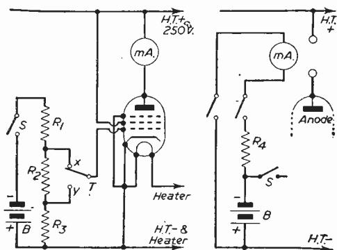
Figs. 1 and 2.—The circuit diagram and method of arranging battery check.
