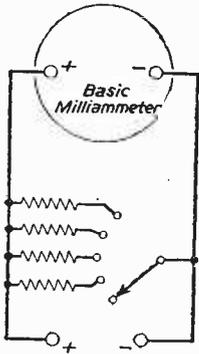
Fig. 7.—How shunts may be switched for multi-range milliammeters.
