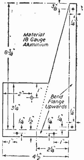
Fig. 3.—Details of the dial bracket.
