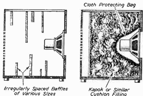
Figs. 3 and 4.—Alternative ideas for reducing cabinet resonance or "boom."
