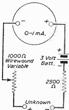
Fig. 8.—Circuit arrangement for an ohm-meter.
