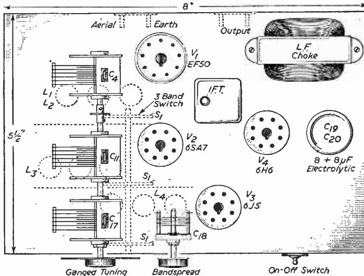
Fig. 2.—Chassis dimensions and layout.
