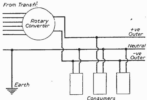
Fig. 2.—Three-wire D.C. supply.
