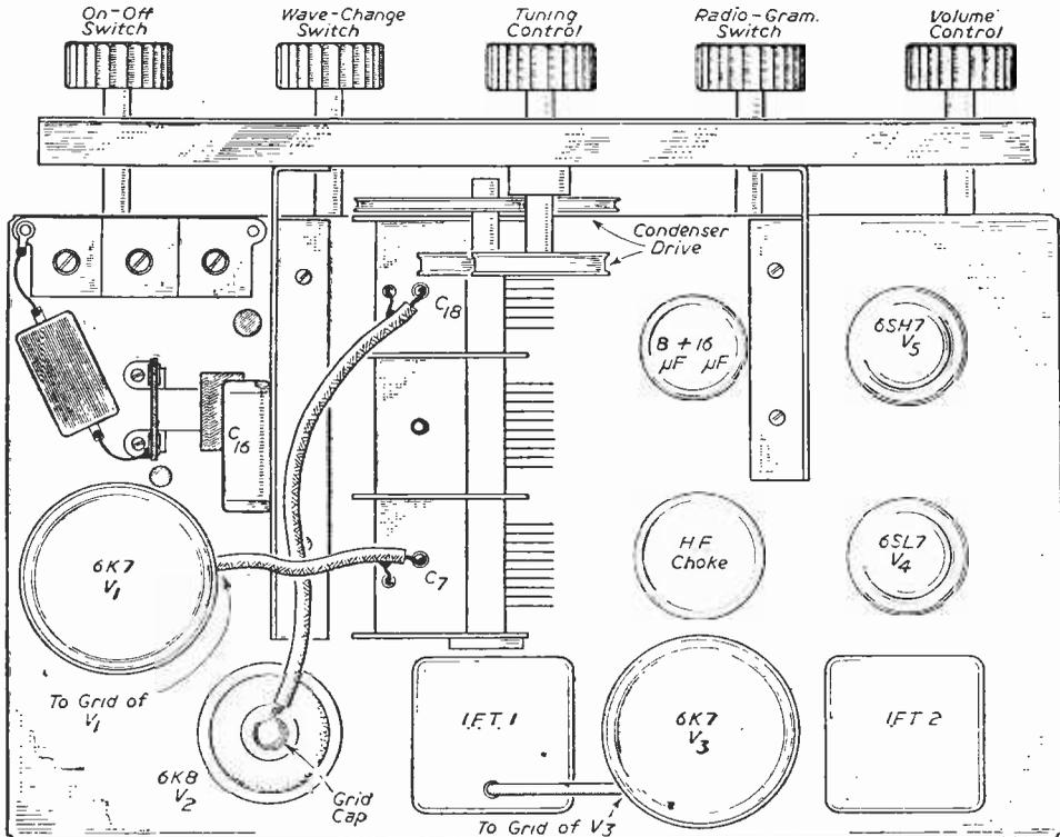
Fig. 4.—Top of chassis view of the tuner.
