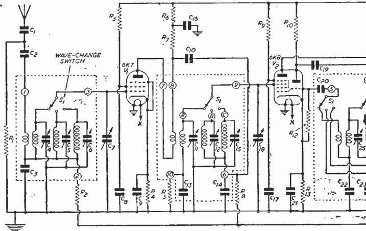
Fig. 1.—Theoretical circuit of the tuner unit. The components within
