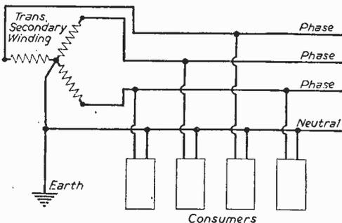
Fig. 1.—Three-phase, four-wire system for A.C.
