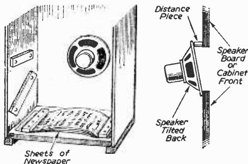
Figs. 1 and 2.—Cabinet resonance may be modified or reduced, as shown here.
