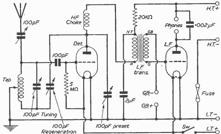
Fig. 1.—Theoretical diagram of a 2-valve Hartley Circuit.
