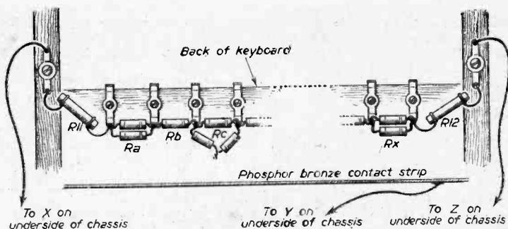
Fig. 14.—Arrangement of resistors to obtain correct tuning as explained this month.
