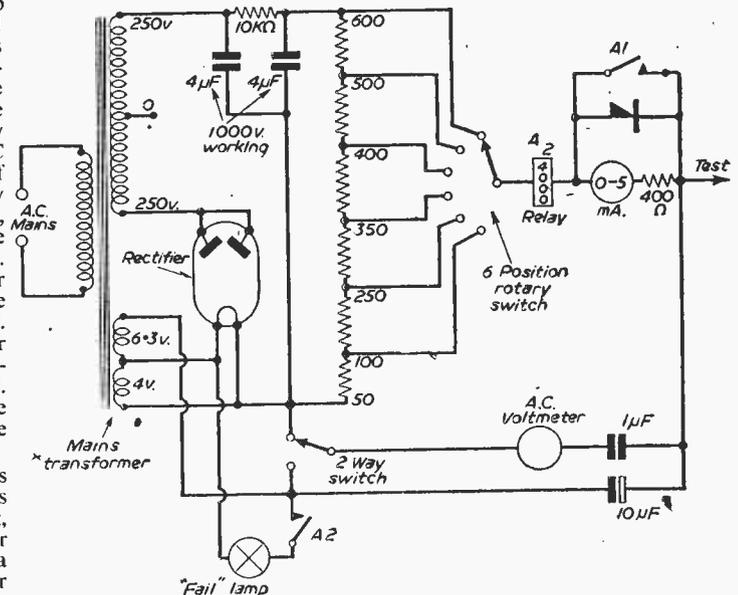
Circuit of the condenser test set.
