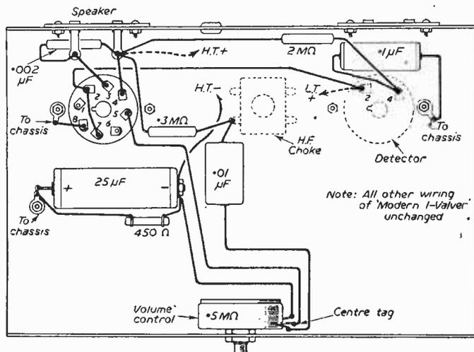
Components and wiring for the L.F. stage.
