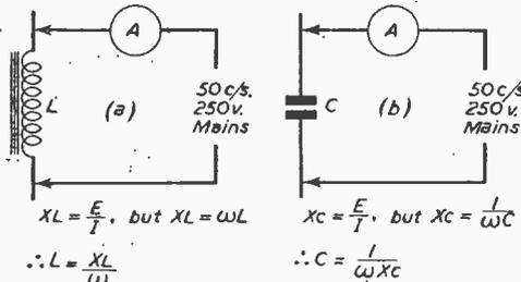
Fig. 1 (a) and (b).—Method of measuring the value of  $L$  or  $C$ .
