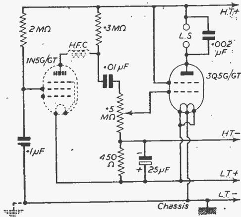
Theoretical circuit, showing additional wiring.
