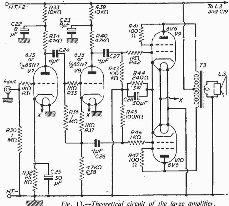
Fig. 13.—Theoretical circuit of the large amplifier.
