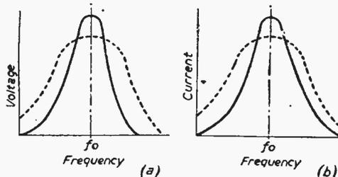
Fig. 8.—(a) Response curve of the rejector circuit, and (b) response curve of the acceptor circuit.
