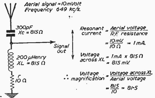
Fig. 6.—The acceptor circuit.
