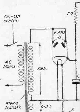
Fig. 1.—Theoretical circuit.
