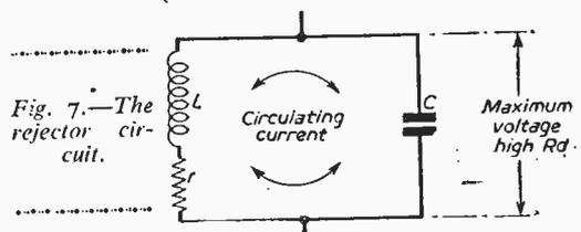
Fig. 7.—The rejector circuit.
