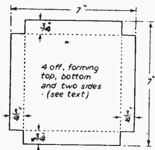
Fig. 5.—Details of the case.
