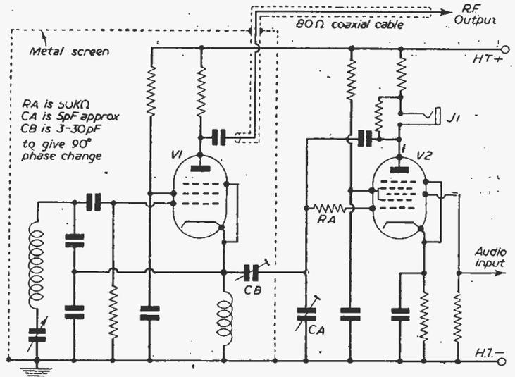
Fig. 1.—Basic N.B.F.M. V.F.O.-reactance modulator circuit.
