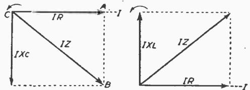
Fig. 2. (Left)—Showing how the voltage  $IX_c$  across a condenser lags the current by an angle of 90 deg.
