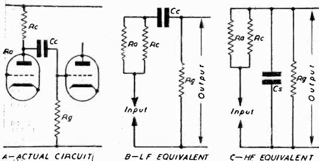
Fig. 1.—Resistance-capacitance coupling circuit and equivalents for L.F. and H.F. response. (a) Actual circuit. (b) L.F. equivalent. (c) H.F. equivalent.
