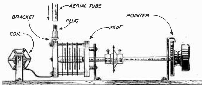
Figs. 1 and 2.—Two views of the unit to show layout and wiring.
