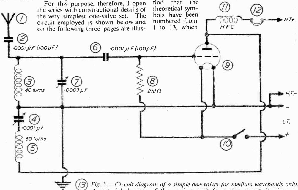
13 Fig. 1.—Circuit diagram of a simple one-valver for medium wavebands only. A pictorial diagram of the receiver built from this circuit is given on page 253. Where crossing lines are connected by a dot, they are to be joined by solder.
