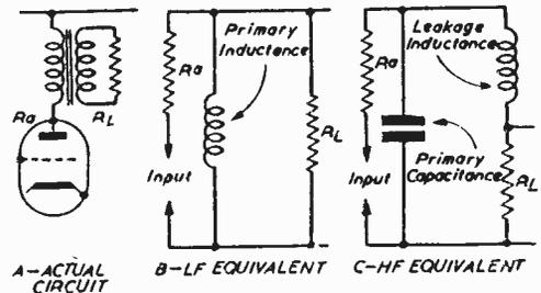
Fig. 3.—Output transformer circuit and equivalents. (a) Actual circuit. (b) L.F. equivalent. (c) H.F. equivalent.
