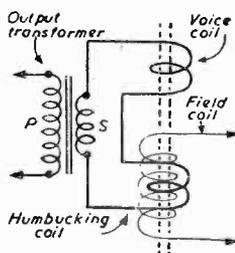
Fig. 1.—Showing the connections for a hum-bucking coil.
