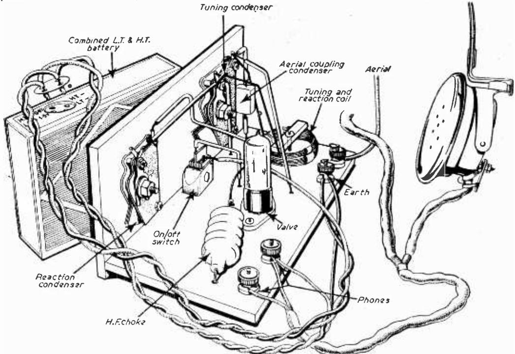
Fig. 10.—Pictorial wiring diagram of circuit shown by Fig. 1. Some of the wiring is underneath the baseboard, which is fixed to the panel to clear the valve holder sockets.
