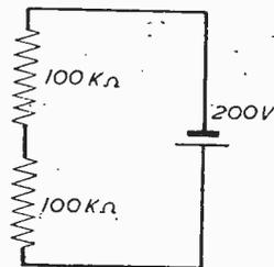
Fig. 1.—Diagram to explain voltage drop across two resistors in series.
