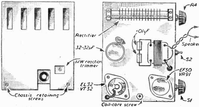
Fig. 2.—Details of the chassis.
