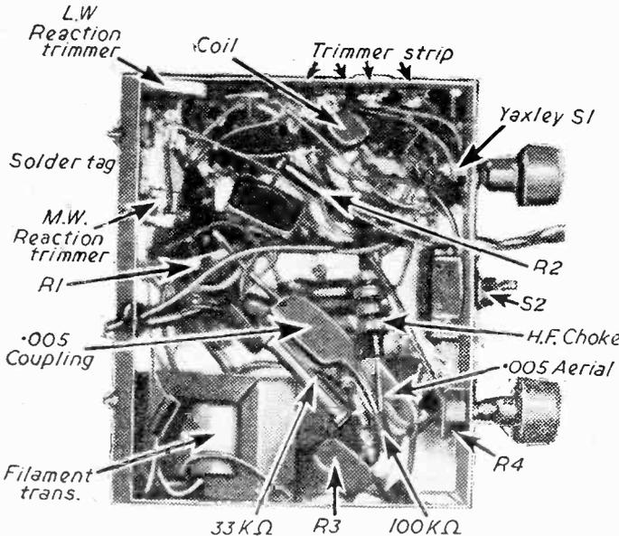
View of the underside with main components identified.
