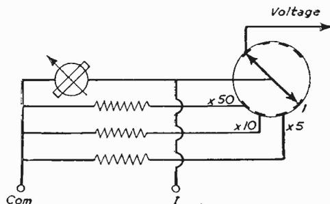
Fig. 3.—Circuit of a current meter to give different ranges by means of a selector switch.
