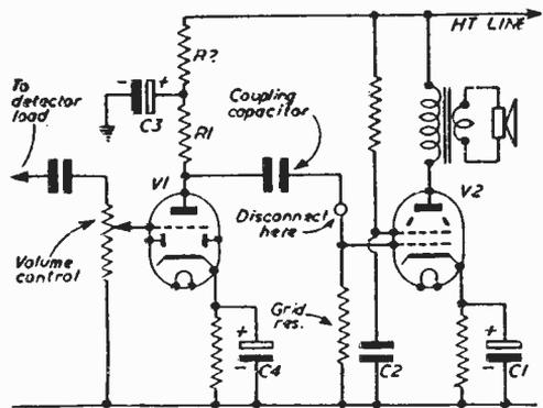
Fig. 2.—The output stage and first A.F. amplifier of a typical receiver.
