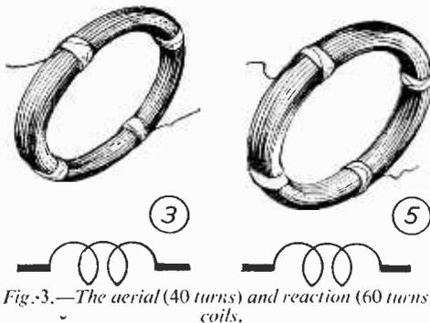
Fig. 3.—The aerial (40 turns) and reaction (60 turns) coils.
