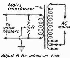
Fig. 3.—A method of balancing the valve heater circuit.
