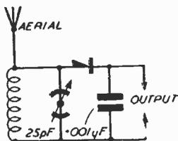
Fig. 3.—Theoretical circuit of the meter.
