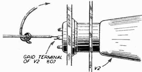
Fig. 5.—Details of neutralising condenser.
