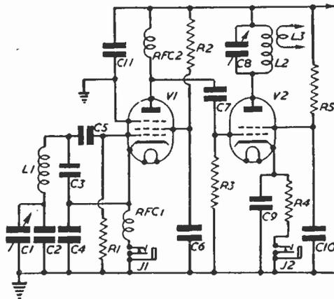
Fig. 1.—Theoretical circuit of the transmitter.
