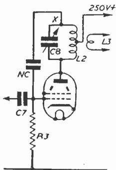
Fig. 4.—P.A. circuit using neutralisation.
