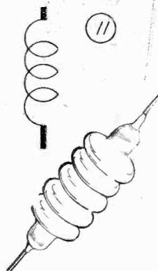
Fig. 9.—The high-frequency choke.
