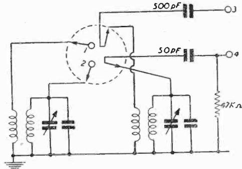
Fig. 2.—Wiring to the wavechange switch.
