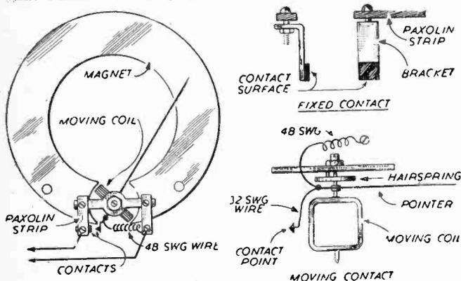
Fig. 3.—Details of the microamp relay.
