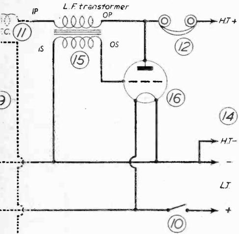
which is modified from the one valve circuit given in Fig. 14. The new wires and additional components are shown in dotted lines. The new wires and additional components are a low-frequency transformer, a valve and a valve filament transformer (15 and 16).
