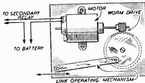
Fig. 4.—A typical controlling mechanism.
