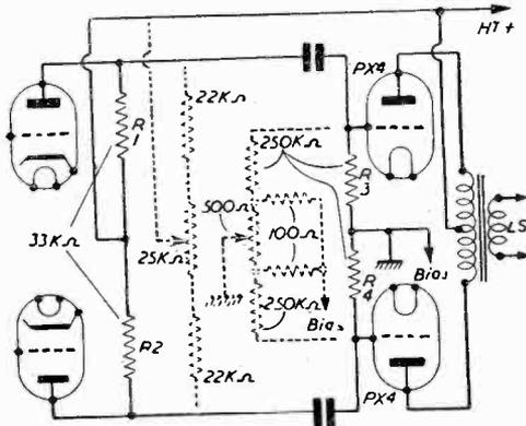
Fig. 1 (a).—Networks to be substituted for R1-R4 are shown in broken lines.
