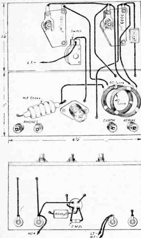
Fig. 12.—Wiring diagram for the simple one-valve circuit diagram of which was given last month. A circuit diagram showing how to convert it into a two-valve is shown in Fig. 13.
