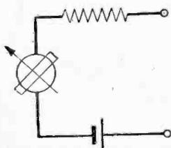
Fig. 4.—Basis of the ohm-meter.
