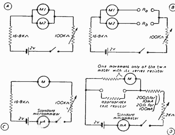
Fig. 2.—Circuits used in checking meters and test resistors.
