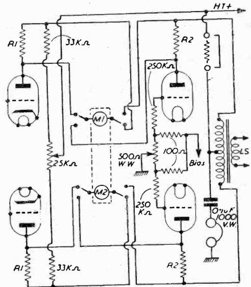
Fig. 3.—Test voltages are developed across R1-R4, whose values are calculated as described in the text.
