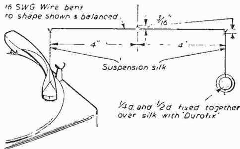
*Adjusting the weight of the pick-up.*
