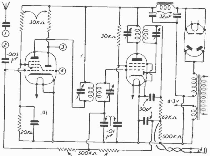
Fig. 1.—Theoretical circuit of the feeder unit.
