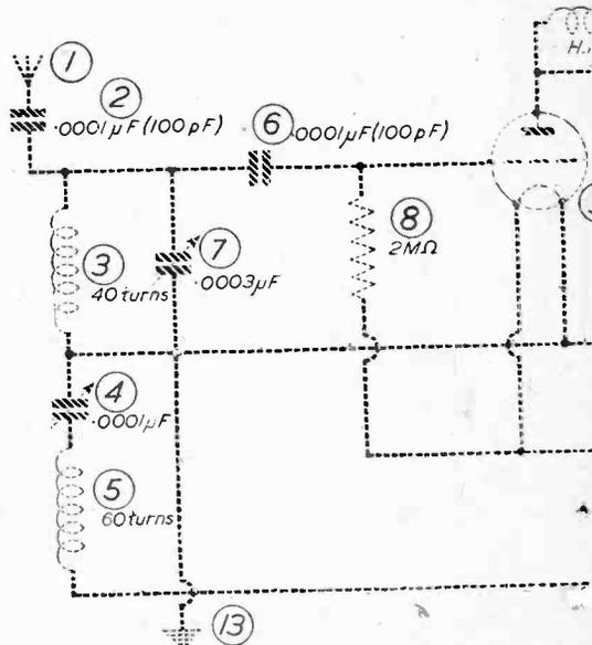
Fig. 13.—Theoretical circuit of a two-valve receiver, as last month. The one valve circuit is shown by means of dashed lines. The only additional parts are shown by solid lines. The only additional parts are shown by solid lines. The only additional parts are shown by solid lines.
