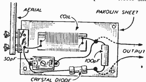
Fig. 2.—Wiring diagram of the receiver.
