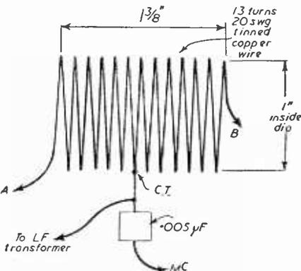
Fig. 4.—Details of the tuning coil.
