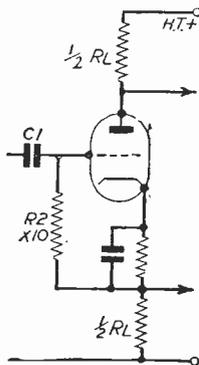
Fig. 2.—The "concertina" phase splitter circuit.
