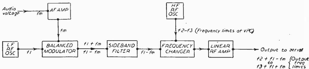
Fig. 2.—This is another S.S.B. block schematic.
