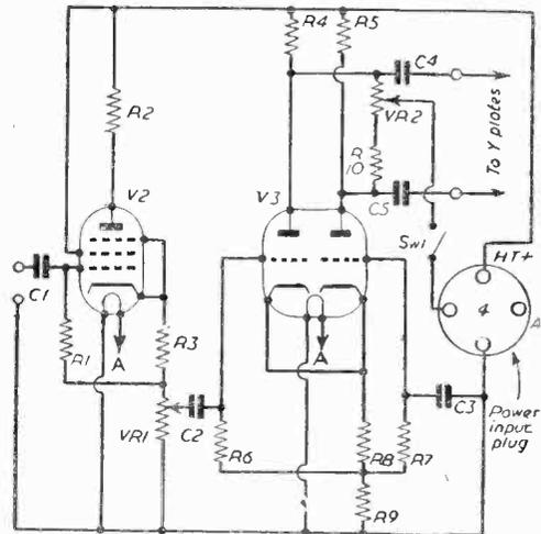
Fig. 4.—The "Y" Amplifier showing sync control.
