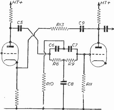
Fig. 7.—Treble cut arrangement.
