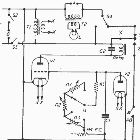
Fig. 4.—Final circuit of the Timer.
