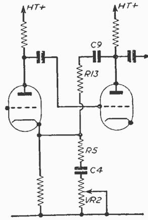
Fig. 6.—Treble boost circuit.
