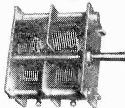
GANG CONDENSERS. Available as 1, 2 or 3 gang, 490 p.F nominal capacity with Cadmium plated steel frame, aluminium vanes; matched and standardised to close limits. Low loss non-hygroscopic insulation. Prices from 9/-.
