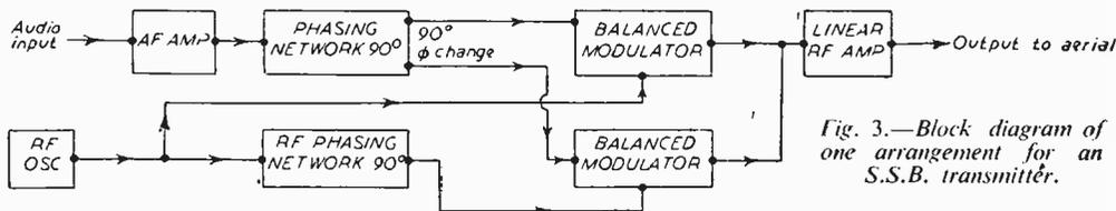
Fig. 3.—Block diagram of one arrangement for an S.S.B. transmitter.
