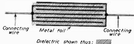
Fig. 42.—A diagrammatic representation of a fixed condenser.
