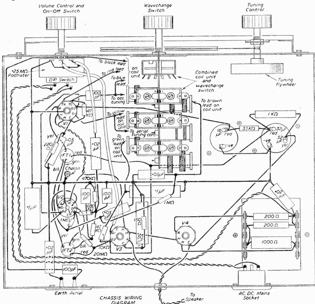
Wiring diagram of the A.C./D.C. Coronet Four.
