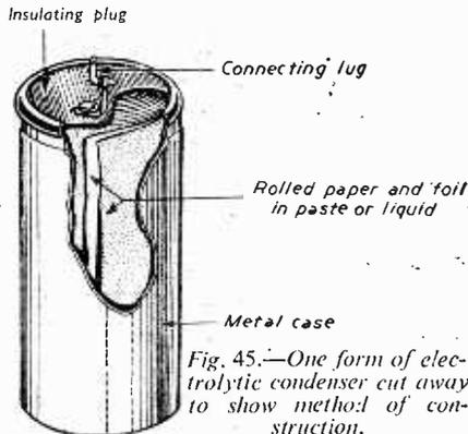
Fig. 45.—One form of electrolytic condenser cut away to show method of construction.
