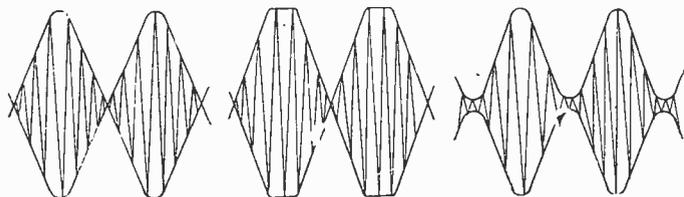
Figs. 4, 5 and 6.—Two-tone waveforms, in which the two sine-wave frequencies are separated by 1.5 Kc's.
