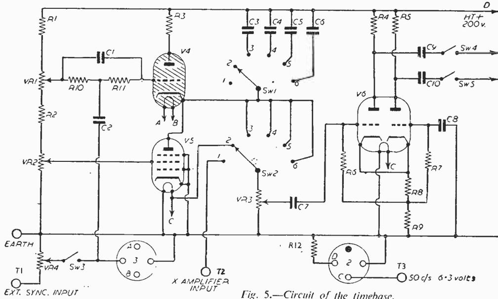
Fig. 5.—Circuit of the timebase.
