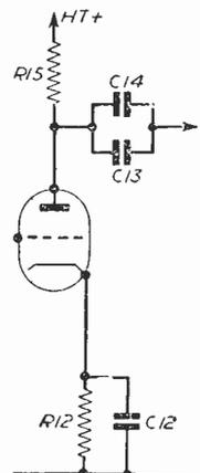
Fig. 8.—Bass cut circuit.
