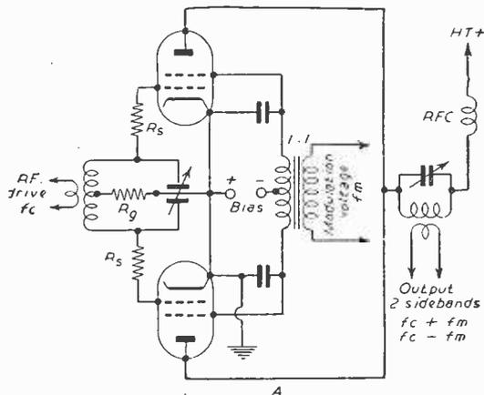
Fig. 1A.—One circuit for a balanced modulator.
