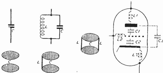
Figs. 1 and 2.—A diagrammatic explanation of inductance and capacity and "strays" in a valve.
