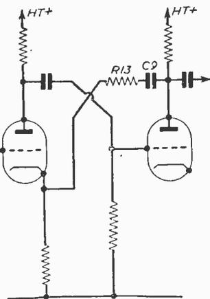
Fig. 4.—Circuit analysis at middle frequencies.
