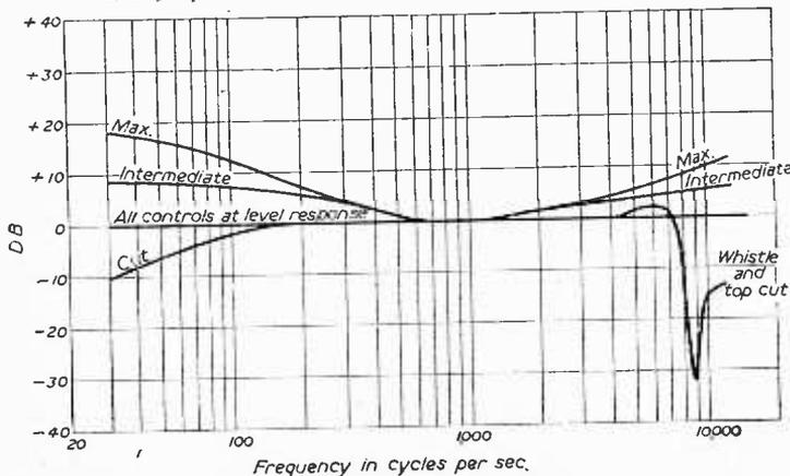
Fig. 1.—Response curves at various settings of the controls.
