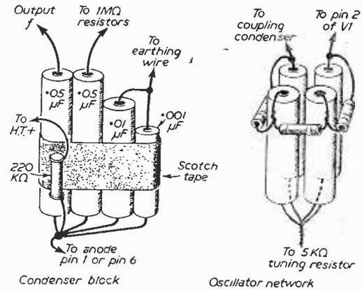
Fig. 21. — Details of the condenser blocks and oscillator units.
