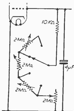
Fig. 3.—Details of the resistor adjustment.
