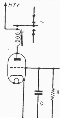
Fig. 2.—Relay operating circuit.
