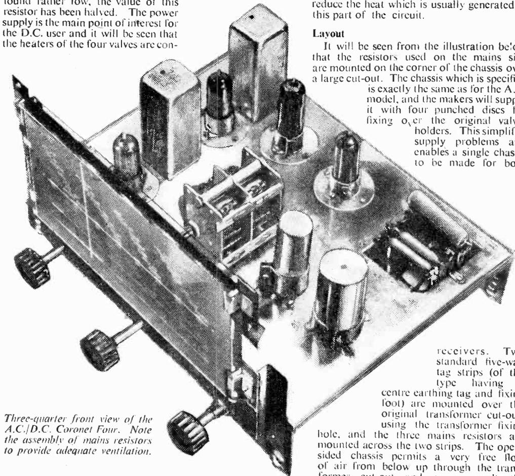
*Three-quarter front view of the A.C./D.C. Coronet Four. Note the assembly of mains resistors to provide adequate ventilation.*
