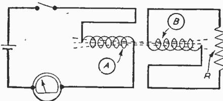
Fig. 41.—Circuit illustrating mutual induction.
