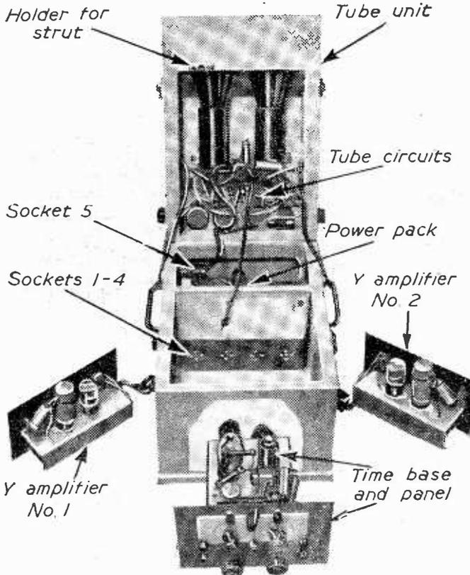
The Assembly "opened out" and the parts identified.
