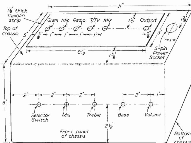
Fig. 9.—Details of the chassis for the tone control pre-amplifier.
