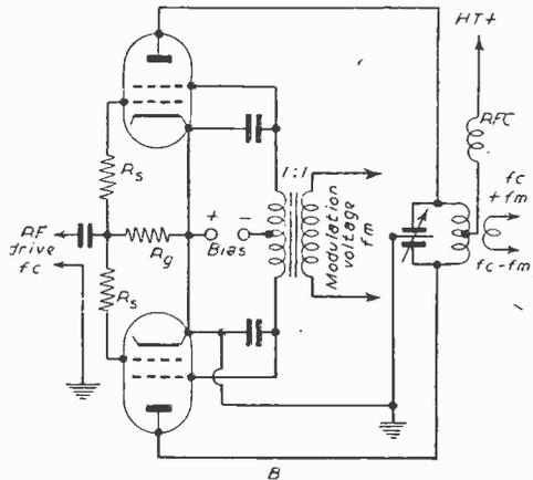
Fig. 1B.—Another circuit for balanced modulation.
