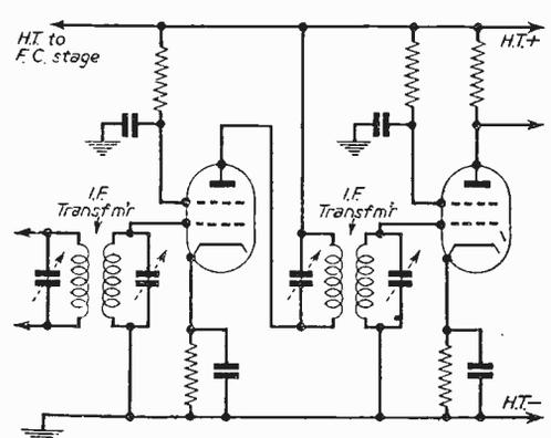
Fig. 2.—Circuit modified for superhet.
