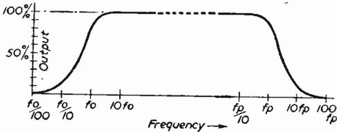
Fig. 17.—Typical response curve.
