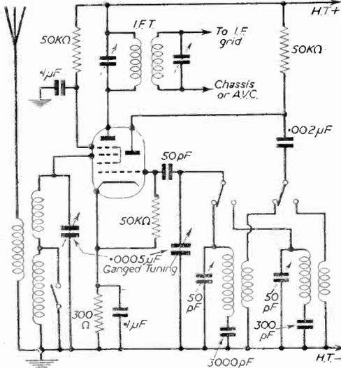
Fig. 3.—A 6K8 frequency changer stage.
