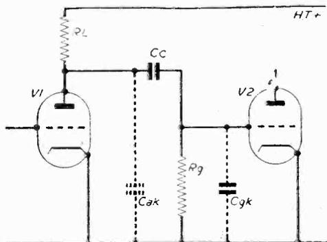
Fig. 15.—An amplifier coupled to a following valve.
