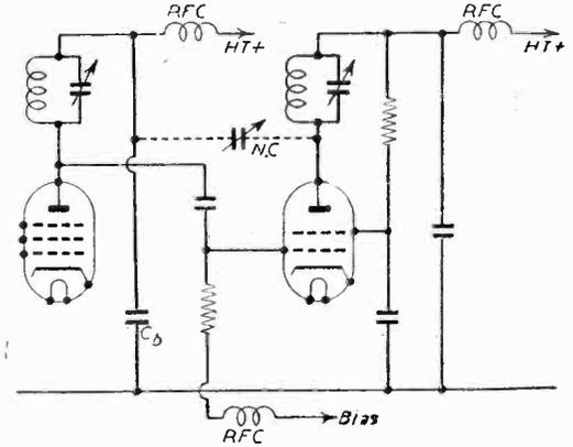
Fig. 4.—A P.A. with an untuned grid circuit driven by capacity coupling from the tank of the driver valve can have a neutralising capacitor added as shown by the dotted lines. Strictly the anode earth capacity of the driver valve should be included in calculating the "bridge ratio."
