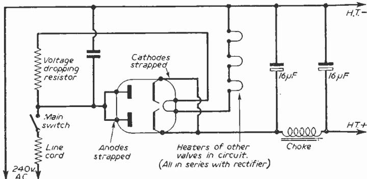
Fig. 2.—Typical A.C./D.C. mains unit.
