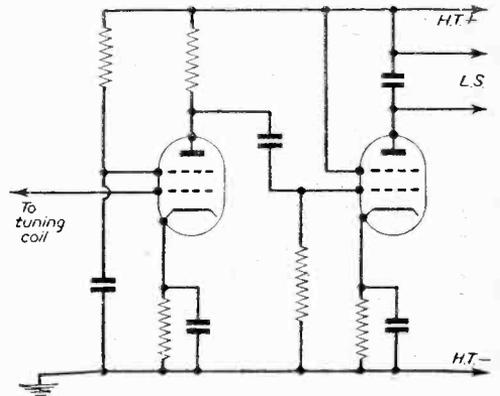
Fig. 4.—T.R.F. detector and output stages.
