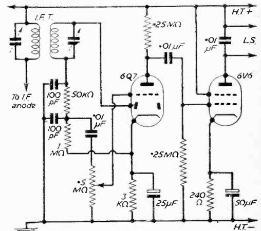
Fig. 5.—A D.D.T. and output stage for a superhet.
