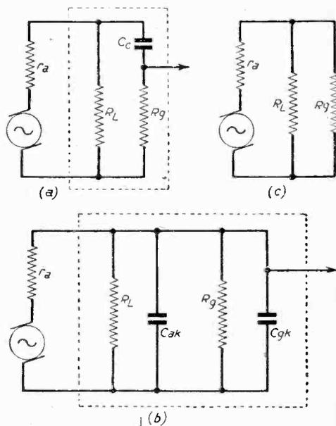
Fig. 16.—Equivalent circuits at different frequencies.
