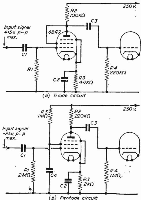
Fig. 14.—Complete single-stage circuit.
