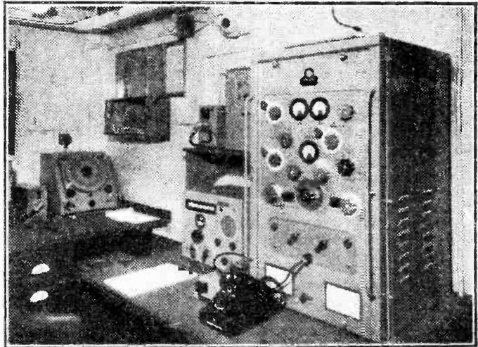
*The bench-mounted version of the new "Oceanspan" radiotelephony and telegraphy transmitter on board the new P. & O. liner Arcadia.*
