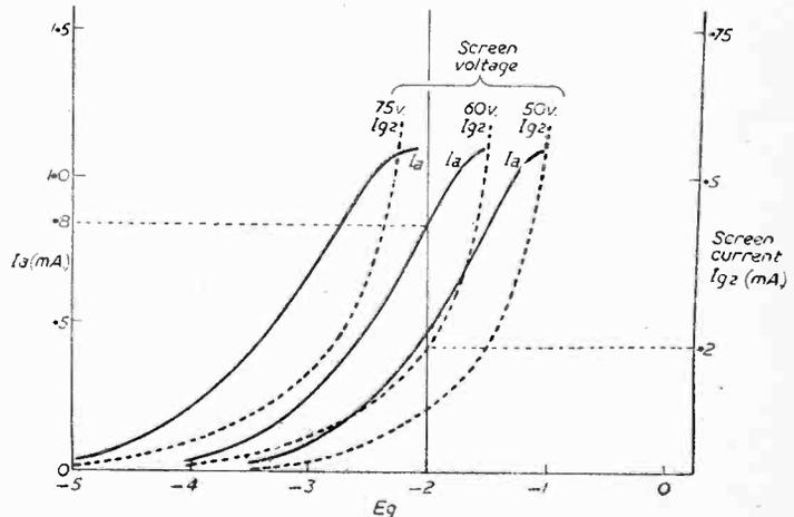
Fig. 13.—Dynamic characteristic curve of a 6BR7 pentode-connected valve. RL=220k and H.T. 250 v.
