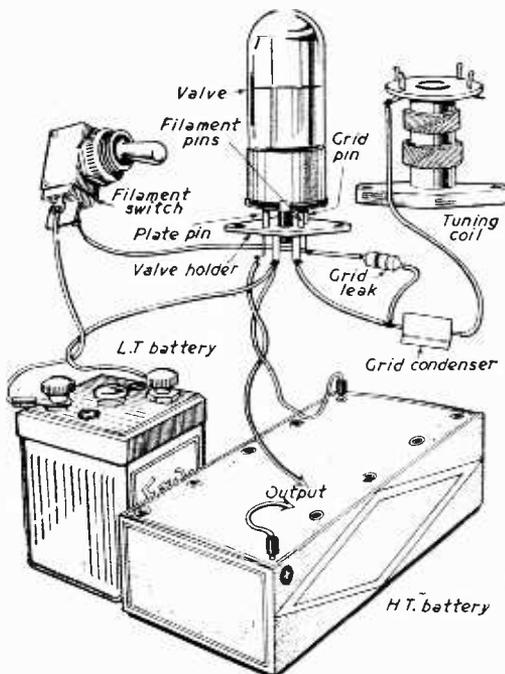
Fig. 65.—Battery connections.
