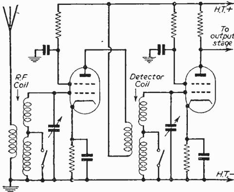
Fig. 1.—Typical T.R.F. R.F. and detector stages.
