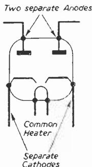
Fig. 1.—Theoretical symbol for a double-diode.
