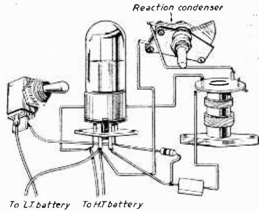
Fig. 66. — The reaction circuit.
