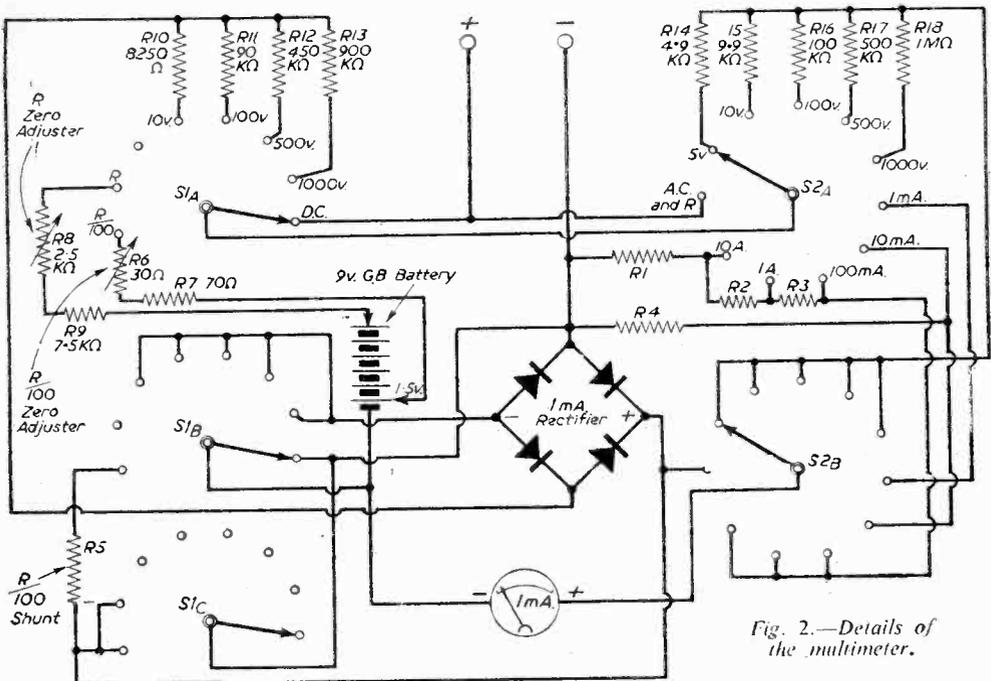
Fig. 2.—Details of the multimeter.
