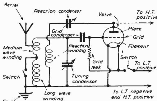
Fig. 64. — Circuit of a detector stage.
