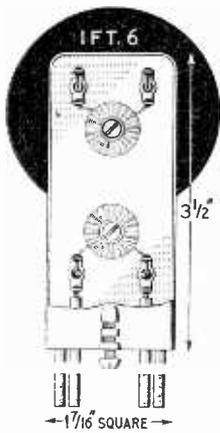
**IFT.6/465 kc/s or 1.6 Mc/s.**—A superior I.F. transformer for use in high quality receivers and tuners. Permeability tuned, Litz wound coils, using Neosid iron dust cores, and high quality silver mica condensers housed in an extruded aluminium can. Termination is made by four coloured leads. Coupling is optimum at 465 kc/s and slightly sub-optimum for increased selectivity at 1.6 Mc/s.
