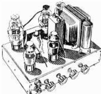
LOOPS with 15 db in the main loop from output transformer to voltage amplifier. Frequency response  $\pm 3$  db. 50-20,000 c.p.s. HUM and DISTORTION LESS THAN 0.5
