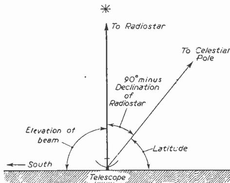
Fig. 1.—Setting up a radio-telescope: The declination of the area of the sky investigated depends on the elevation of the beam and on the latitude of the place of observation.
