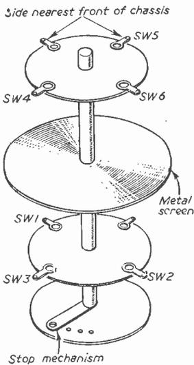
Fig. 6.—How the switch assembly is made up.
