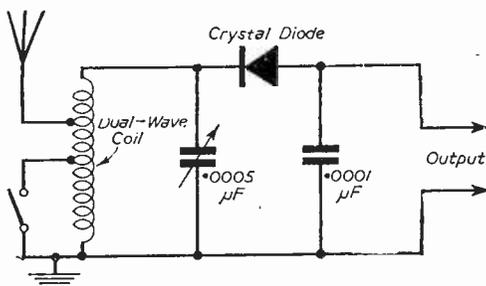
Fig. 1.—A simple crystal diode tuner.
