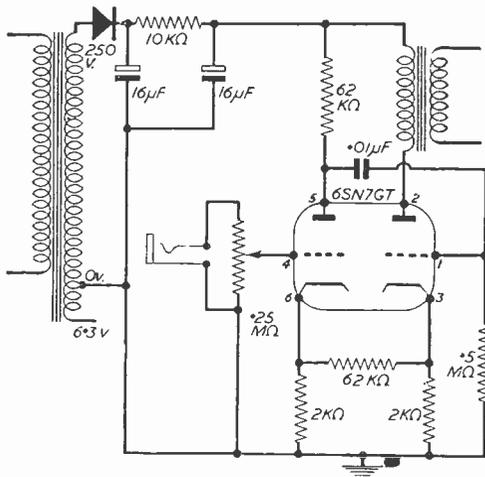
Fig. 1.—Basic theoretical circuit.
