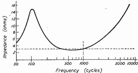
Fig. 33.—Impedance curve of a typical moving-coil speaker, nominally 3 ohms.
