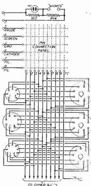
Fig. 2.—Wiring to the valholders.
