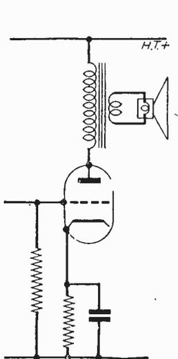
Fig. 35.—Basic circuit of triode output stage.
