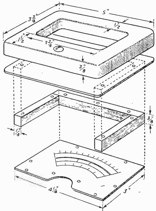
Fig. 5.—Details of the dial mounting.
