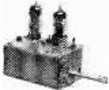
Instant and positive selection of any one of the 5 B.B.C. television channels, by a single control knob. Uses EF.80 R.F. pentode and ECC81 or 12AT7 Double Diode Triode as frequency changer. Tuning by switching incremental inductances. Size : 4 1/2 x 2 1/2 x 2 1/2 ins. Spindle 2 1/2 ins. long. 1in. diameter. I.F. Output 9.5-13 Mc/s. noise figure better than 10.5dB. I.F. rejection better than 45dB. on all channels. Power gain 24dB.
