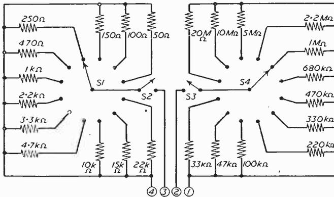
Fig. 3.—Low and high values are selected in this arrangement.
