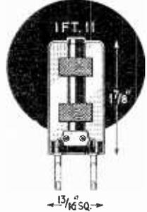
**IFT.11/465 kc/s or 1.6 Mc/s.**—Miniature I.F. transformers for 465 kc/s or 1.6 Mc/s, giving excellent performance at low cost. The coils are Litz wound and permeability tuned with high-grade Neosid iron dust cores. Coupling is critically adjusted to give maximum gain with good selectivity. Ideal for use with Miniature B9A or B7G based valves.
