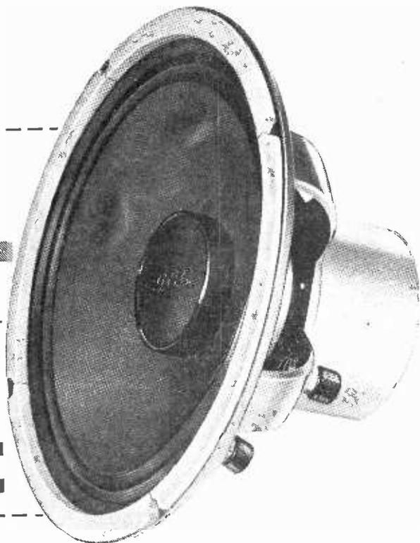
The G.E.C. metal cone loudspeaker gives lifelike reproduction of any type of sound over a range of 9 octaves. This includes the entire musical fundamental range together with overtones which give tonal quality and character to the performance of each musical instrument. The sound engineer will appreciate the simplification and improvement in performance which has been achieved by combining the following attributes in a single unit.
