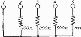
Fig. 5.—The arrangement used in the P.O. box.
