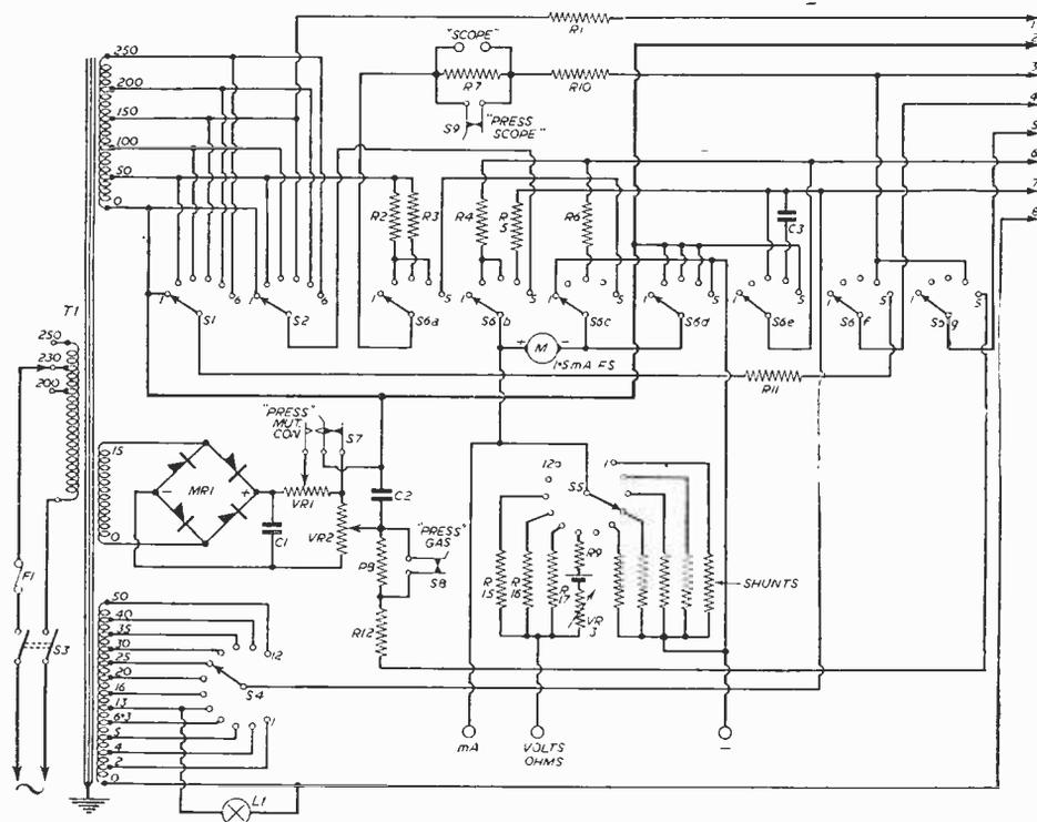
Fig. 1.—Theoretical circuit of the main part of the tester.
