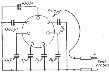
Fig. 1.—The simplest form of capacitor substitution panel.
