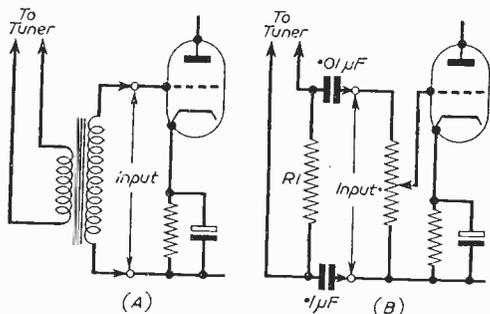
Fig. 4.—Two types of input circuit.
