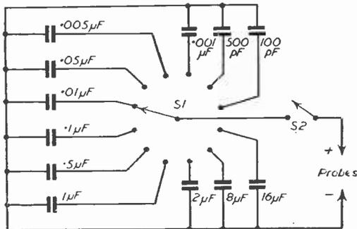
Fig. 2.—A switched version of a capacitor selector.
