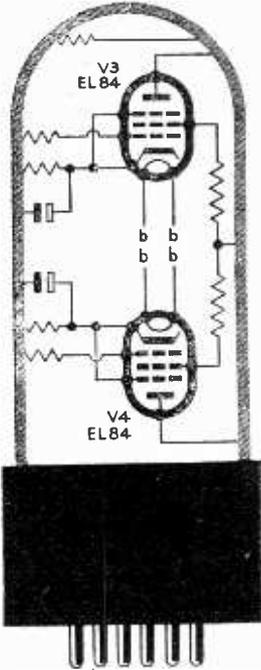
Mullard have designed a new high quality 10 watt audio frequency amplifier circuit around five Mullard valves. It follows conventional lines and comprises a high gain input stage (Mullard EF86), a cathode coupled phase-splitter (Mullard ECC83) and a push-pull output stage employing two Mullard EL84 pentodes.
