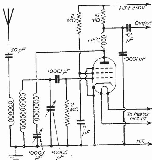
Fig. 2.—A simple one-valve tuner.
