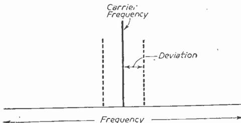
Fig. 9. — Diagram illustrating the deviation obtained in F.M.
