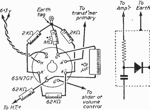
Fig. 2.—Wiring layout and suitable probe unit.
