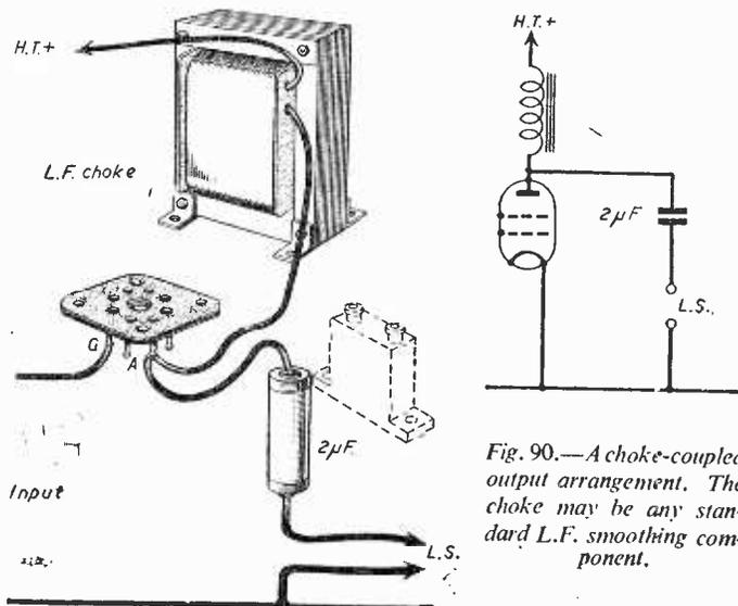
Fig. 90.—A choke-coupled output arrangement. The choke may be any standard L.F. smoothing component.
