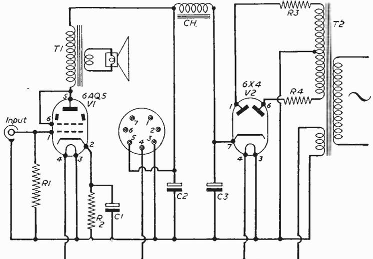
Fig. 36.—Complete circuit for a triode power amplifier—A.C. version.
