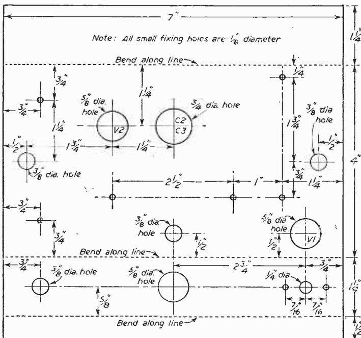
Fig. 37.—Chassis drilling diagram for A.C. amplifier (Fig. 36). Note that the  $\frac{3}{8}$ " holes are for gronimets.
