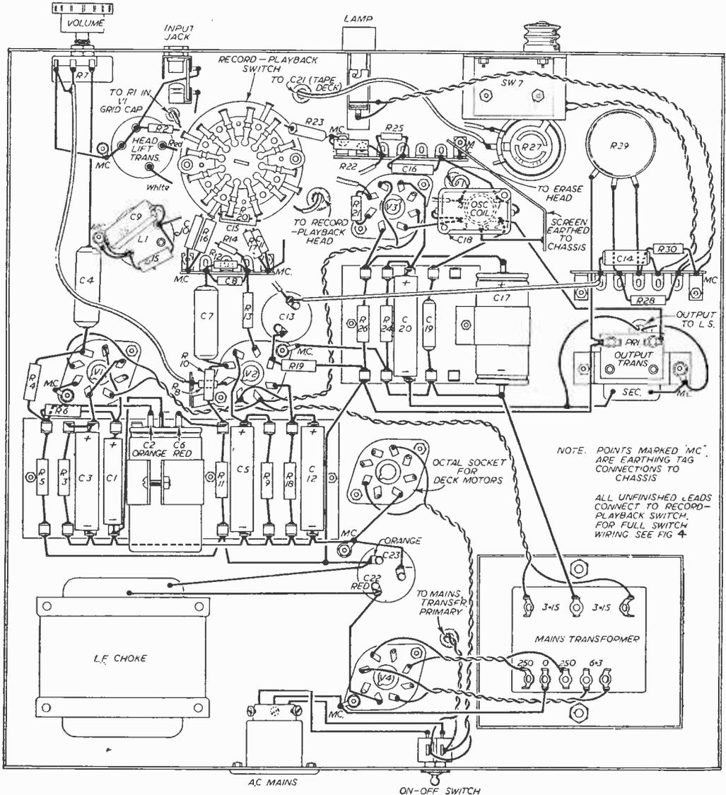
Fig. 5.—Wiring diagram of the amplifier. Note that R24 should be 220 $\Omega$  and not 220K as shown in the list of parts.
