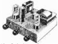
which is suitable for either 3-ohm or 15-ohm Speakers. Negative feedback is applied from the secondary of the output Transformer over the whole Amplifier to the input stage giving an excellent frequency response. Due to the high gain and wide range tone controls any type of pick-up may be used. Overall size 9 x 7 x 5 1/2in. Price of Amplifier complete, tested and ready for use, £5/5/-, plus 3/6 pkg. and carr.
