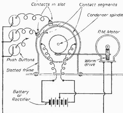
Fig. 1.—A motor-driven selector.
