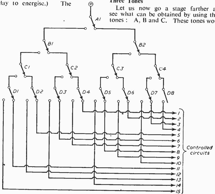
offer us seven combinations: A, B, C, A plus B, A plus C, B plus C, and A plus B plus C. This time it would not be worth while employing the carrier in combination with the tones as it would give only one extra combination (carrier by itself) and would necessitate an additional contact unit on each relay. There is nothing, however, to prevent the carrier from being used to operate the main driving motors, etc., in the manner mentioned previously.
