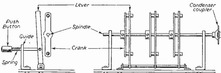
Fig. 2.—System operated by levers.
