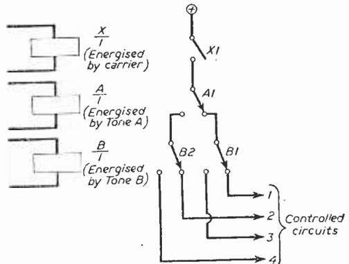
Fig. 26.—Illustrating how a carrier and two tones may be used to control four circuits.
