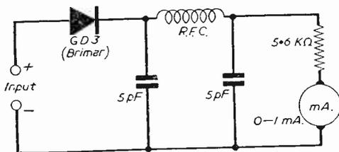
Fig. 29.—A circuit of a typical crystal voltmeter or crystal type R.F. probe.
