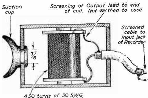
Fig. 3.—The completed attachment.
