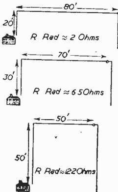
assumed ground resistance of 10 ohms, and with centre-loading coils of various Q values. In practice these figures show an improvement over the values obtainable with base-loaded vertical aeri- als that is worthwhile, especially for the very short aeri- als. It should by now be crystal
