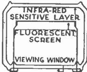
Famous wartime "cats eye" for seeing in the dark. This is an infra-red cell with a screen which lights up (like a cathode ray tube) when the electrons strike it. It follows that as light is rich in infra-red these cells will work as photo cell for burglar alarms, counting circuits. Price 5/- each. Data will be supplied with cells if requested.
