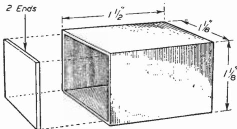
Fig. 1.—The base, made from aluminium tube.
