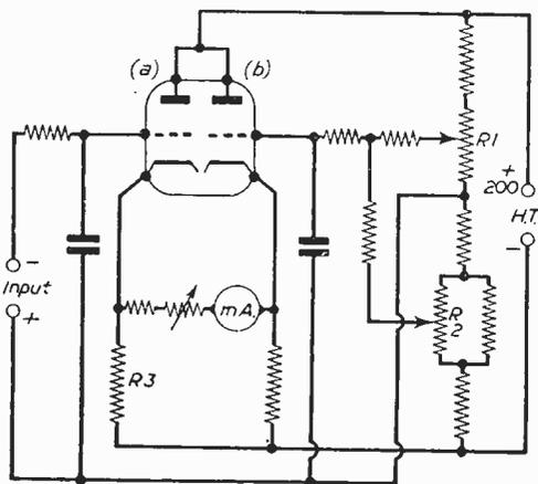
Fig. 27.—A typical valve voltmeter circuit.
