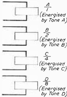
Fig. 29.—Showing how the combinations offered by four tones are capable of operating 15 different circuits.
