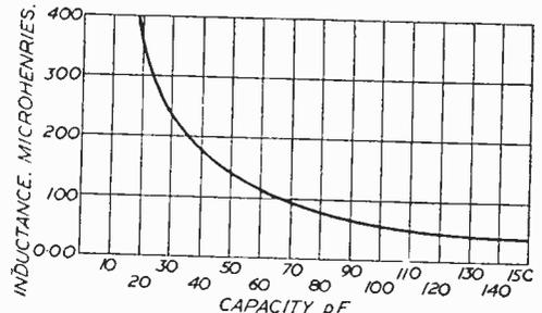
Fig. 8.—Inductance to resonate a given capacity to the middle of topband (1,900 Kc/s).
