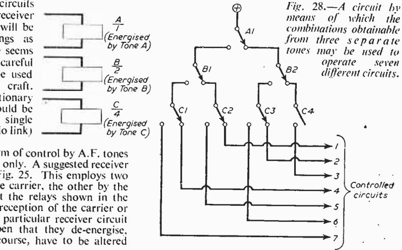
Fig. 28.—A circuit by means of which the combinations obtainable from three separate tones may be used to operate seven different circuits.
