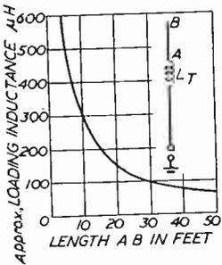
Fig. 3 (inset).—Centre-loaded aerial. Length AB and  $L_T$  should resonate to operating frequency. Fig. 4.—Centre-loading inductance values.
