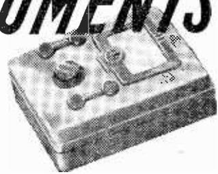
FROM this reasoning it will be realised that by disconnecting the test leads and applying them across an unknown capacitance the meter will deflect to something less than full scale. The actual deflection will, of course, depend on the C to Cx ratio, which, by employing the following formula, can be used to determine the value of the unknown capacitor.
