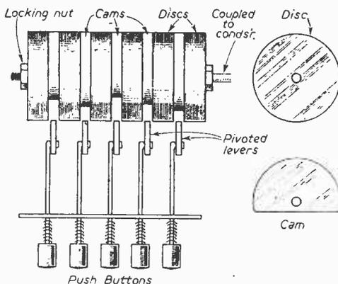
Fig. 3.—A disc and cam actuator.
