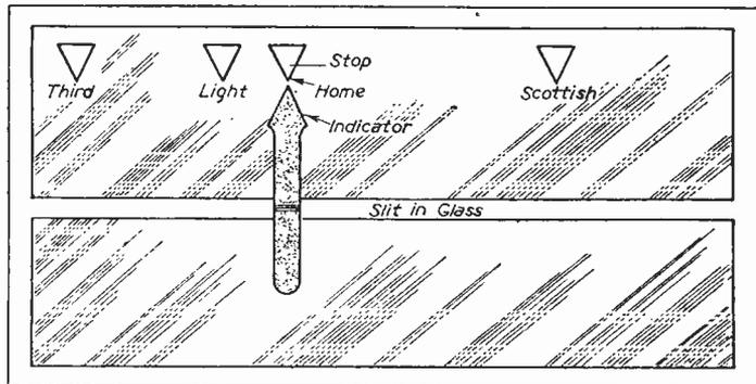
Fig. 1.—The finished modification. Here the indicator is pointing to the Home Service.
