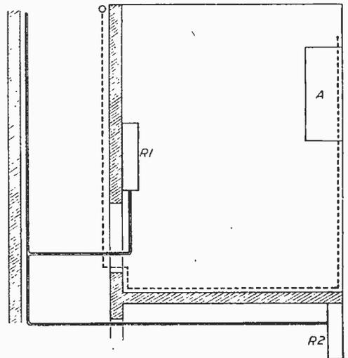
Fig. 3.—The layout of cables, heaters and amplifier and the run of the aerial.
