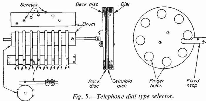
Fig. 5.—Telephone dial type selector.
