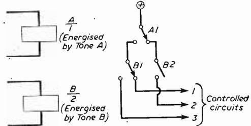
Fig. 27.—Two tones (without making use of the carrier) are capable of controlling three circuits, as shown here.
