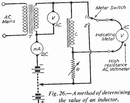
Fig. 26.—A method of determining the value of an inductor.
