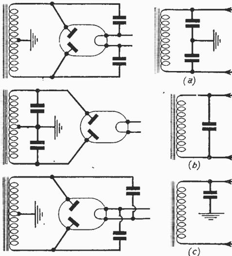
Figs. 1 & 2.—By-pass connections for the transformer secondary. The connections tried on the primary.
