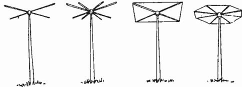
Fig. 6.—Various forms of top-loading skeleton capacities.
