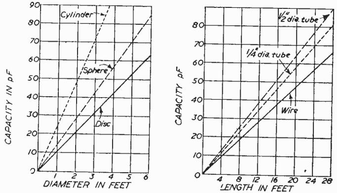
Fig. 7 (a) (left).—Capacities of spheres, discs and cylinders. (Cylinder has its length equal to its diameter.) Fig. 7 (b) (right).—Capacities of wires, rods and tubes.
