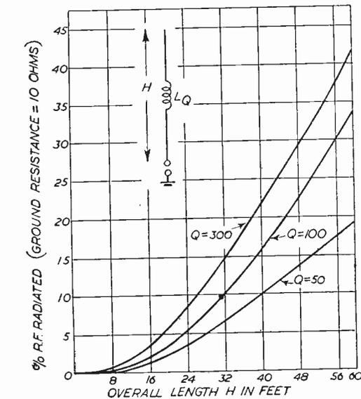
Fig. 5.—Topband efficiency of centre-loaded wires.
