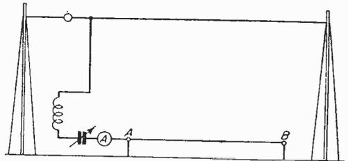
Fig. 2.—A counterpoise, AB, replaces the earth return. In some cases the end B may be earthed. Extra counterpoises may be added in a fan centred on A.
