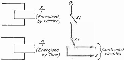
Fig. 25.—A simple receiver relay circuit operated by a carrier and single A.F. tone. The carrier by itself operates circuit 1, the carrier plus the tone operates circuit 2.
