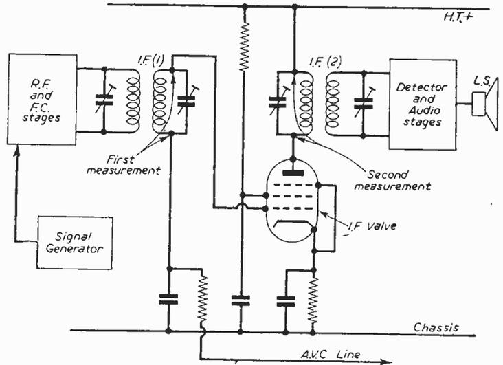
Fig. 28. — Showing the points in a typical I.F. amplifier stage at which comparative R.F. voltage measurements can be taken with a valve voltmeter.
