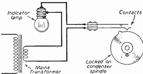
Fig. 4.—Tuning with a bulb indicator.
