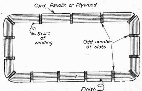
Fig. 5.—Details of a flat frame.
