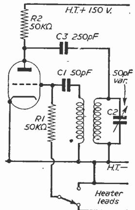
Fig. 6.—Circuit of a test oscillator which may be made up for alignment purposes.
