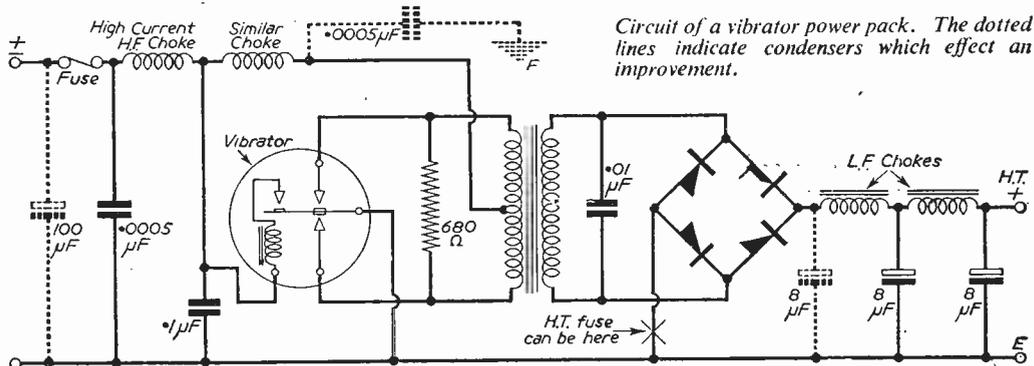
Circuit of a vibrator power pack. The dotted lines indicate condensers which effect an improvement.
