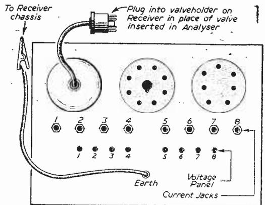
Fig. 3.—Panel layout of the instrument.
