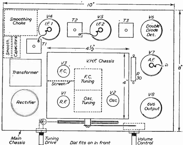
Fig. 7.—Plan of the layout showing valve positions.
