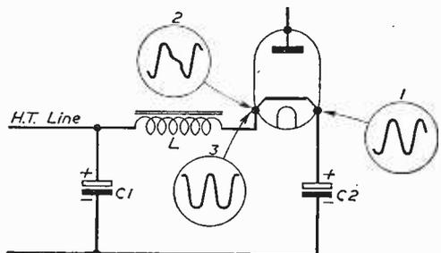
Fig. 59.—A half-wave rectifier circuit; waveforms 1 and 2 normal, and 3 due to L becoming open-circuit. Apart from the 50 c.p.s. ripple frequency, waveforms on the H.T. line are similar to those in the full-wave circuit.
