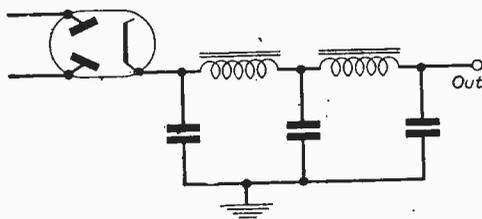
Fig. 12.—A condenser input circuit, followed by two cascaded filters for very great reduction of hum level.
