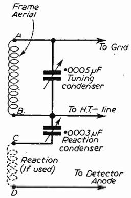
Fig. 1.—Connections for a M.W. frame aerial.
