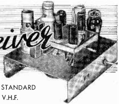
A NOVEL DESIGN OF RECEIVER FOR THE RECEPTION OF STANDARD BROADCAST SIGNALS AS WELL AS THOSE ON V.H.F.
