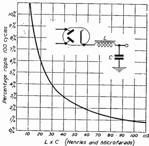
Fig. 7.—Ripple output of a choke input circuit across the following condenser. The product of L and C determines the ripple percentage.
