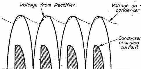
Fig. 1.—Rectifier and condenser charges.
