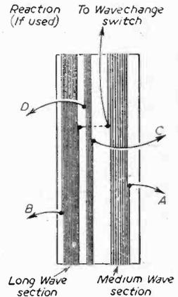
Fig. 4.—Disposition of windings on a dual-wave frame.
