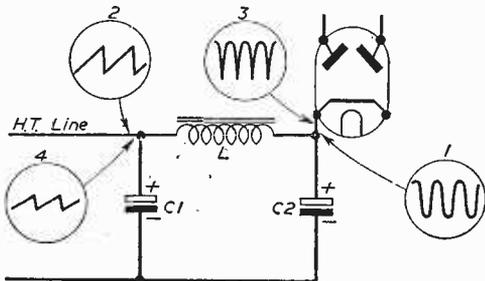
Fig. 58.—A full-wave rectifier circuit; waveforms 1 and 2 normal, 3 due to C2 becoming open-circuit and 4 due to L becoming open-circuit. Ripple frequency 100 c.p.s.
