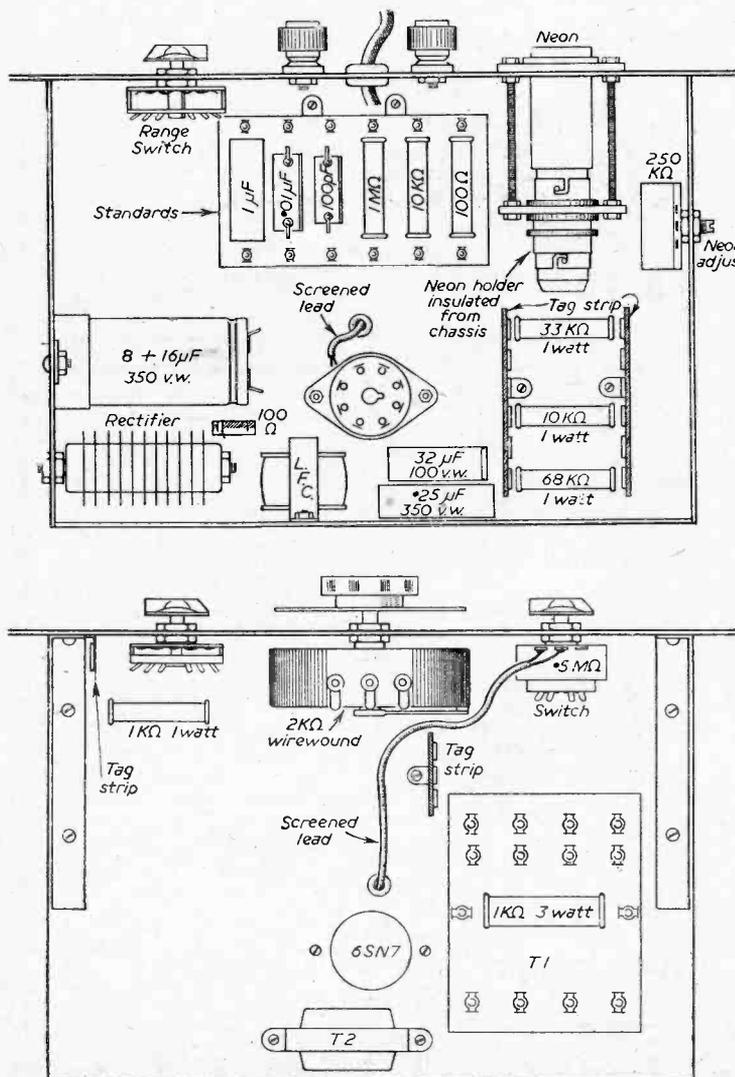
Fig. 5.—Above and below chassis wiring details.
