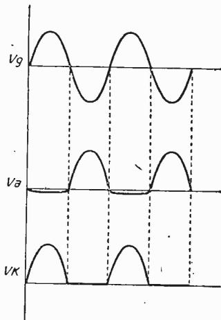
Fig. 3 (Left).—Practical Class B phase inverter. (Right).—Half sine-wave at anode and cathode for sine-wave at grid.
