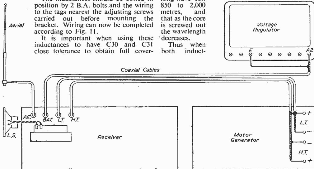
Fig. 8.—Complete installation wiring details.
