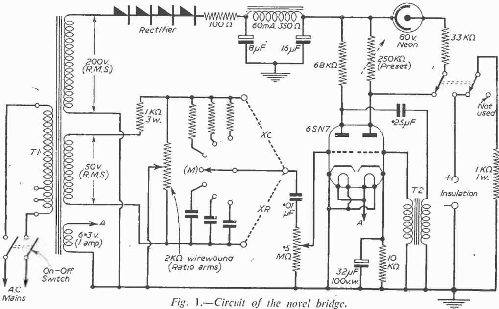
Fig. 1.—Circuit of the novel bridge.
