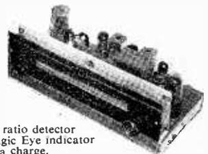
**SPECIFICATION.** The TSL FM/VHF tuner contains 5 valves and 10 tuned circuits. Grounded grid R.F. stage, additive mixer, two high gain I.F. Stages, ratio detector stage and rectifier. A Magic Eye indicator is available at a small extra charge.
