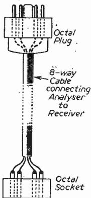
Fig. 2.—Details of the adaptor.
