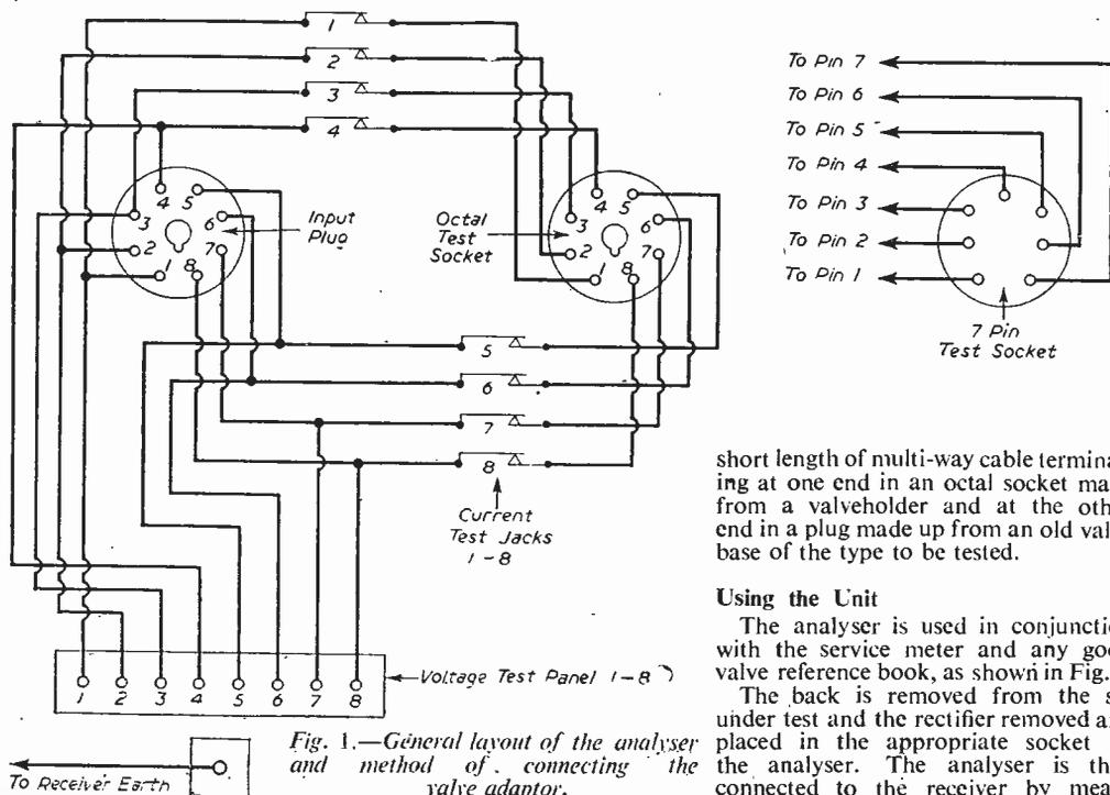
Fig. 1.—General layout of the analyser and method of connecting the valve adaptor.
