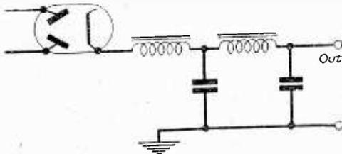
Fig. 10.—A choke input circuit followed by a filter stage gives a complete choke input power pack circuit for practical use.
