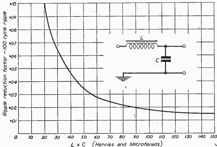
Fig. 11.—Ripple reduction factors for an LC filter stage.
