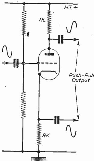
Fig. 1.—Basic phase inverter.
