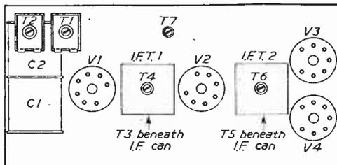
Fig. 2.—Top view of chassis showing trimmer positions.
