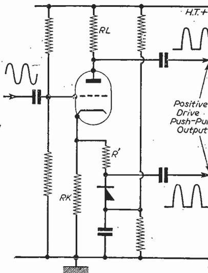
Fig. 2.—Modified phase inverter.
