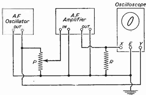
Fig. 51.—Checking the overall phase shift of an amplifier.
