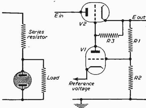
Fig. 2 (left).—Basic circuit, and Fig. 3 (right).—Basis of the new circuit.
