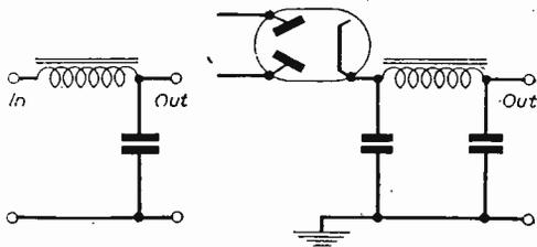
Fig. 8 (left).—A filter stage used to reduce hum. It follows the input circuit. Fig. 9 (right).—Adding a filter section to the condenser input circuit gives the familiar "power pack" circuit as used in many small power supplies.
