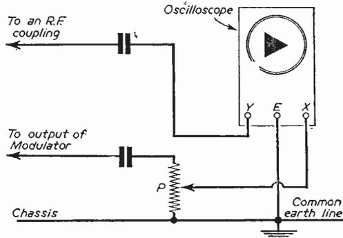
Fig. 63.—The circuit arrangement for checking modulation depth.
