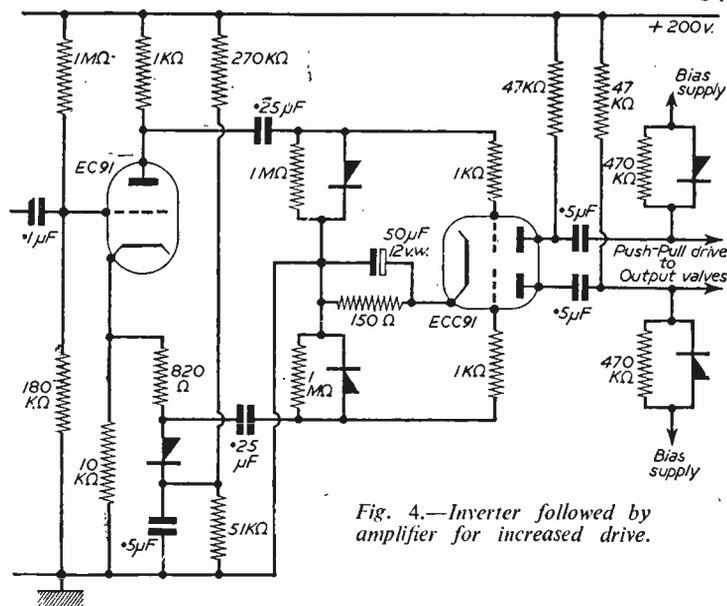
Fig. 4.—Inverter followed by amplifier for increased drive.
