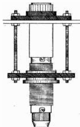
Fig. 4.—Details of the neon holder.
