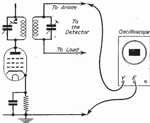
Fig. 61.—A method of connecting an oscilloscope for observing a modulated R.F. waveform.
