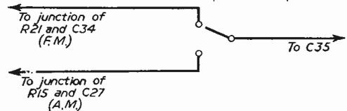
Fig. 9.—Switching to enable A.M. signals to be obtained.
