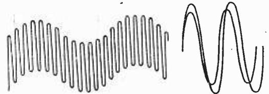
Fig. 56.—Showing the effect of 50 c.p.s. mains hum superimposed on an examination waveform.
