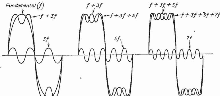
Fig. 53.—Curves showing the formation of a square-wave.
