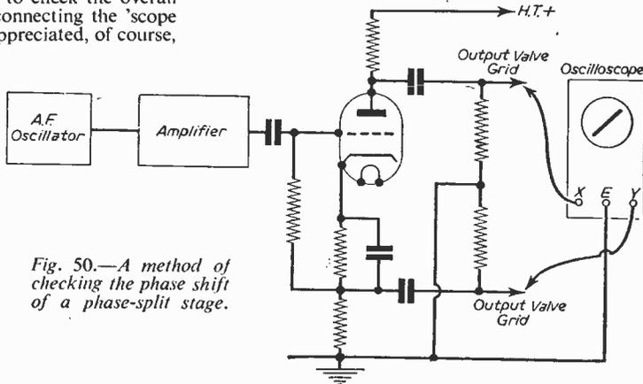
Fig. 50.—A method of checking the phase shift of a phase-split stage.
