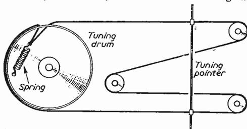
Fig. 3.—Details of the tuning drive arrangement.
