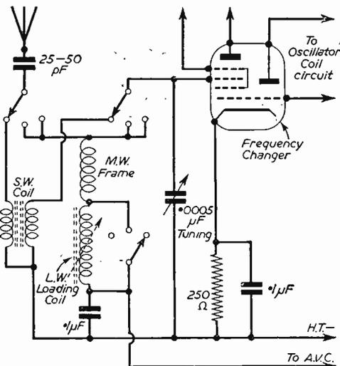
Fig. 2.—Typical all-wave circuit.
