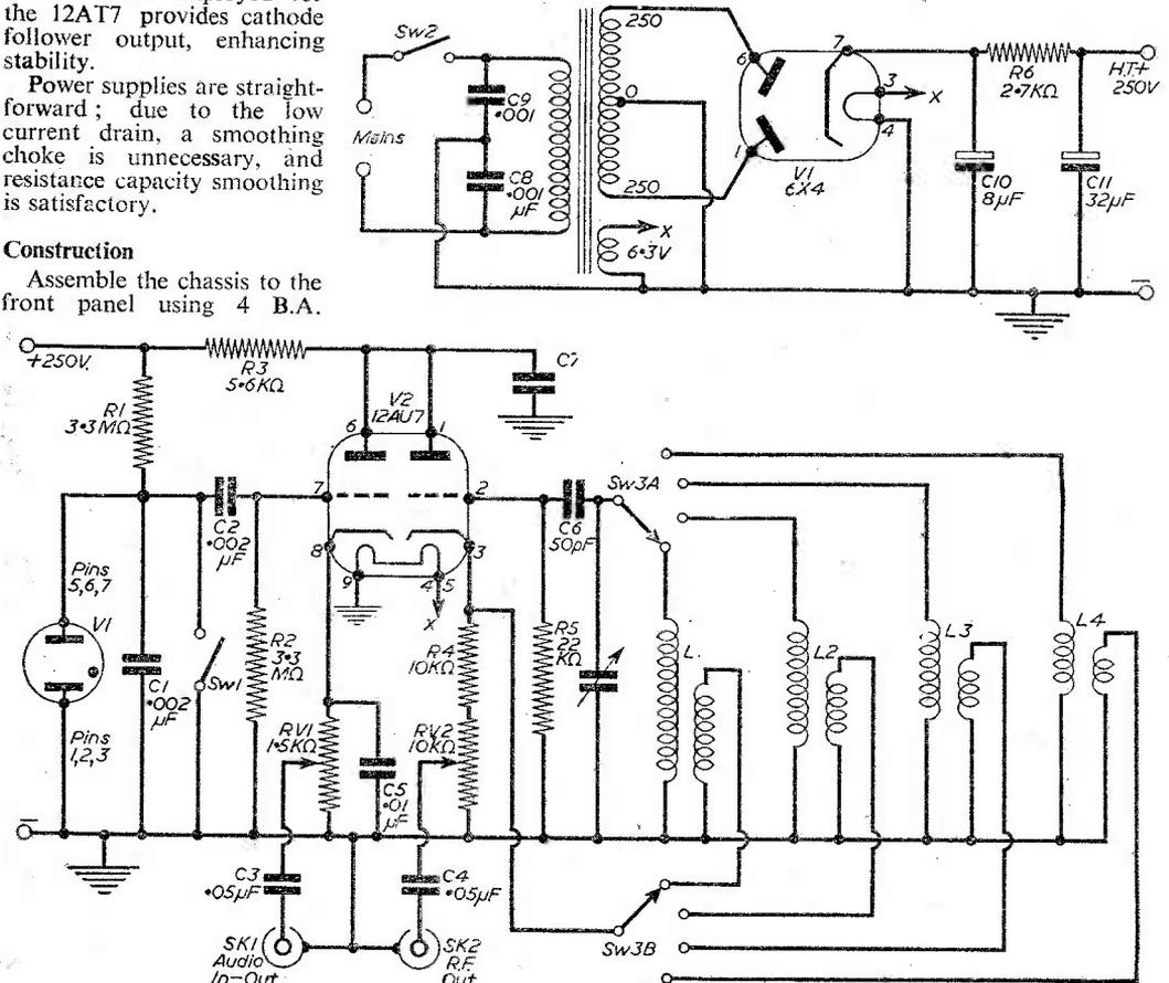
Fig. 1.—Theoretical circuit of the generator, with the mains section above.
