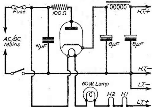
Fig. 3.—The A.C./D.C. version of the power-pack.
