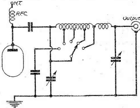
Fig. 4.—The L/C ratio required for 80-metre operation can be achieved by switching in an auxiliary fixed capacitor across the main tuning capacitor. This enables the main capacitor to be a convenient size for comfortable tuning of the higher frequency bands.
