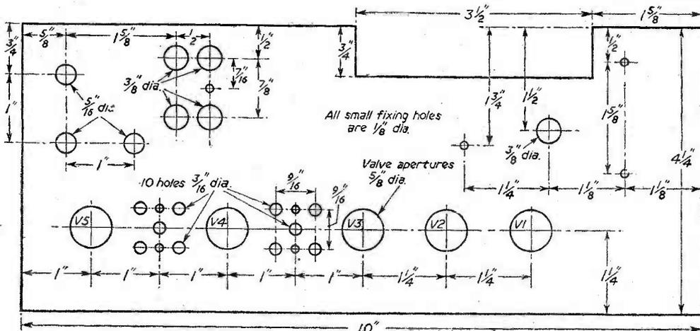
Fig. 2.—Drilling and other data for the chassis.
