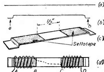
mu-metal  $\frac{1}{16}$  in. wide by approximately 2 in., 40-43 s.w.g. insulated copper wire (not cotton or silk covered), small pieces of mica, two 4 B.A. nuts and bolts, lead out wire and paraffin wax.
