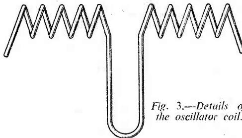
Fig. 3.—Details of the oscillator coil.
