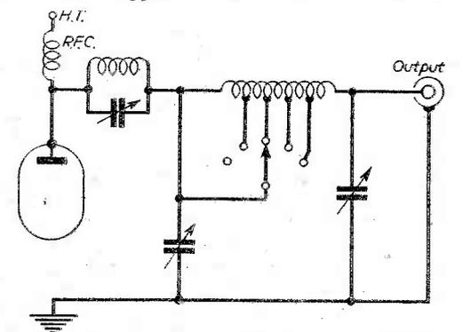
Fig. 3.—A separate coil section for 10 metres obviates short-circuit losses for H.F. operation.
