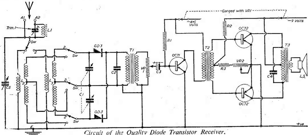
Circuit of the Quality Diode Transistor Receiver.
