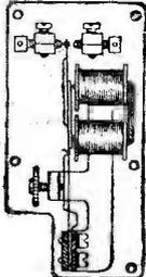
This is a miniature type relay with changeover platinum contacts. Bobbins are 250 ohms each.
