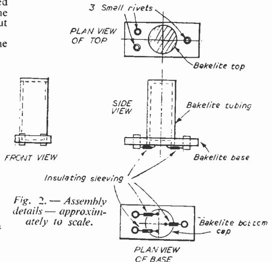
Fig. 2.—Assembly details—approximately to scale.
