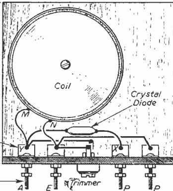
Fig. 4.—Plan of the first set, showing wiring.
