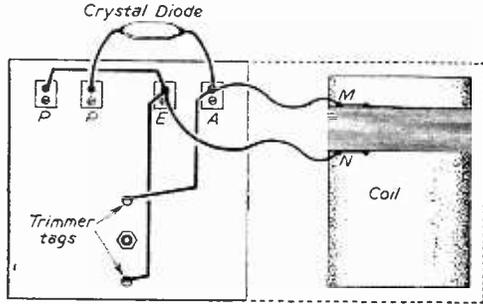
Fig. 6.—Coil and crystal wiring.
