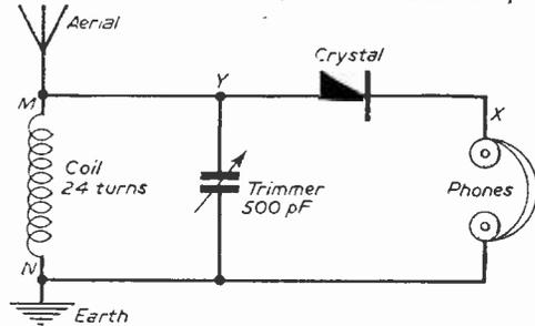
Fig. 5.—Theoretical circuit of the crystal set.
