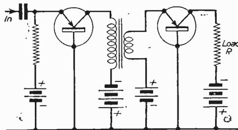
Fig. 3.—A transformer-coupled common base amplifier.
