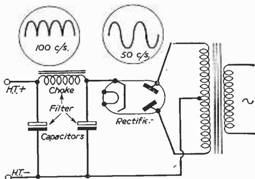
Fig. 3.—Principle of the circuit.
