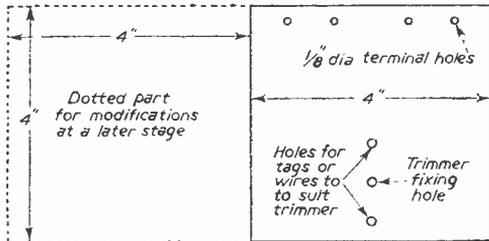
Fig. 1 (a).—Details of the front panel made from  $\frac{1}{4}$  in. plywood.
