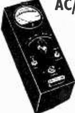
Comprising 2 in. moving coil meter, scale calibrated in A.C./D.C. volts, ohms and milli-amps. Voltage range AC/DC 0-10, 0-100 and 0-500, Milli-amps 0-10, 0-100. Ohms 0-3,000 and 0-10,000. Front panel, range switch, wire-wound pot (for ohms zero setting) two toggle switches, resistors and meter rectifier. In grey hammer-finish case.
