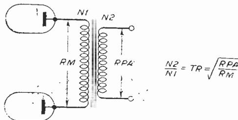
Fig. 2.—The turns ratio of the modulation transformer is calculated by the relationship shown above.  $R_M$  is the required load value for the modulator valve or valves, while  $R_{PA}$  is the effective resistance presented by the P.A. stage.  $N_1$  and  $N_2$  are the number of turns in the primary and secondary windings respectively. In practice the ratio of turns  $TR$  is all that need be known to effect a match.
