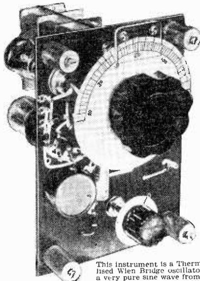
This instrument is a Thermistor stabilised Wien Bridge oscillator providing a very pure sine wave from 20 c.p.s. to 20 KCS., in three ranges. High accuracy of calibration and constancy of output voltage are features making this an exceptionally useful instrument for the testing of high-fidelity equipment. Send stamp for full details.
