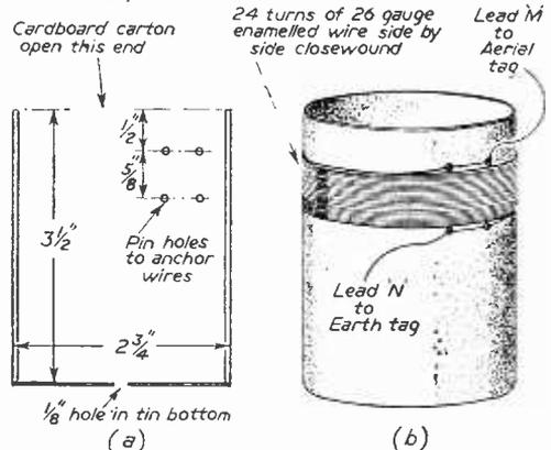
Fig. 3.—Details of the tuning coil.
