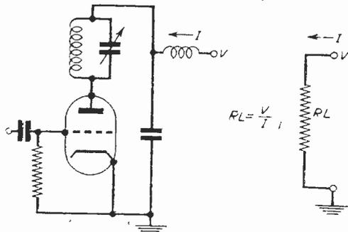
Fig. 1.—The "load impedance" of the P.A. stage for modulation purposes, is calculated as a purely ohmic resistance by Ohm's Law. In other words, the resistance corresponding to the P.A. plate current drawn at the applied plate voltage is calculated as for any other type of resistance.
