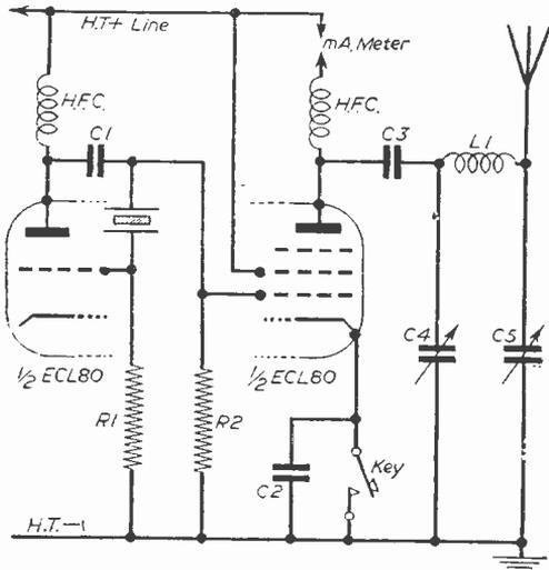
Fig. 1.—The original 1-valve circuit.
