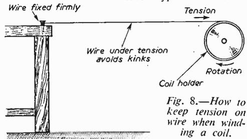
Fig. 8.—How to keep tension on wire when winding a coil.
