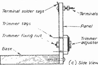
Fig. 1 (c).—Side view of panel and baseboard.
