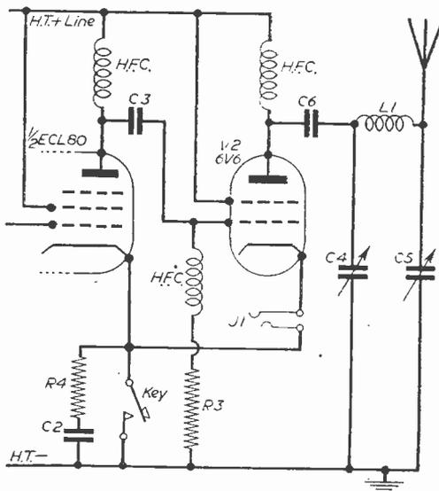
Fig. 2.—The new P.A. stage.
