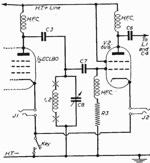
Fig. 3.—Modification to enable frequency doubling to be effected in the pentode section of the ECL80.
