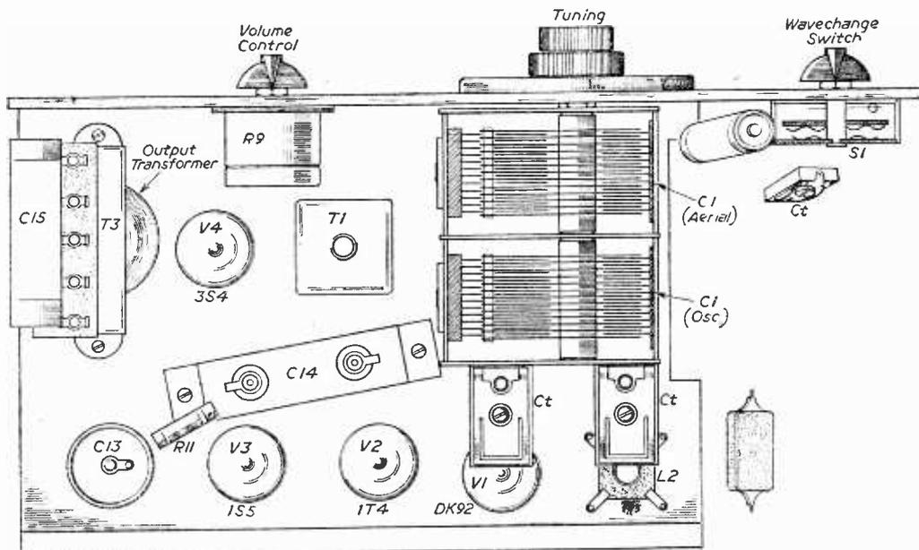
Fig. 3.—Top wiring details.
