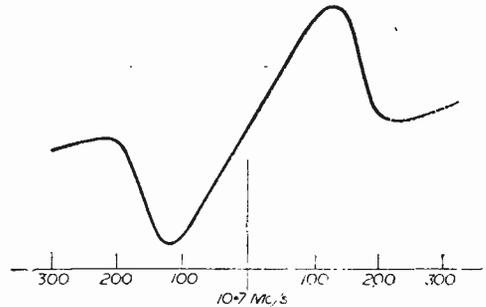
Fig. 6.—Result obtained after the third I.F. transformer is adjusted.
