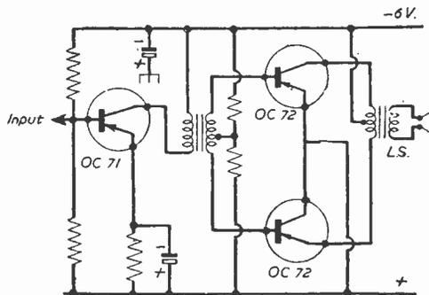
Fig. 2.—A transistorised output stage.
