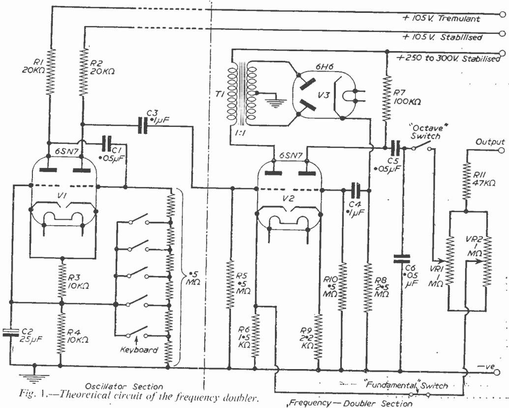
Fig. 1.—Theoretical circuit of the frequency doubler.
