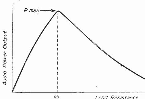
Fig. 4.—With constant audio grid drive, the power output from Class AB2 and Class B valves varies from the maximum output, and maximum audio output is obtained at one load value RL. Any other value of load impedance results in a loss of audio power. With values of R greater than RL, increased grid drive results in severe peak clipping. With load values less than RL, excessive drive may give increased output, at a cost of grid heating and excessive anode peak currents. (See text.)
