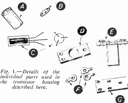
Fig. 1.—Details of the individual parts used in the transistor housing described here.
