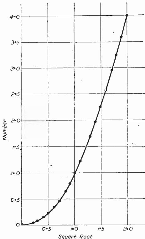
Fig. 3.—A graph of square roots produced by the "Inverse Method" of squaring a series of numbers, enables a useful square root graph, suitable for modulation ratio determination, to be drawn. The original series of numbers provides the square root values corresponding to numbers obtained by squaring the original series. As will be seen the graph was obtained by squaring a number sequence arranged in steps of 0.1.
