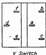
The lettering is given looking at back of switch towards the front panel
