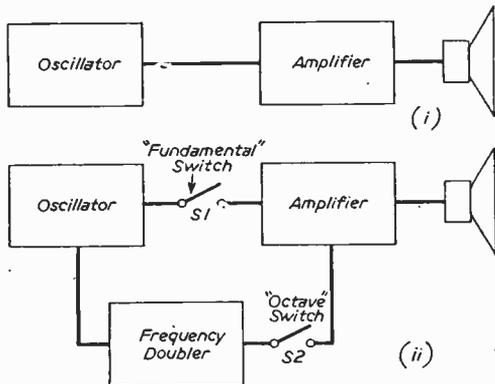
Fig. 4.—How the unit is incorporated in an organ.
