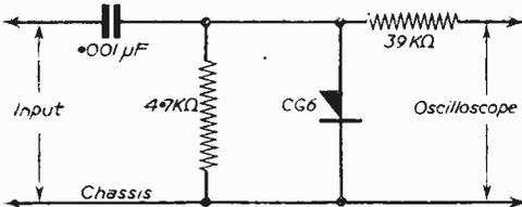
Fig. 5.—Detector assembly which should be used with the scope.
