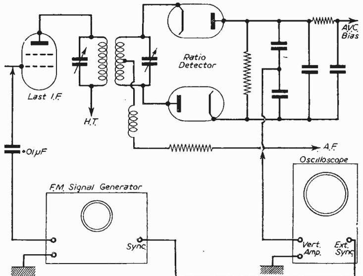
Fig. 3.—The set-up with ratio detector.
