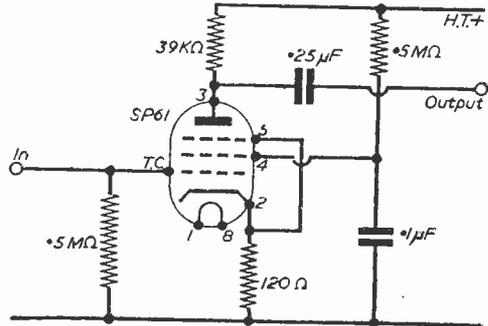
Fig. 9.—A one-valve switch.
