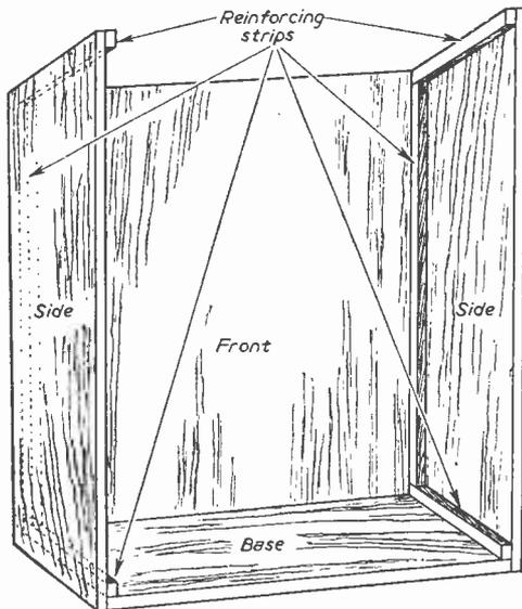
Fig. 5.—Assembly details of the case.
