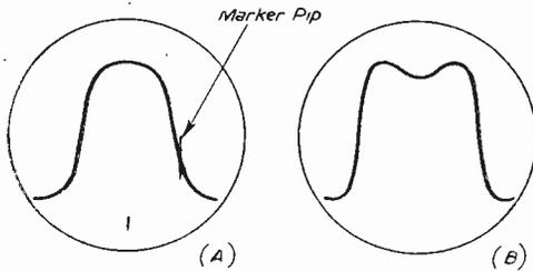
Fig. 4.—Curves obtained when the I.F.s are adjusted correctly.
