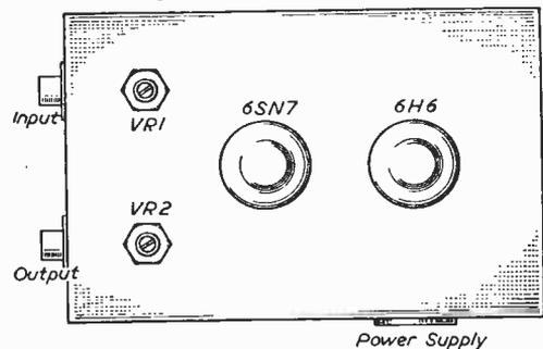
Fig. 5.—Suggested layout for frequency doubler circuit only.
