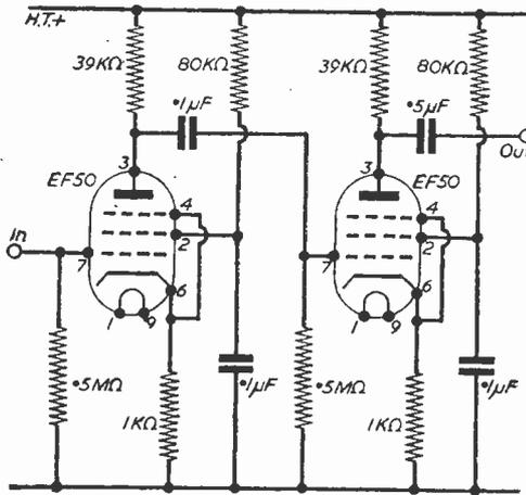
Fig. 8.—A two-valve switch.
