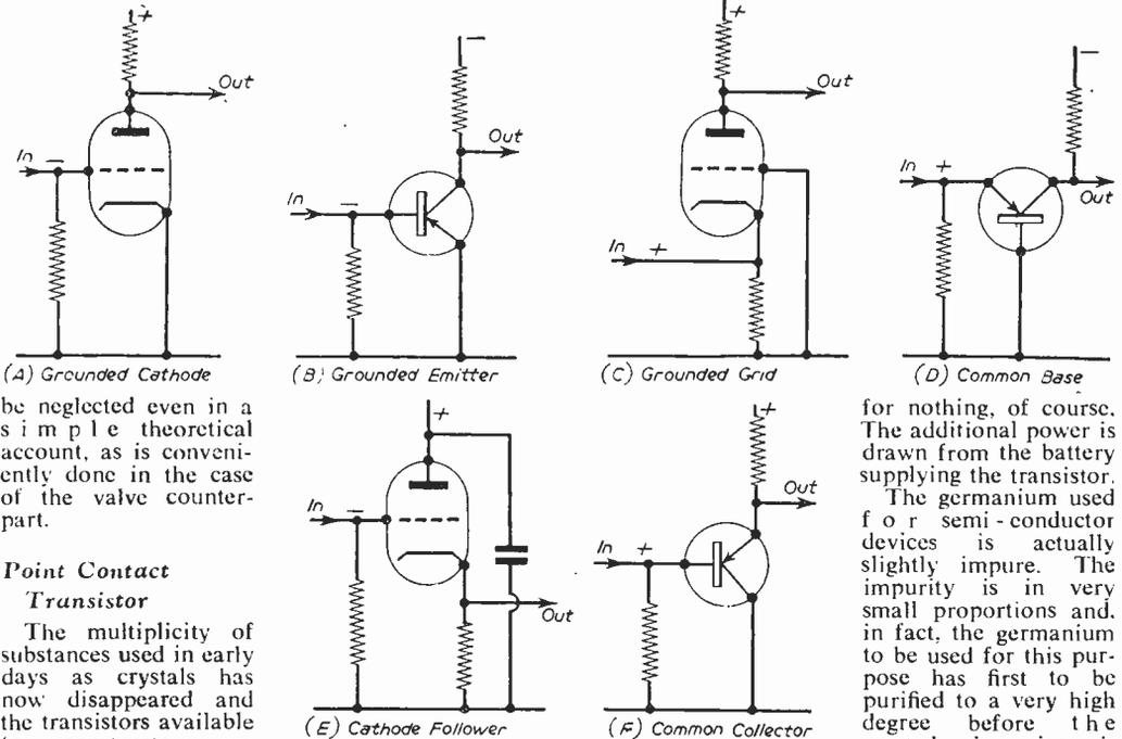
Fig. 1.—Diagrams showing comparison between the triode valve and the transistor. The signs indicate D.C. potentials with regard to earth.
