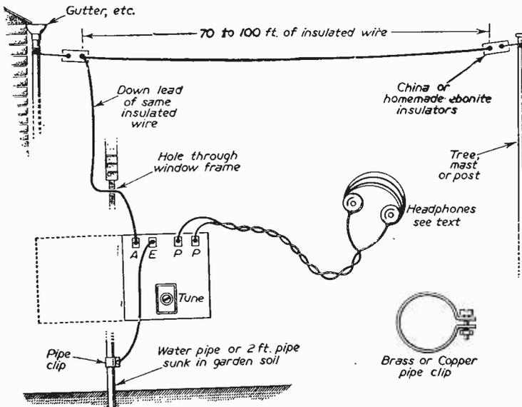
Fig. 7.—General layout for a crystal receiver.
