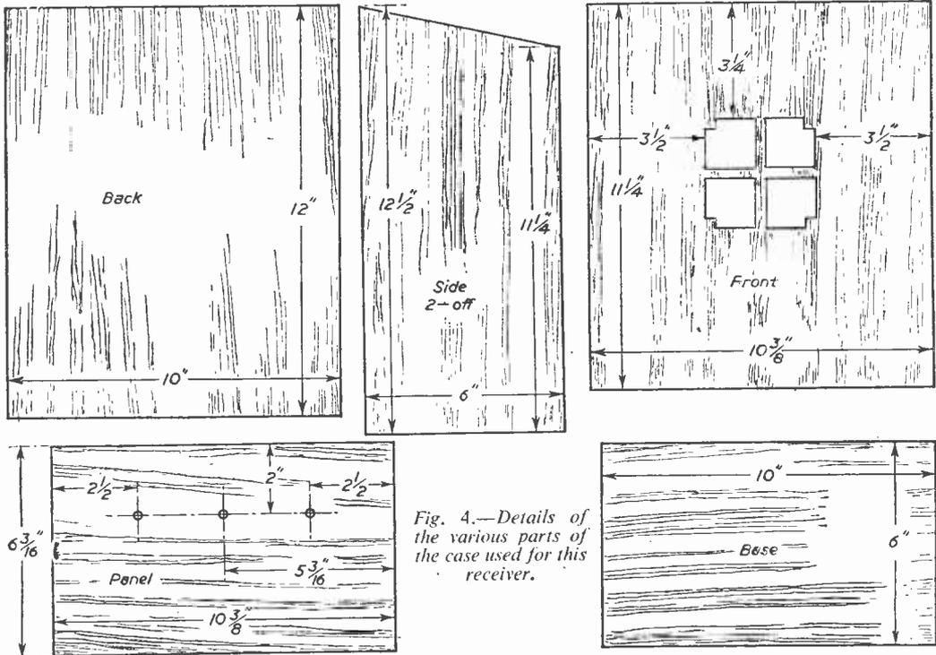
Fig. 4.—Details of the various parts of the case used for this receiver.
