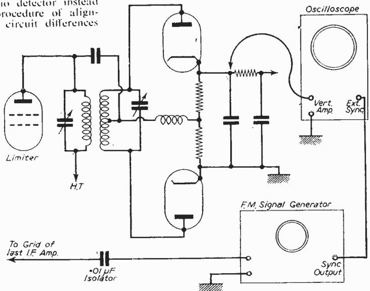
Fig. 1. The set-up of scope and discriminator stage.
