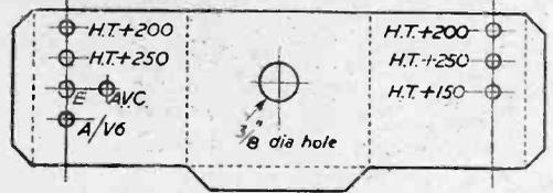
Fig. 7.—Screen for feeder chassis.
