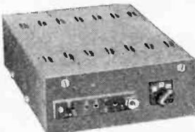
Type BM2. Size 8 x 5 1/2 x 2 1/2 in. Supplies 120 v. 90 v. and 60 v. 40 mA. and 2 v. 0.4 a. to 1 amp. fully smoothed. Thereby completely replacing both H.T. batteries and L.T. 2 v. accumulators. When connected to A.C. mains supply 200-250 v. 50 ccs.
