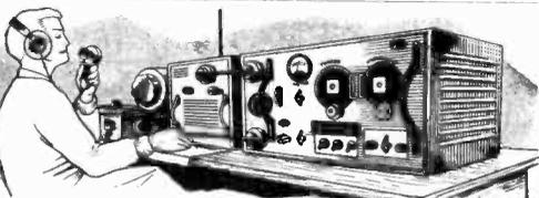
● THE WIRELESS SET No. 19 incorporates a VHF Transmitter/Receiver covering 230 to 240 Mc/s. and an intercom system. Tuning meter giving aerial and all voltage readings. Complete installation as illustrated.
