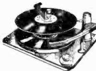
4-speed plays 10 records 12in. 10in or 7in. at 16, 33, 45 or 78 r.p.m. Intermixes 7in., 10in and 12in. records of the same speed. Has manual play position; colour brown. Dimensions: 12 1/2in. x 10 1/2in. Space required above baseboard 4 1/2in., below baseboard 2 1/2in. Fitted with Full-Fi turnover crystal head.
