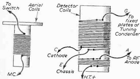
Fig. 4.—Construction of the aerial and detector coils.
