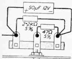
Fig. 3.—Wiring of the sub-assemblies for the triode stage.
