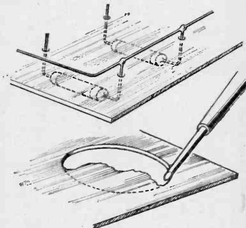
Fig. 1.—Method of fixing resistors and making holes in the plastic sheeting.
