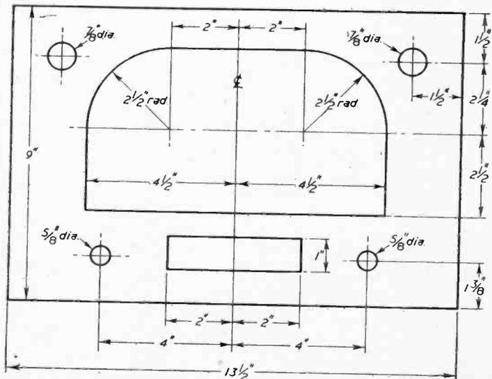
Fig. 8.—The front panel.
