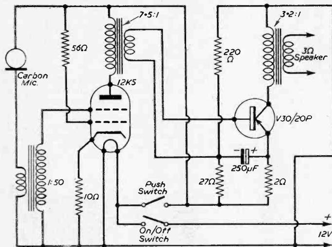
Fig. 3.—Circuit with valve pre-amplifier for 12V operation.
