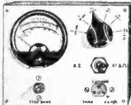
Comprising 2in. moving coil meter, scale calibrated in A.C./D.C. volts, ohms and milliamps. Voltage range A.C./D.C. 0-50, 0-100, 0-250, 0-500. Milliamps 0-10, 0-100. Ohms range 0-10,000. Front panel, range switch, wire-wound pot (for ohms zero setting), toggle switch, resistor and rectifier. In grey hammer finish case.
