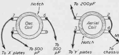
Fig. 4.—Aerial and oscillator coils.
