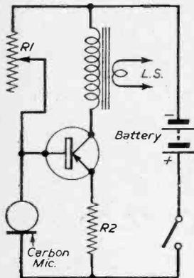
Fig. 1.—Directly coupled circuit.
