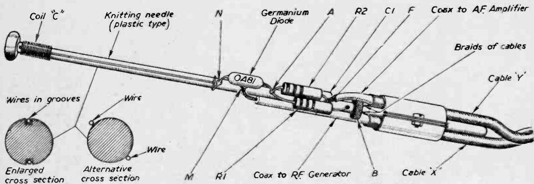
Fig. 2.—Construction and wiring of the "Needle."
