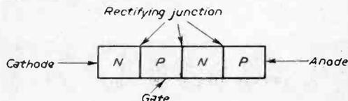
Fig. 1.—Diagram of the device.
