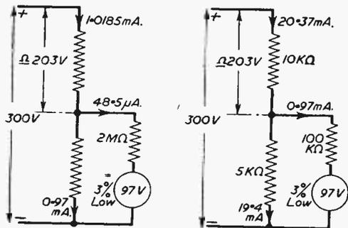
Fig. 3 (Left).—Result of using a meter of 20,000 $\Omega/V$ .
