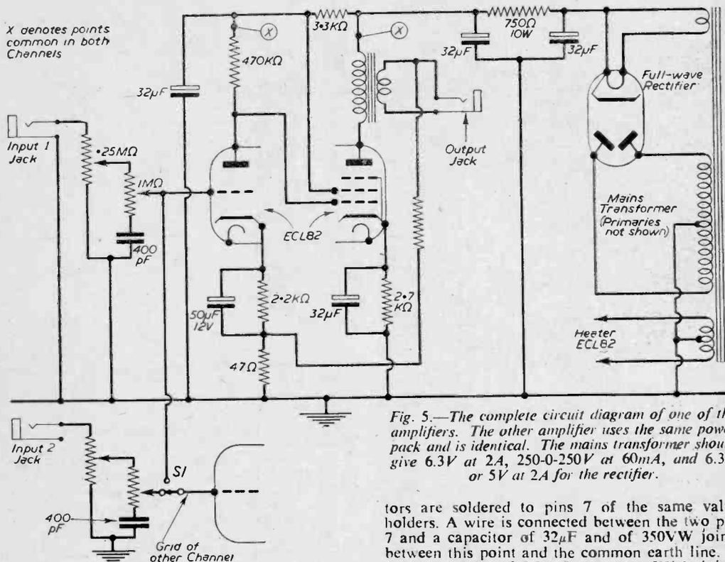
Fig. 5.—The complete circuit diagram of one of the amplifiers. The other amplifier uses the same power pack and is identical. The mains transformer should give 6.3V at 2A, 250-0-250V at 60mA, and 6.3V or 5V at 2A for the rectifier.
