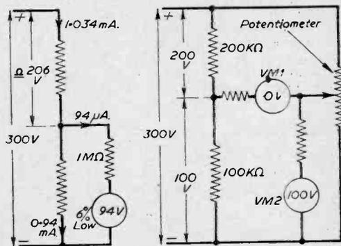
Fig. 5 (Left).—Effect on the circuit conditions of Fig. 2 when the meter is switched to a higher range.
