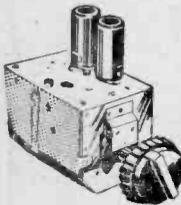
Ideal for converting an old or building into new T.V. These are brand new stock, not surplus, supplied complete with valves and coils for local Band I and Band III stations. Model 1. I.F. Output 33.33 Mc/s series heaters (parallel heaters, 5/- extra).
