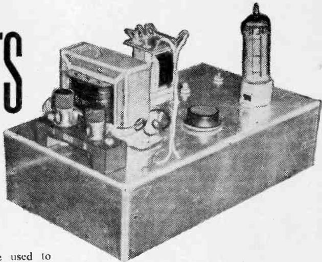
A TRANSISTOR amplifier can be used to work a loudspeaker for sports, outdoor events, and similar functions, and this type of equipment can be independent of the need for mains or accumulator supplies. It is not practicable to obtain volume equalling that of a large mains-operated public address amplifier, which may deliver many watts, but a useful output can nevertheless be obtained.
