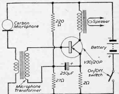
Fig. 2.—Adding a coupling transformer.
