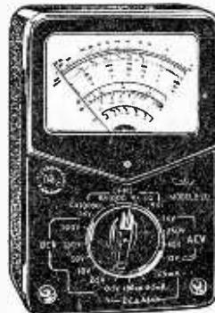
**MODEL A-10 (500 Micro-amp Movement).** D.C. (2k per volt) 0/10/50/250/500/1000 v. A.C. (2k per volt) 0/10/50/250/500/1000 v. D.C. current 0/0.5/25/250 mA. Resistance: 0/10K/1 Meg. Size: 5½ x 3½ x 1½in. Weight: 17 ozs. Price £4.17.6, P.P. 1/6 inclusive of Test Prods, Instruction Book and Batteries
