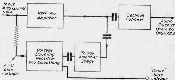
Fig. 3.—Block diagram of the proposed AVC system.
