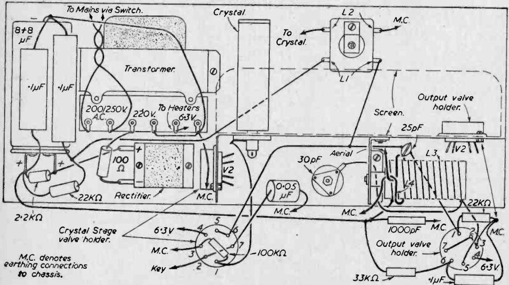
Fig. 2.—Wiring and the layout of the components.
