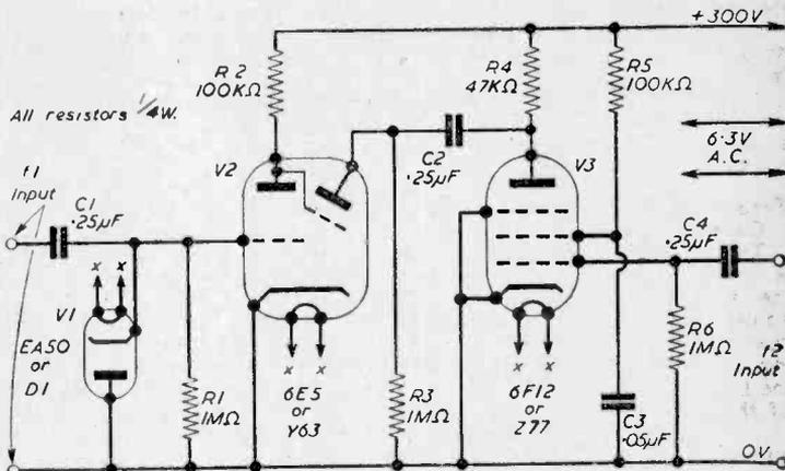
Fig. 4.—Frequency comparator circuit.
