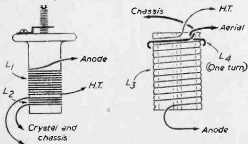
Fig. 3.—Details of the coils.
