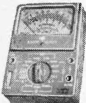
A.C. and D.C. 3333 ohms per volt. Ohms ranges up to 2 megs. Volts A.C. and D.C. up to 1,200. 300 micro-amps—300 m/a. Decibels, 2 ranges, —20 to +23 and —20; to +37 db. Accuracy  $\pm 3\%$ . Large full vision dial. Overall size:  $5\frac{1}{2} \times 3\frac{3}{8} \times 1\frac{1}{2}$  in.
