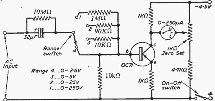
Fig. 4.—The complete circuit of the voltmeter.
