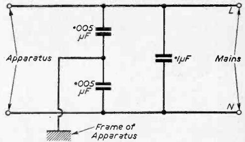
Fig. 6.—Suppressor circuit for connecting in the flex lead to the apparatus concerned. This must be wired as close to the offending apparatus as possible—within 6in.
