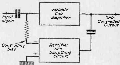
Fig. 1.—Block diagram of the AVC unit.
