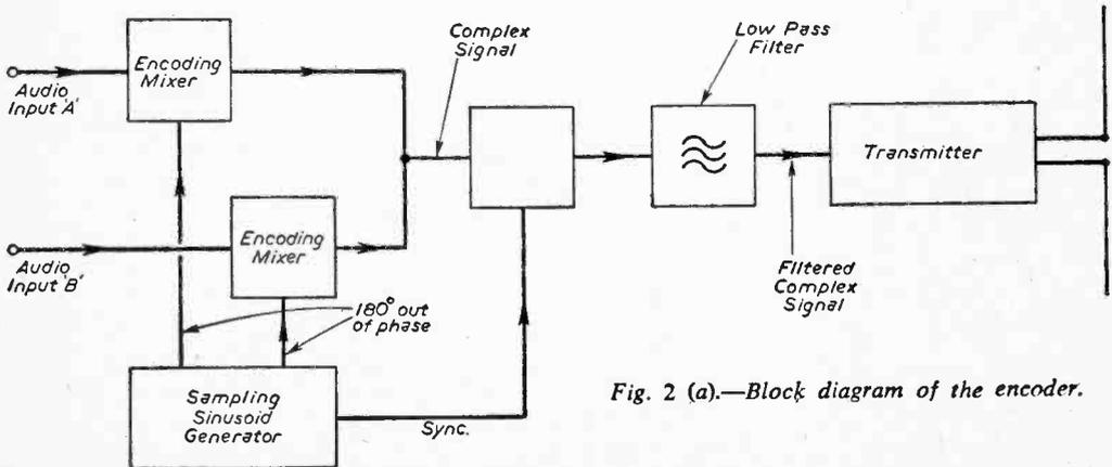
Fig. 2 (a).—Block diagram of the encoder.
