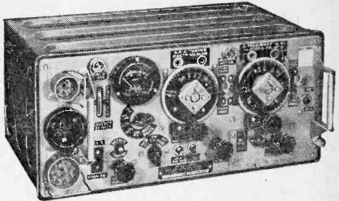
IN the two previous articles, information has been given on modifications to the receiver section of the No. 19 Set and the intermediate testing was discussed. A circuit for a Q-multiplier to improve selectivity was also given. The valve used in this circuit was half of a 12AX7 double triode and in the circuit diagram (Fig. 6, page 1028 of the April issue) the unmarked coil is a high inductance R.F. choke. The remaining two coils are QA5/6/300 types, L1 being 7.5 to 3mH and L2 120-150μH.
