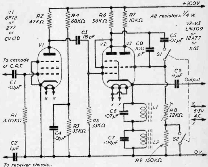
Fig. 1.—The circuit of the calibrator.
