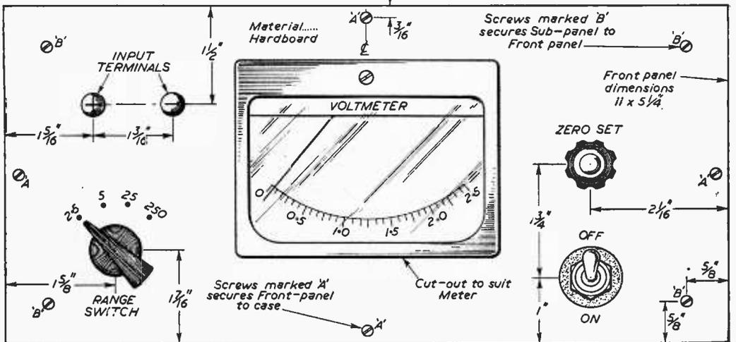
Fig. 5.—Layout and measurements of the front panel.
