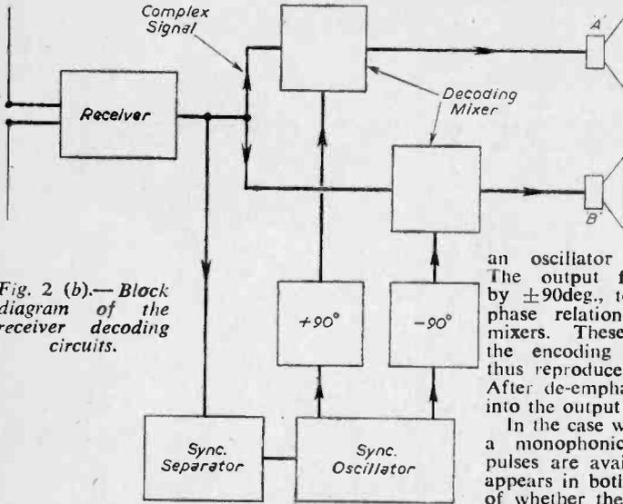
Fig. 2 (b).—Block diagram of the receiver decoding circuits.
