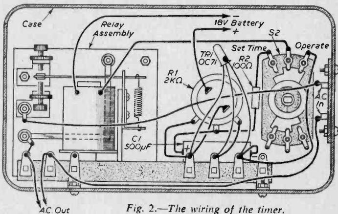
Fig. 2.—The wiring of the timer.
