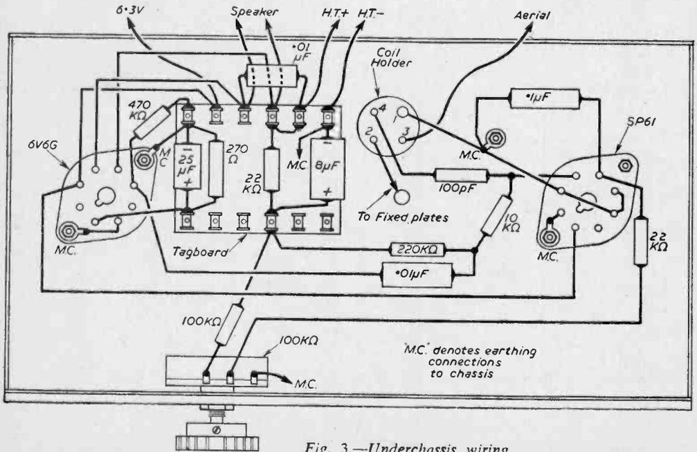
Fig. 3.—Underchassis wiring.
