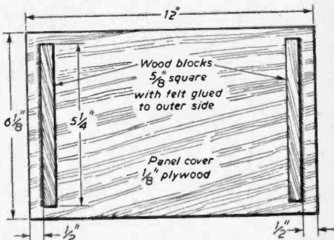
Fig. 26.—Felt glued to the wooden battens, makes the front panel a push-fit.
