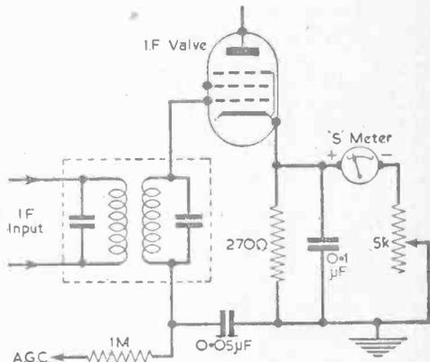
Fig. 2.—A circuit using a 1mA meter.
