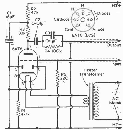
Fig. 2 (right).—A modified circuit for A.C./D.C. amplifiers.
