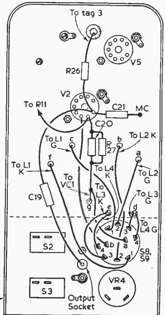
Fig. 10 (right).—The underchassis wiring.
