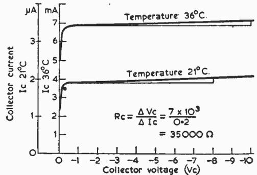
Fig. 2.—Collector-diode curves.
