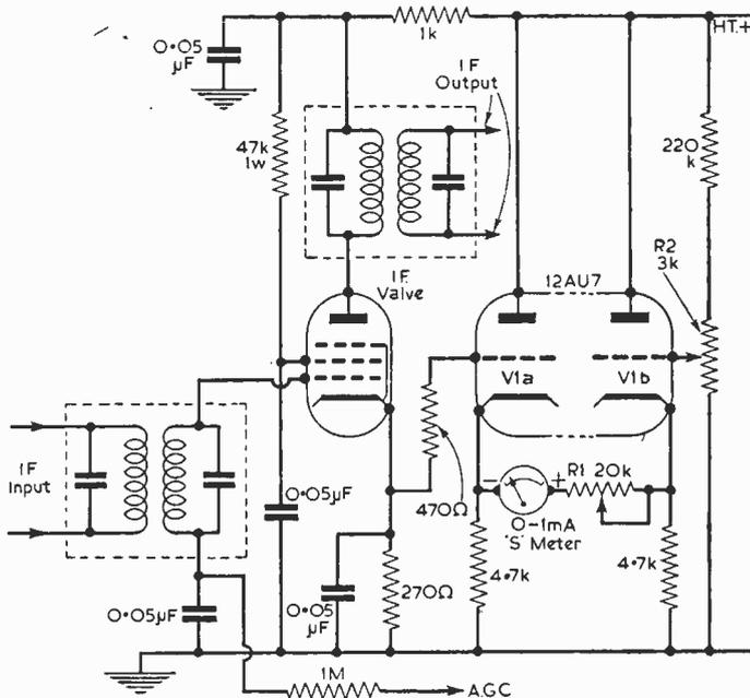
Fig. 5.—A circuit which employs a double triode.
