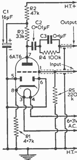
Fig. 1 (left).—The basic circuit of the booster unit.
