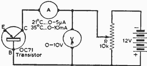
Fig. 1.—The collector-diode test circuit.
