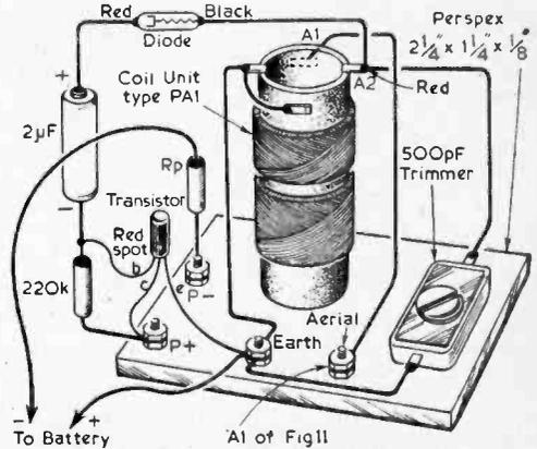
Fig. 12 (above).—Layout of the crystal diode receiver. (The collector of the transistor is indicated either by a spot of paint near to it or by wider spacing from the middle wire, which is the emitter. The remaining wire is the emitter.)
