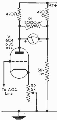
Fig. 4.—A circuit which requires an extra valve.
