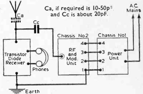
The units are wired as shown in Fig. 13 for the test. If an ordinary receiver is used the wiring is the same. If the receiver is sensitive then the aerial need only be short, if insensitive it must be long. Ca may be necessary for reasonable selectivity if a long aerial is used on very simple receivers.
