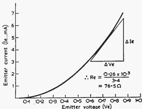
Fig. 4.—Emitter-diode curve.
