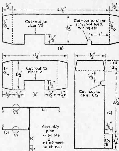
Fig. 6.—Details of the screens and their assembly.
