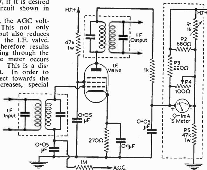
Fig. 3.—A forward-reading circuit.
