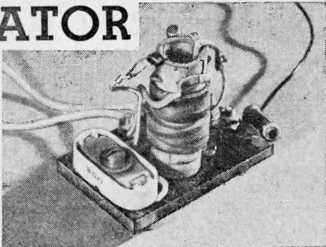
A view of the crystal receiver used for testing.
