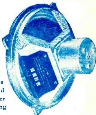
This range of Stentorian loudspeakers, incorporating the patented cambric cone, was developed to provide reproduction that takes full advantage of the television and V.H.F. sound transmissions and high fidelity recordings now available. The cone of the loudspeaker is made from uncured cambric and bonded pulp, the whole being completely cured together and made into one composite cone.
