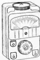
A must for all home constructors. Basic movement 300µA. Sensitivity 1,000/V. A.C. and D.C. Ranges 10-50-250-500-1,000V. D.C. and A.C. 1-100-500mA. D.C. 2K/200K ohms. Accuracy: 3% FSD and D.C. 5% F.S.D. and A.C. 10% on Resistance scale. Dimensions 5½ x 3½ x 2½ in. Complete with test leads, prods and 1.5V cell. **59/6**
