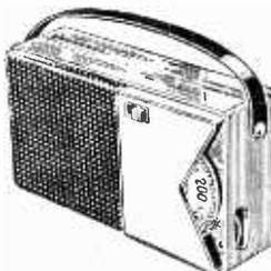
In attractive two-tone contemporary case, with gold plated speaker grille and attractive dial. Size only 5½ x 3½ x 1½ ins. No aerial or earth required—completely self contained. Genuine 3in. high flux PM speaker. First grade transistors. Push pull output—250 milliwatts. Volume control with on/off switch. Condenser tuning. Easy assembly on eyeletted circuit board. Total Building Cost **£4.19.0** P. & P. 2/6. (Long wave 6/- extra).
