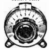
A precision vernier dial with approx. 8 to 1 ratio. Surface mounting. Accurately centred metal insert for fin. shaft. Reads counter clockwise 0-100 in 180°. 1 1/2in. diameter dial. 13/16in. front to back 14/-, Post Paid.
