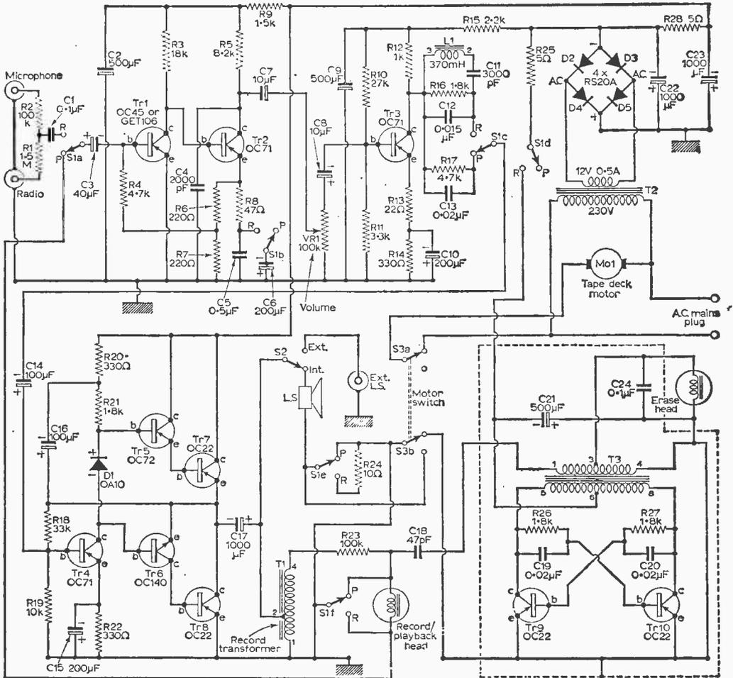
Fig. 1: The complete circuit of the recorder.
