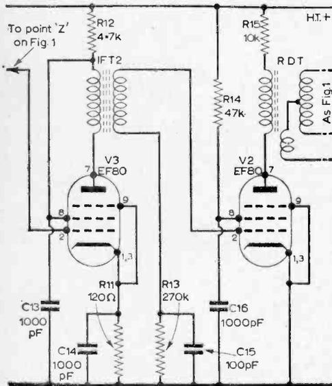
Fig. 5: The circuit employing an additional i.f. stage.
