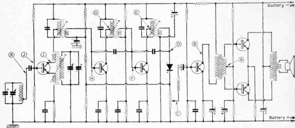
Fig. 11: A typical transistor superhet circuit.
