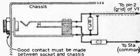
Fig. 5: Connections to the jack socket, JK1.
