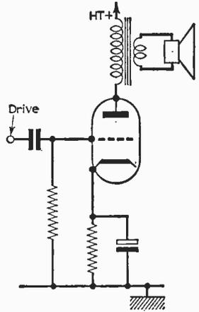
the r.m.s. current swing thereby represented is, as always, about a third of the peak-to-peak swing, i.e. some 6mA in our example. We know that 6mA flowing in  $5k\Omega$ , develops some 180 milliwatts of power, which is therefore roughly the actual power output to be expected in our example. This example corresponds roughly to that which would be achievable with a EC92 valve, and shows in general how to calculate expected power output in designing such cathode followers.
