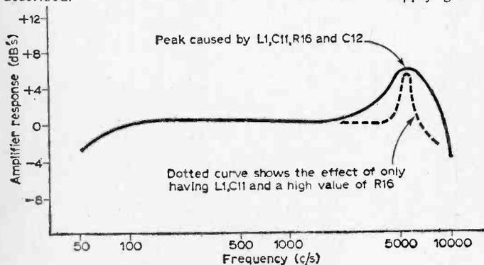
Fig. 2 (above): The record response curve.
