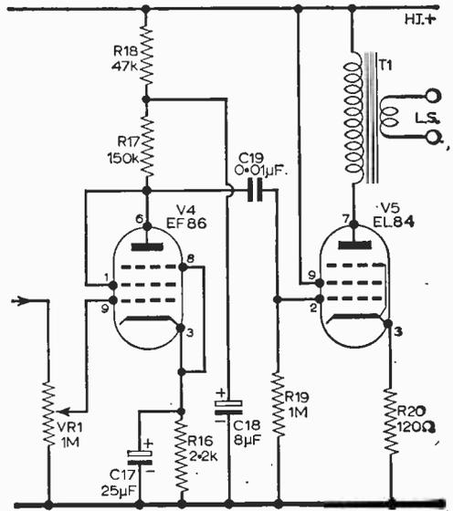
Fig. 7 (above): The a.f. amplifier circuit.
