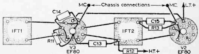
Fig. 6: The wiring of the additional i.f. stage.
