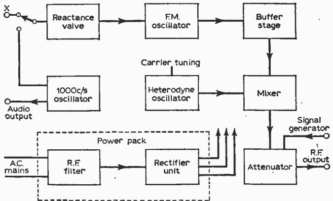
Fig. 7: Block diagram of the Cosor 1324 f.m. alignment generator.
