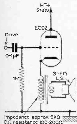
Fig. 1: A typical low-power cathode follower output stage for use in audio frequency applications.
