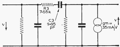
Fig. 2:  $\pi$  circuit for OC45 at  $470kc/s$  only.
