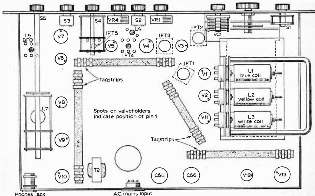
Fig. 6: Under-chassis layout of components.
