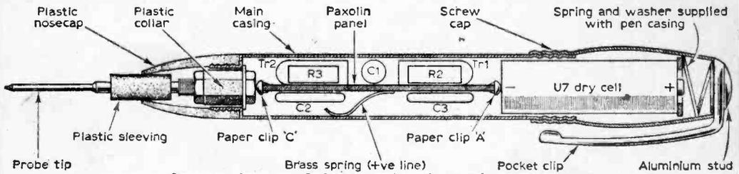
Sectional view of the completed signal injector.
