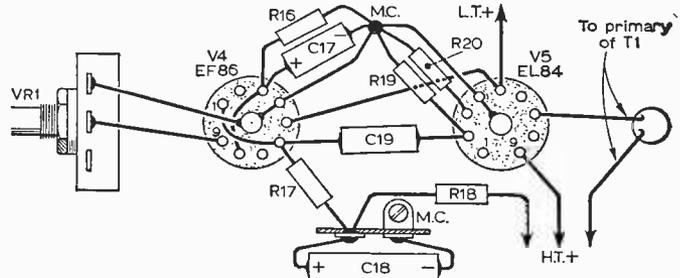
detector stage to the volume control to eliminate 50c/s hum. Another useful precaution in this respect would be to keep the leads carrying the heater current well away from all a.f. points.
