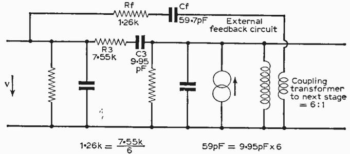
will be  $nC3$  and  $R3/n$ . At a ratio of  $6:1$ ;  $Rf=1.26k\Omega$  and  $Cf=59.7pF$ . The equivalent circuit with both internal and external feedback paths is in Fig. 3.
