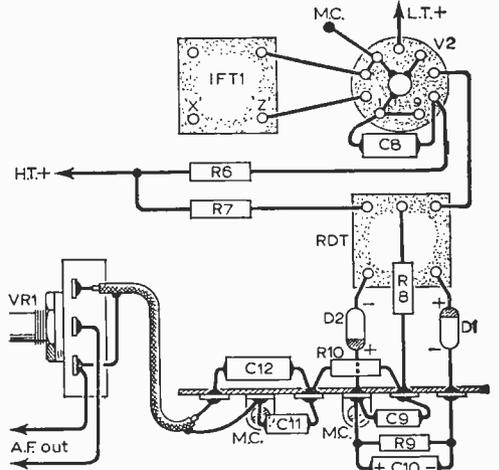
Fig. 4: The i.f. and detector stages wiring diagram.
