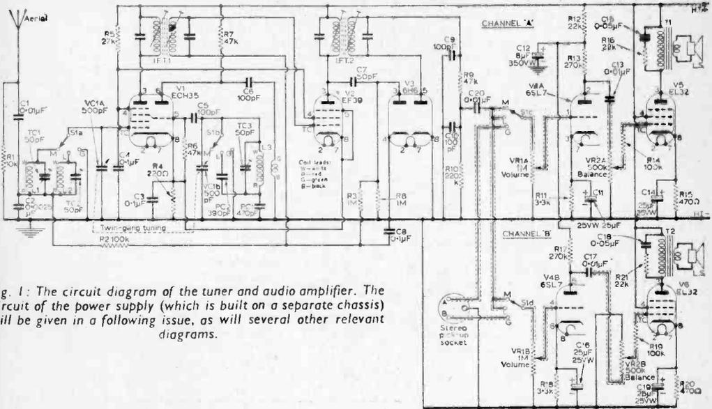
Fig. 1: The circuit diagram of the tuner and audio amplifier. The circuit of the power supply (which is built on a separate chassis) will be given in a following issue, as will several other relevant diagrams.
