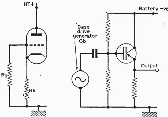
Fig. 3 (left): Basic circuit of a cathode follower circuit.
