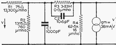
Fig. 1: Hybrid  $\pi$  circuit for OC45 at any frequency.
