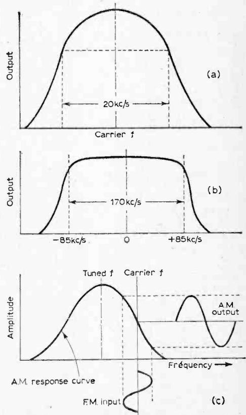
Fig. 3: Response curves of a.m. and f.m. receivers.
