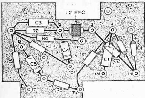
Fig. 2: Showing the arrangement of the majority of the components.
