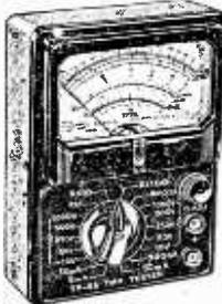
**20,000 OHMS PER VOLT MODEL TP-58** (Illustrated). Reads voltages up to 1,000 D.C. at 20,000 ohms per volt and A.C. at 10,000 o.p.v.; D.C. current to 500 mA; Resistance to 10 Megs. Capacitance to 0.1µF; Decibels from -20 to +36. Size 3¼ x 5¼ x 1¼ in. £5.19.6.
