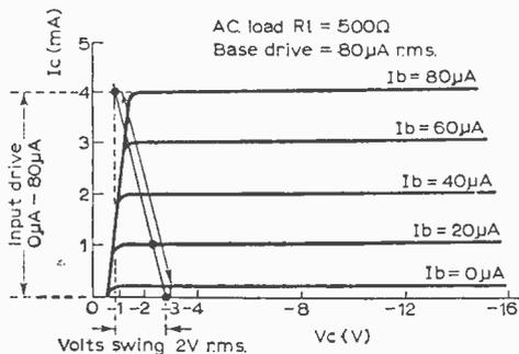
Fig. 1: Increasing the base drive current causes distortion on the upward swing, due to the "knee" of the characteristic.
