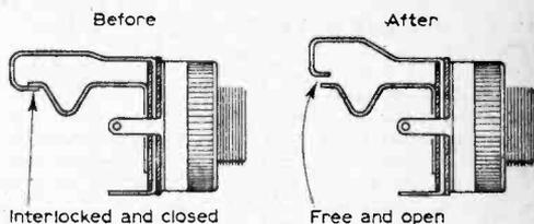
Fig. 4: The earpiece socket before and after modification.
