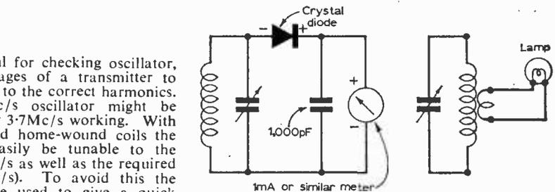
Fig. 2: Two absorption meter circuits including some form of indicator.
