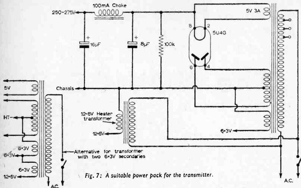
Fig. 7: A suitable power pack for the transmitter.
