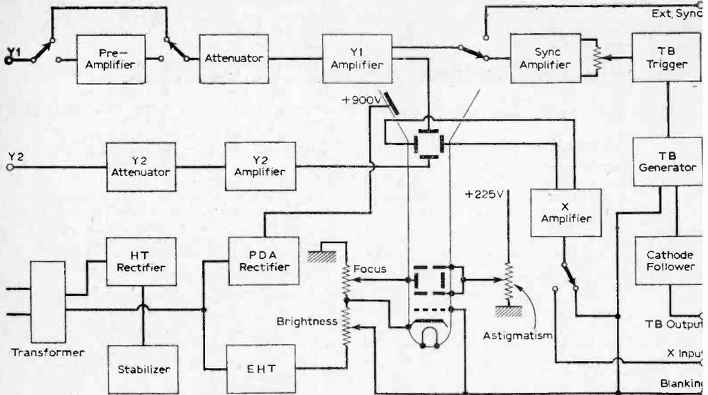
Fig. 6: Block diagram of the Cossor 1091, double-beam oscilloscope.
