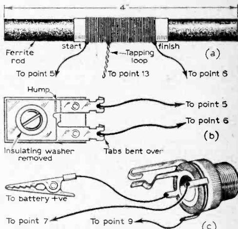
Fig. 5: Showing connections from (a) the aerial, (b) the tuning capacitor and (c) the earpiece socket.
