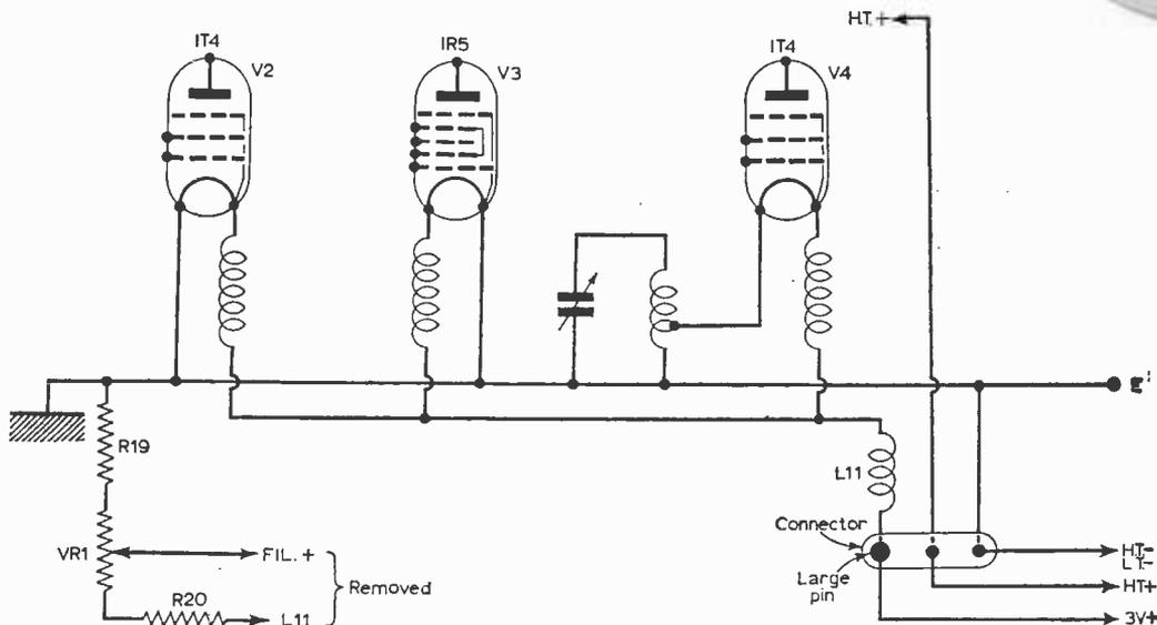
Fig. 5: The crystal calibrator No. 10 power supply circuit.
