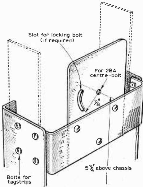
Fig. 4: Construction of the bridge mount for British tubes.
