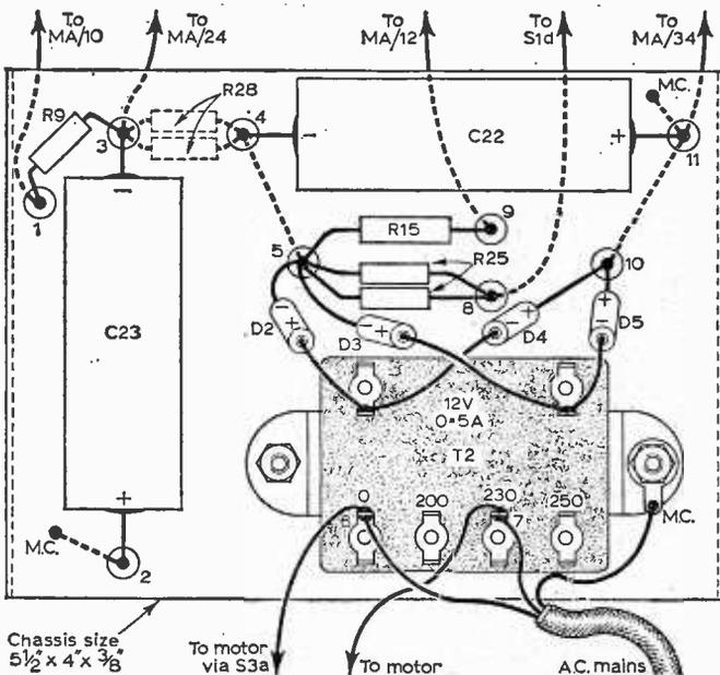
Fig. 9: The layout and wiring of the suggested power unit.
