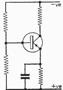
Fig. 2: Base bias voltage derived from potentiometer.
