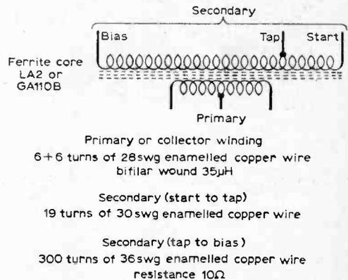
Fig. 12: The erase oscillator transformer, T3.
