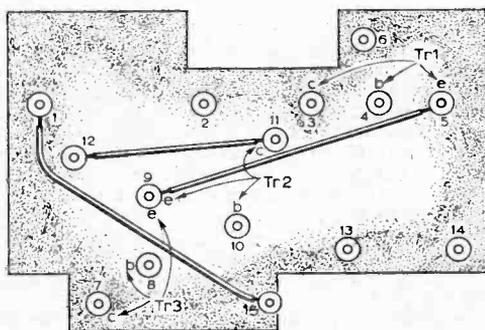
Fig. 3: The positions of the connecting wires and transistor base details.
