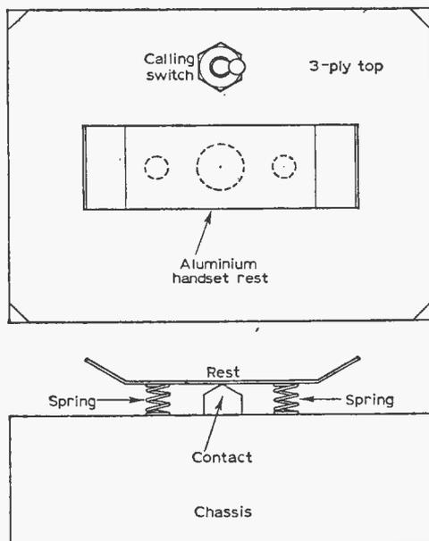
Fig. 2: Construction details of the telephone rest.
