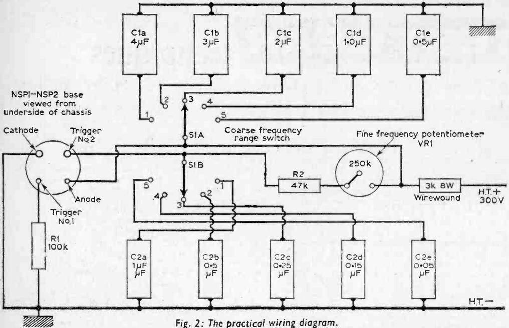
Fig. 2: The practical wiring diagram.
