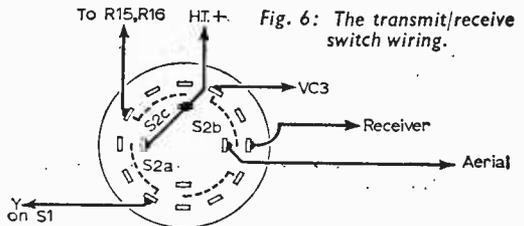
Fig. 6: The transmit/receive switch wiring.
