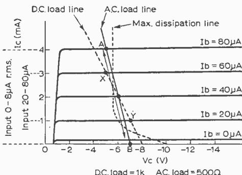
Fig. 2: Supply raised to 8V resulting in movement of load-line to the right, away from the "knee".
