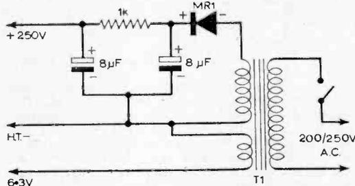
Fig. 4: A power pack for the crystal marker.
