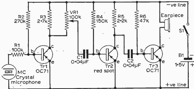
Fig. 1: The circuit of the amplifier.
