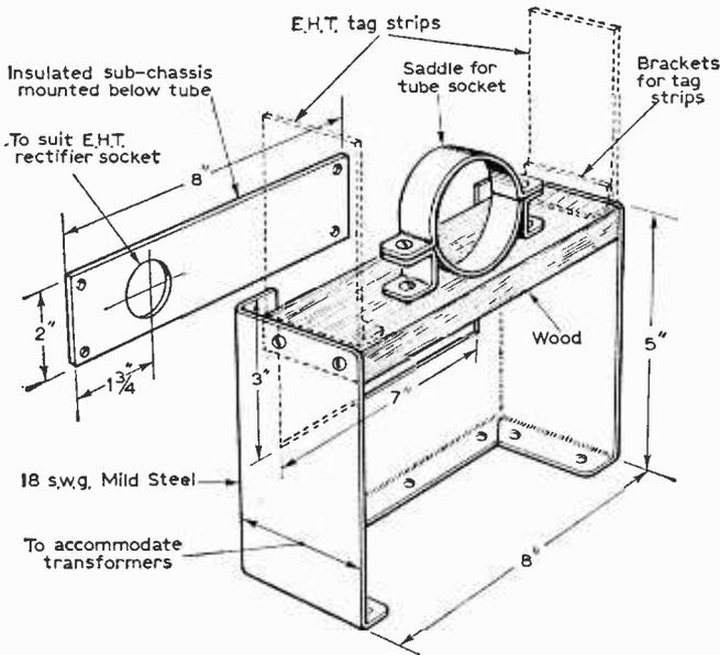
Fig. 3: Bridge assembly for American type tubes.
