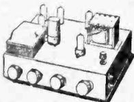
Hi Fi 15 watts. Valves ECC83, ECC83, ECF82, EL84, EL84, EZ81. Four jack inputs. Six controls: two volume, bass, treble, tremolo speed, depth. Remote
