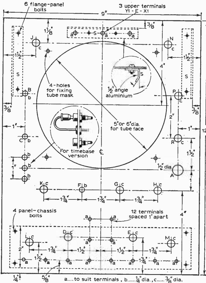
Fig. 1: Drilling details of the front panel.
