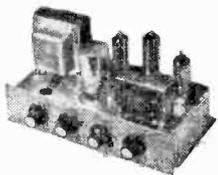
A small versatile 3-4 watts Gram Amplifier suitable for Crystal Pick-up or Radio Tuner, ideally suited for a small domestic installation. Output Imp. 3 ohms, volume control, treble control, bass control and middle control. Valve line-up: EL24, EF86, E750.
