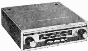
**HIGH PERFORMANCE CAR RADIO, CR-1.** Superb LW/MW entertainment, wherever you drive. For 12V pos. or neg. earth systems. Tastefully styled to match any car colour scheme. Many special features. Send for details. Can be built for a total price Kit (less spkr) £12.17.0 incl. P.T. (6 x 4 LS £1.4.5 extra)
