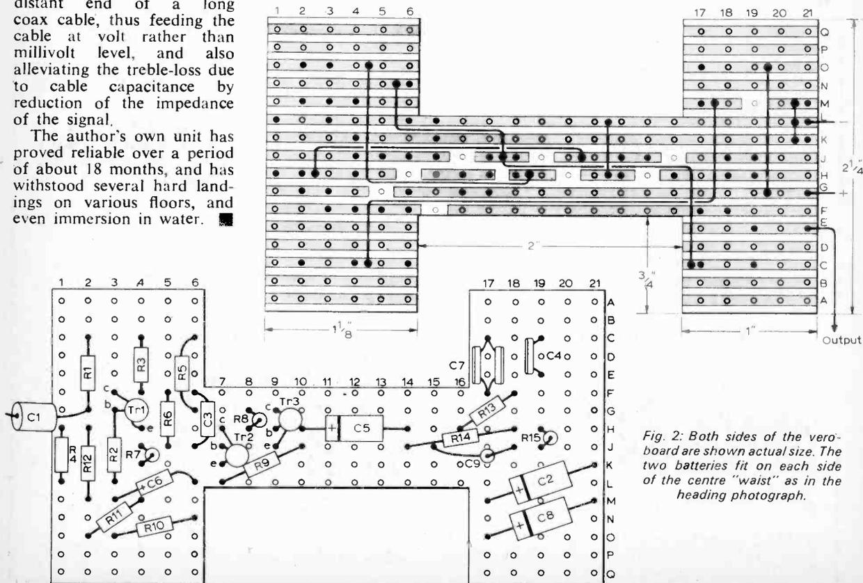
Fig. 2: Both sides of the veroboard are shown actual size. The two batteries fit on each side of the centre "waist" as in the heading photograph.
