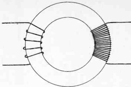
Fig. 4. Toroidal transformer.
