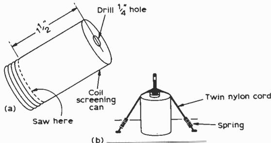
Fig. 7a: Screening can modifications; 7b: Mounting method
