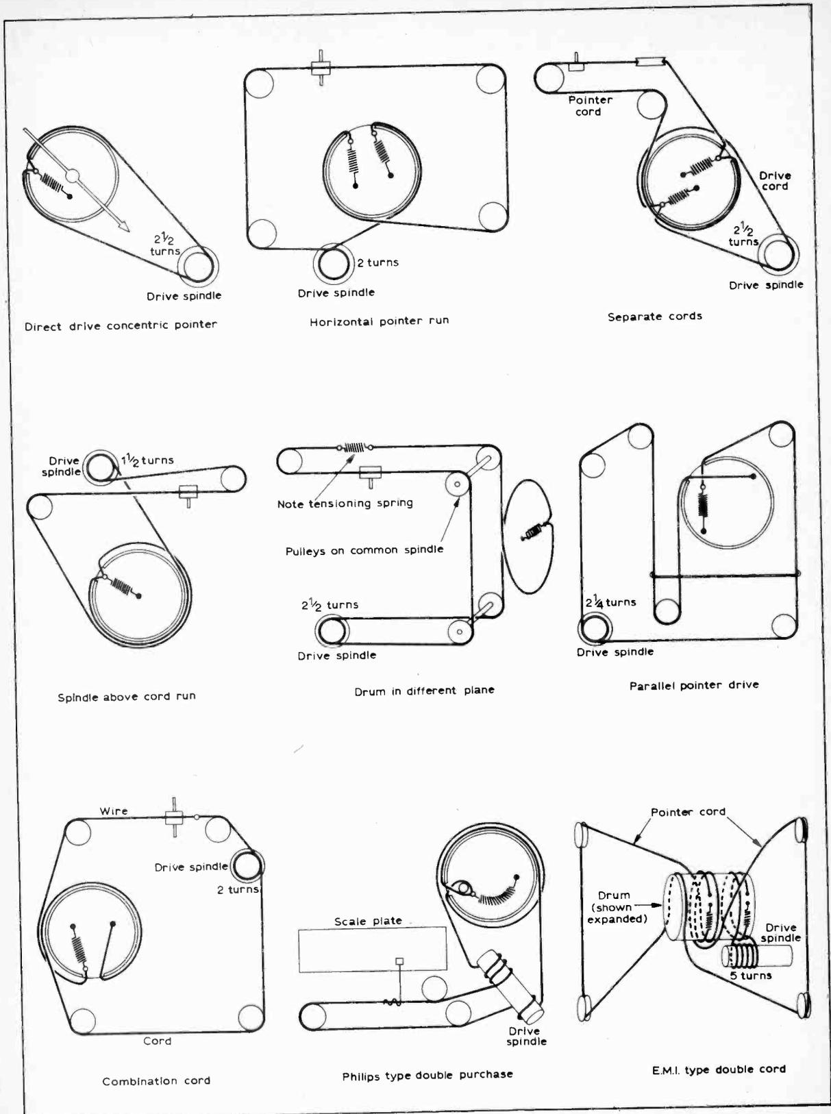
Fig. 11: Collection of cord drive systems from popular receivers, old and new. Note the importance of correct number of turns around spindles, drums, etc., and relative direction of cord run to main gang.
