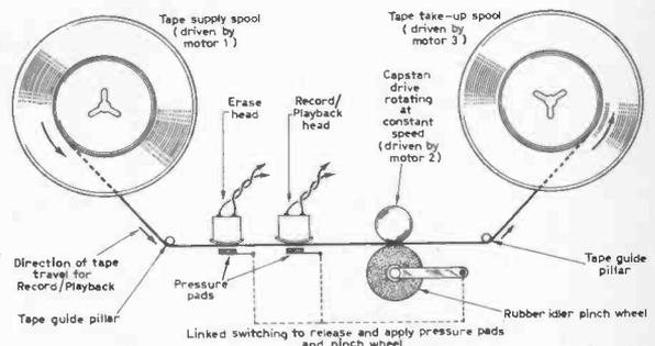
Fig. 9: The arrangement of the feed and takeup spools, the heads and the pinch wheel on a three motor tape deck.
