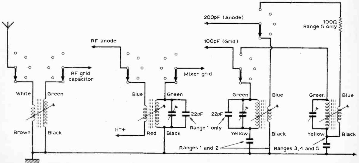
Fig. 5: The skeleton circuit of the r.f. and oscillator coils. Note the wiring differences in the oscillator section between ranges 1 and 2 and 3, 4 and 5.
