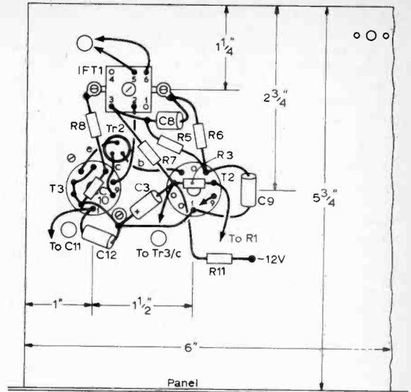
Fig. 5: Below chassis layout and wiring with dimensions.
