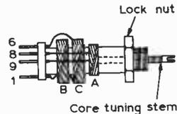
Fig. 6: Aerial and inter-stage coils.
