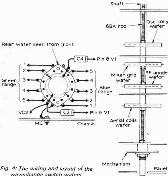
Fig. 4: The wiring and layout of the wavechange switch wafers.
