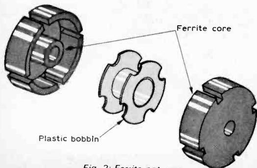
Fig. 2: Ferrite pot core.
