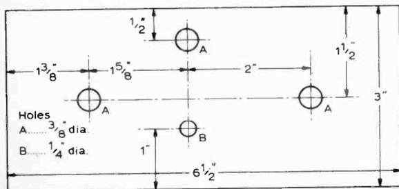
Fig. 3: Front panel dimensions.
