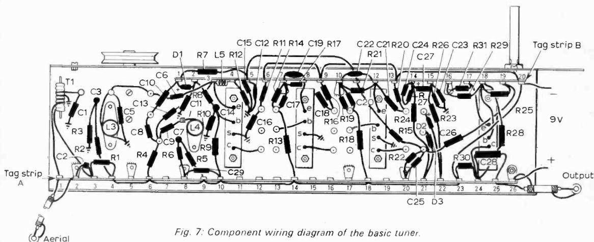
Fig. 7: Component wiring diagram of the basic tuner.
