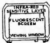
Famous war-time "cat's eye" used for seeing in the dark. This is an infra-red image converter cell with a silver caesium screen which lights up (like a cathode ray tube) when the electrons released by the infra-red strike it. A golden opportunity for some interesting experiments. 7/6 each, post 2/6. Data will be supplied with cells, if requested.
