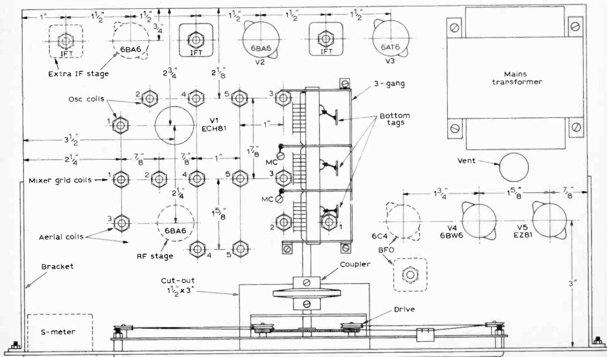
Fig. 2: The layout and details of the chassis viewed from the top.
