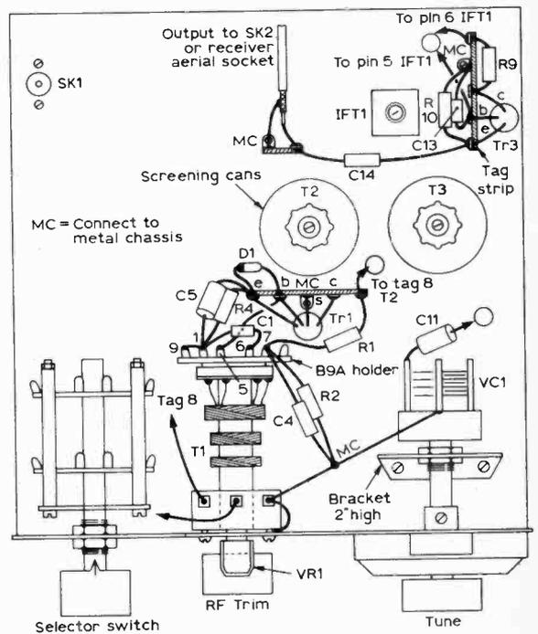
Fig. 4: Above-chassis layout and wiring details.
