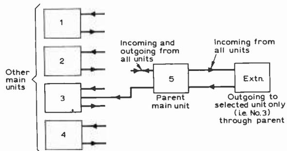
Fig. 11: Block diagram showing connection of auto-extension.
