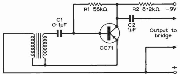
Fig. 4: A simple 800Hz audio oscillator suitable for driving a bridge.
