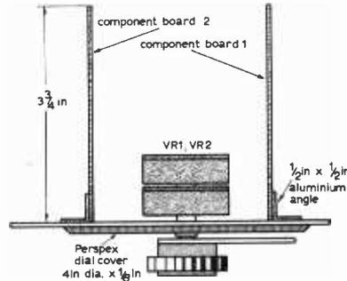
Fig. 4: The two transistor and component boards are attached to the front panel as shown on left. Details of the Perspex dial cover are also shown.
