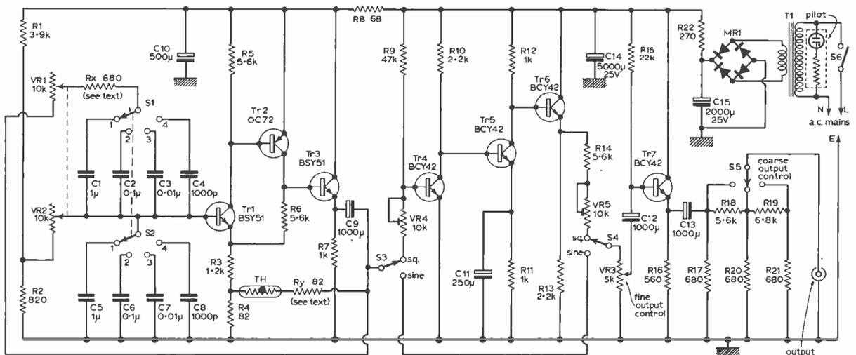
Fig. 1: Complete circuit of the sine and square wave audio signal generator.
