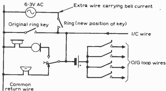
Fig. 13: Modification of circuit for a.c. ringing.
