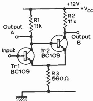
Fig. 5.1: A basic Schmitt trigger.
