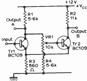
Fig. 5.2: A Schmitt trigger with variable setting.
