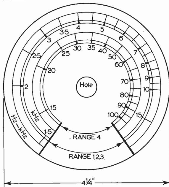
Fig. 9: The calibrated dial. This may be scaled-up to 4 $\frac{1}{4}$ in. diameter to give actual size.
