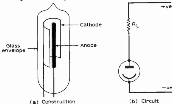
Fig. 16: The photoemissive valve.
