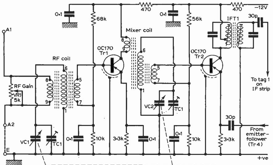
Fig. 4: Circuit for the front end using p-n-p transistors. Although providing better gain it suffers from cross modulation.
