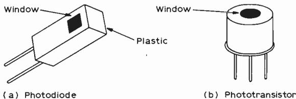
Fig. 18: Photodiode and phototransistor encapsulations.
