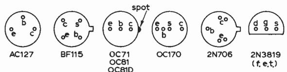
Fig. 5: The transistor connections for the types mentioned.
