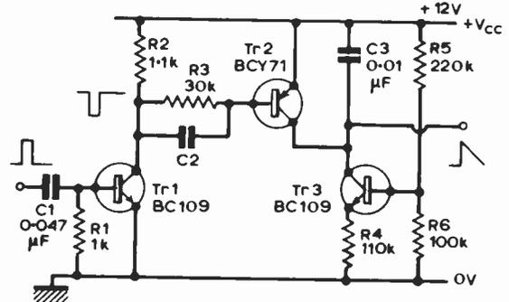
Fig. 5.5: A sawtooth or ramp generator.
