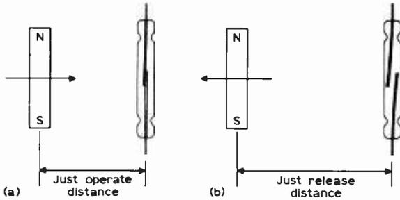
Fig. 10: Reed relay operation.
