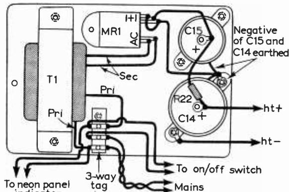
Fig. 6: Layout and wiring of the power supply.
