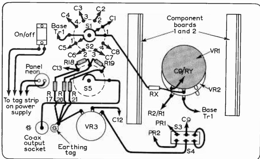
Fig. 5: Showing front panel wiring and layout.
