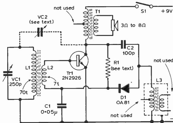
Fig. 1: The circuit of the one transistor radio.
