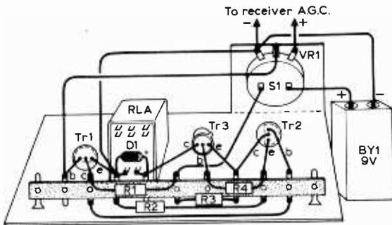
radio. Any reasonable signal will then cause the relay to de-energise but it is often useful to set VR1 so that only strong signals can break through the squelch. In this way, the crowded medium wave band can be "weeded out" so that it is reduced to a few strong local stations separated by silence.
