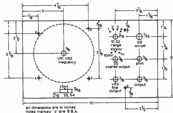
Fig. 2: Front panel dimensions and drilling details.
