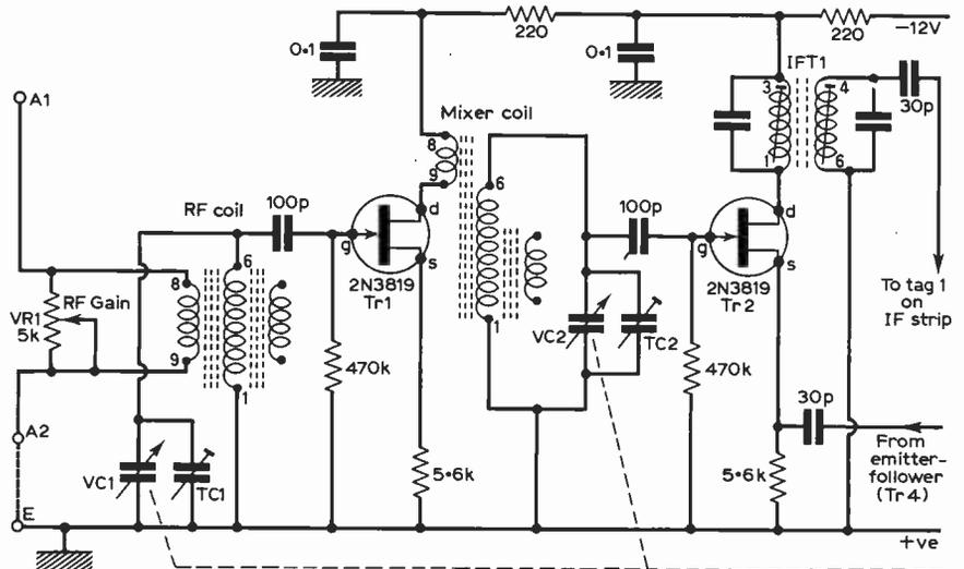
Fig. 3: An alternative front end using f.e.t.s. Although this circuit lacks gain, the use of 2N3829's should be an improvement.
