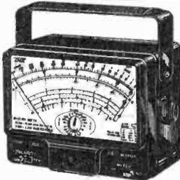
A highly reliable instrument using an entirely new range selection mechanism which permits the use of a really large meter in a more compact cabinet. The range selected is clearly indicated on the actual meter face facilitating instant identification without taking your eyes from the meter. High speed rotary range selection knob; also features polarity reversal switch, shielded meter movement with overload protection circuit; Special uA and mA measurement ranges.
