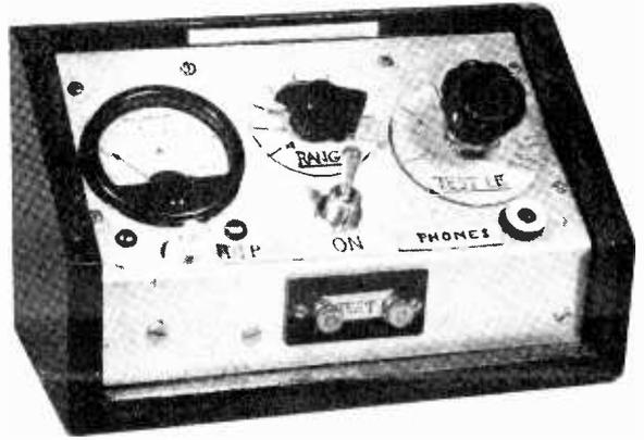
Hz indicated by headphones across R2. The current should be approximately 1mA. Headphones could be used directly to the bridge after this oscillator circuit, but some amplification enables a meter to be used, as already explained.
