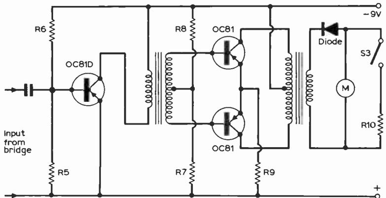
Fig. 5: A push-pull amplifier, detector and meter.
