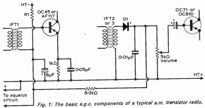
Fig. 1: The basic a.g.c. components of a typical a.m. transistor radio.
