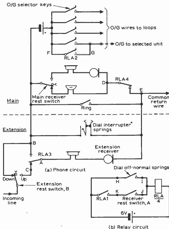
Fig. 12: Circuit diagram of auto-extension.
