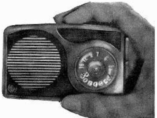
Apollo "6" will probably be bang up-to-date well into the seventies! It bristles with latest technical innovations. Six stage stable reflex N.P.N. and P.N.P. circuit consisting of 2 Radio Frequency stages, 1 Diode demodulation stage and 3 Audio Frequency stages. Uses latest Silicon Planar Epitaxial Epoxy transistors (similar to types used in America's Space
