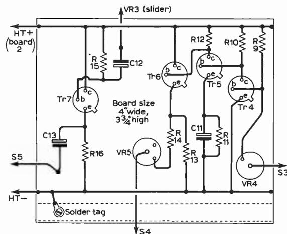
Fig. 8: Component board 1 layout and wiring (squaring circuit and emitter follower output stage).
