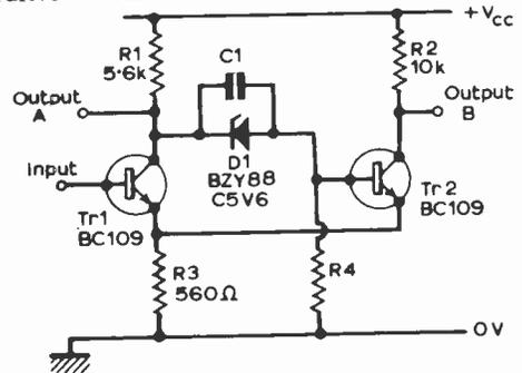
Fig. 5.3: Use of a Zener diode to set the triggering point.
