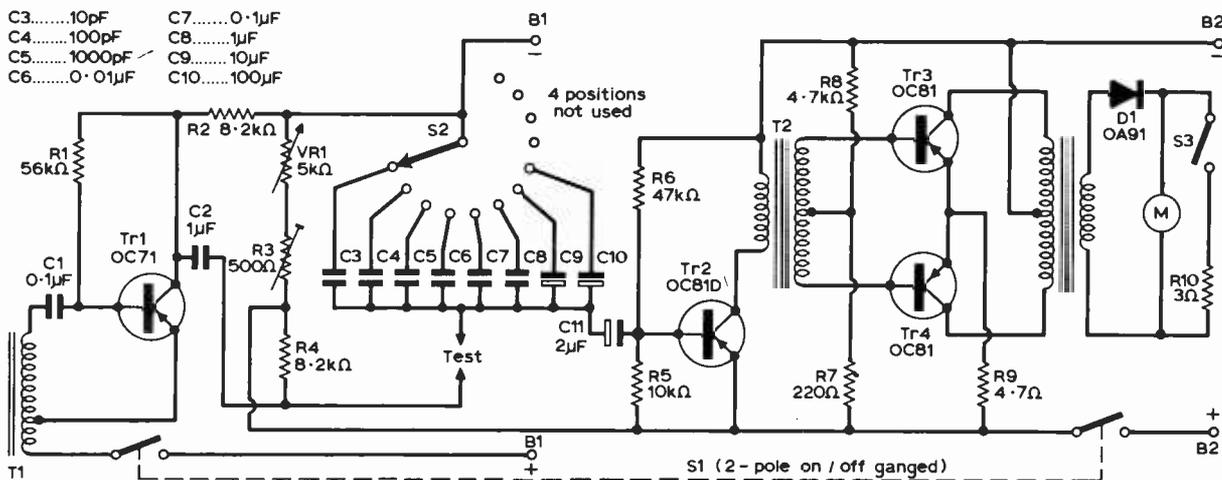
Fig. 6: The complete capacitance bridge capable of measuring from 1pF to 100μF. The accuracy of the bridge can be improved by decreasing the coverage of each range, revised component values being given in Table 1.
