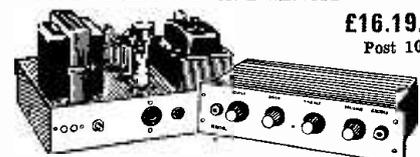
Main power amplifier and 2 valve pre-amplifier. Silver grey fascia panel. Volume, treble and bass controls. Function switch: Radio, Tape 1, Tape 2, Gram LF, Gram 78. Tape output socket. Valves: 2 x EL84, 3 x EF86, 1 x EC083, 1 x EZ81. Ultra linear Farnako output transformer. 20dB negative feedback. 10 watts r.m.s. mono. 3 or 15 ohm output. Brand New. Guaranteed.
