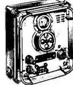
Small portable crystal controlled wavemeter. Size 7 x 7 1/4 x 4in. Frequency range 500 Kc/s-10 Mc/s (up to 30 Mc/s on harmonics). Calibrated dial. Power requirements 300V. D.C. 15mA at 12V D.C. 0.3A.
