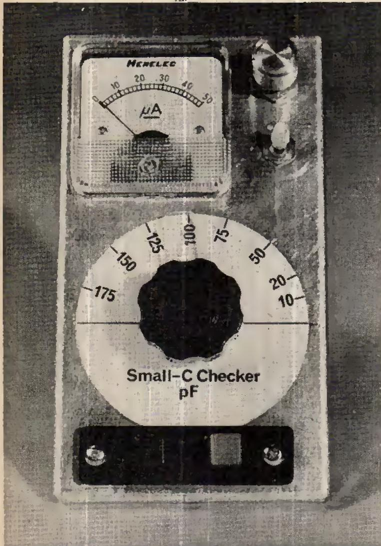
IN the course of time the average constructor accumulates quite a lot of odd small-value capacitors which eventually lose their markings and identity either by constant handling or by just being jostled around in the junk box. In any case they are then virtually useless and a positive menace and might just as well be thrown away. A 10pF capacitor used inadvertently with a tuned circuit instead of 100pF can cause an awful lot of trouble.
