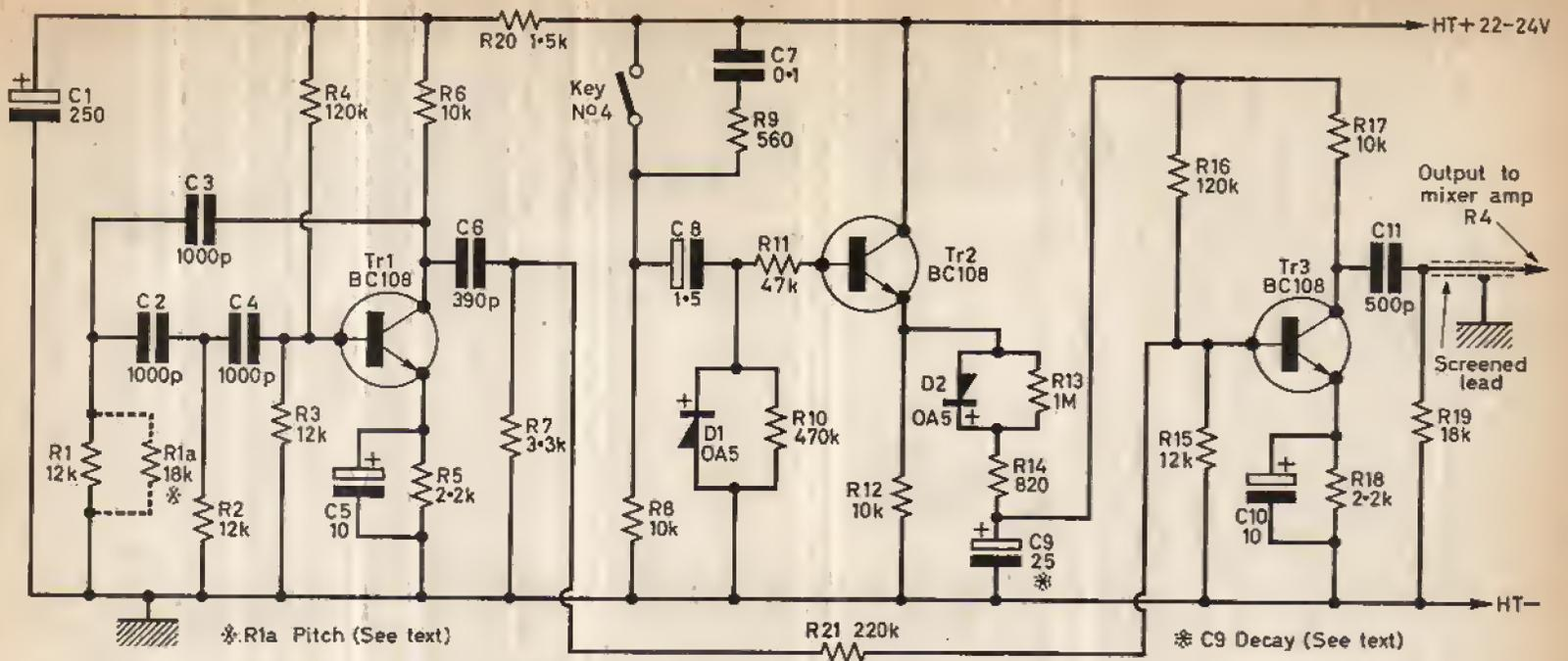
Fig. 11: The circuit of the triangle sound synthesiser.
