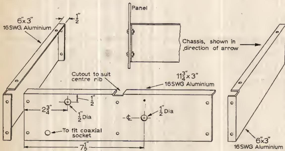
Fig. 7. Exploded view of chassis members. Note that panel extends below the bottom of the chassis, see Fig. 6. Part One. Since the rear member carries only the coaxial socket it can be left off until all wiring and constructional work is completed.
