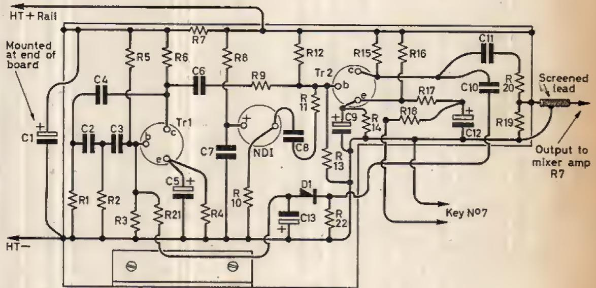
Fig. 18: The component layout for the circuit in Fig. 17, the train whistle synthesiser.
