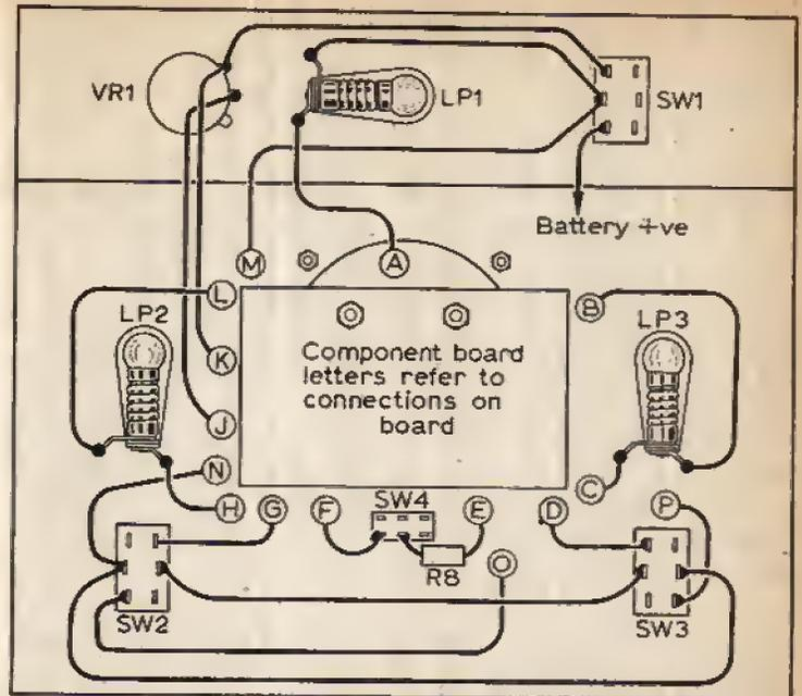
Fig. 4: The internal wiring of the reaction tester.
