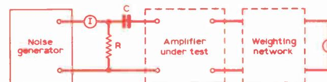
5% of specified source resistance and C must have an impedance at 1000Hz of less than 5% of the specified source resistance. Weighting network is inserted when the amplifier is intended to feed a sound reproducer. Results shall then be the 'weighted noise factor'. Weighting network reduces the effect of hum and any tendency to low-frequency cut-off due to the blocking capacitor.
