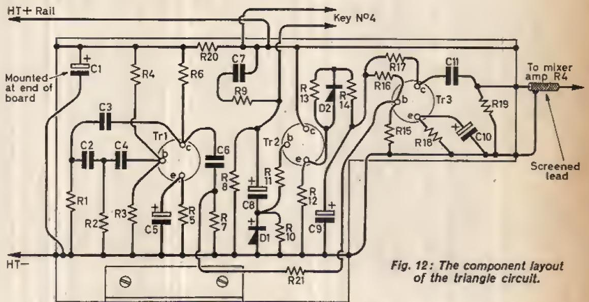
Fig. 12: The component layout of the triangle circuit.
