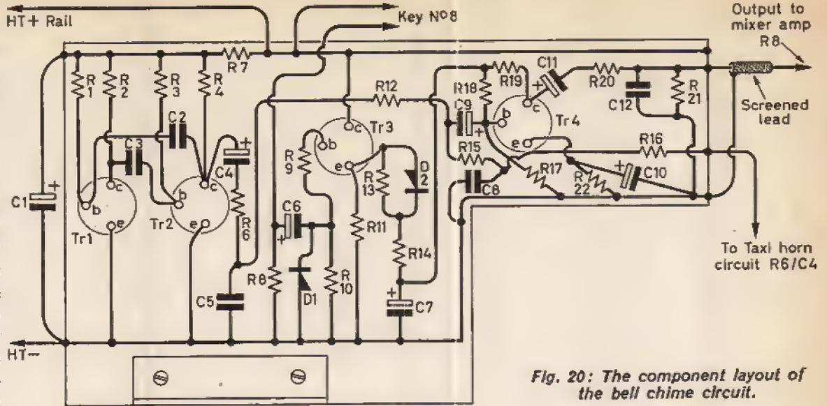
Fig. 20: The component layout of the bell chime circuit.
