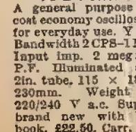
A general purpose low cost economy oscilloscope for everyday use. Y amp. Bandwidth 2 CFS-1MHz. Input imp. 2 meg Ω 25 P.F. Illuminated scale. 2 in. tube. 115 x 180 x 230mm. Weight 8lb. 220/240 V a.c. Supplied brand new with handbook. £22.50. Carr. 50p.
