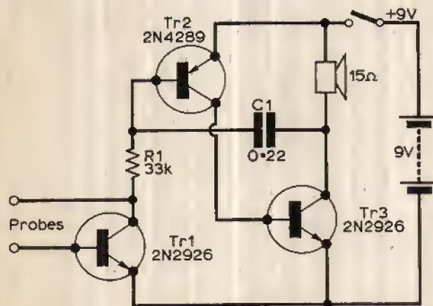
Fig. 1: The circuit of the Take 20 rain alarm
