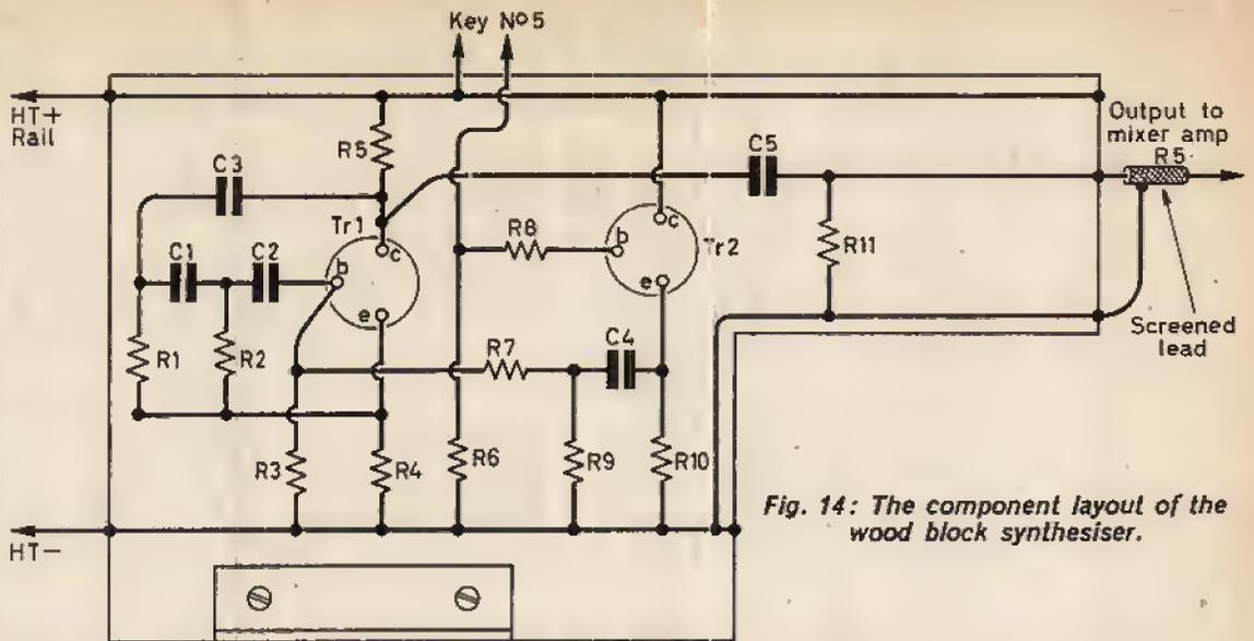
Fig. 14: The component layout of the wood block synthesiser.
