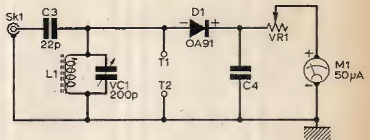
Fig. 1: Circuit of the Mk I capacitor checker.
