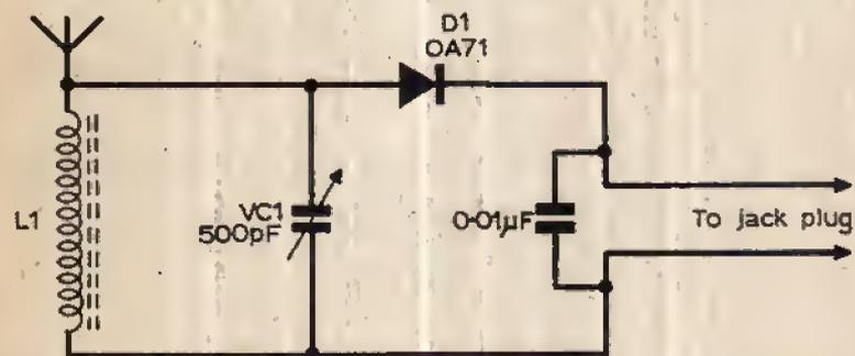
Fig. 1: Circuit of the crystal tuner. A resistor R1, 10kΩ, should be shown across the 0.01µF capacitor, but see text.
