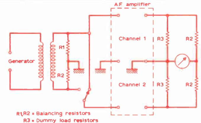
are made with input signals (a) in phase and (b) in opposition. The ratio of these two measurements is expressed, in dB, as a function of frequency.
