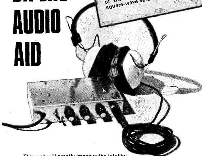
This unit will greatly improve the intelligibility of weak DX signals—by filtering the a.f. rather than working at r.f. It incorporates a highly efficient adjustable noise limiter together with an audio filter which will virtually eliminate heterodynes, whatever the strength.
