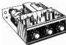
A superb solid state hi-fi amplifier. Brand new components throughout. 6 silicon transistors plus 2 power output transistors in push-pull. Full wave rectification. Output approx. 13 watts
