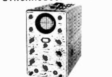
3-in tube fitted with telescopic viewing hood, giving bright display in full daylight. Sensitivity 10mV/mm (narrow band) to 30mV/mm (wide band). Bandwidth 10 c/s - 10 mc/s. Triggered sweep pre-set at 1.2-5.10-30-100-300-1000-3000 µsec per stroke. Free-running time base 20 c/s to 2000kc/s with built-in crystal calibrator providing timing marks at .05-2-1-5-20-100 µs.
