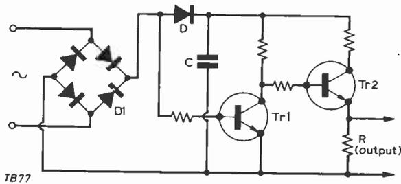
Fig. 4: Basic circuit which generates the pulses at the point of zero voltage crossing.
