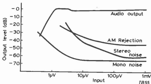
Fig. 1: Graphs comparing receiver performance with the input signal level.
