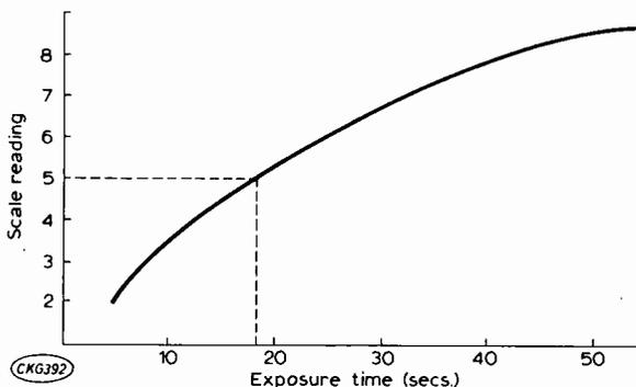
Fig. 4: A calibrated graph relating the knob markings of 1-10 to the time.
