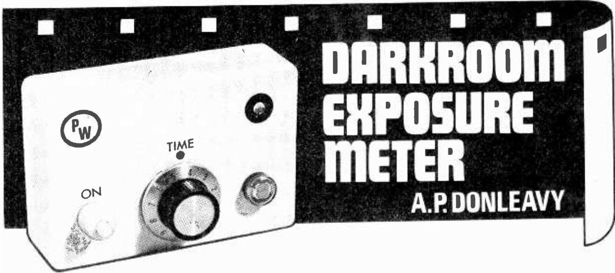
**T**HIS instrument was designed for use with a photographic enlarger, to determine the exposure required for any particular print. It is cheap to build and easy to use, with a range up to about 40 seconds.
