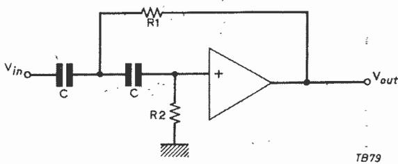
Fig. 7. Basic high pass filter. ▲
