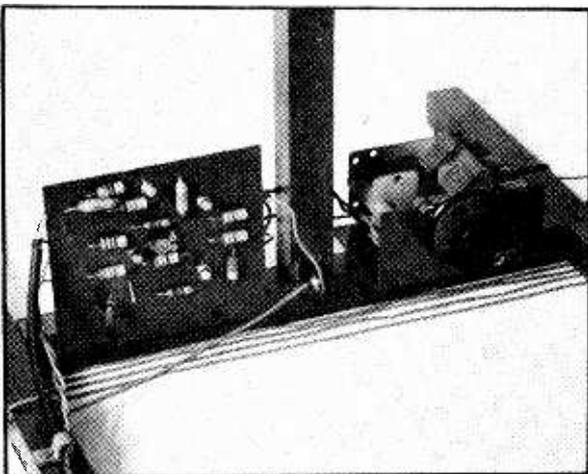
Close-up of the matching amplifier and loop tuning capacitor.
