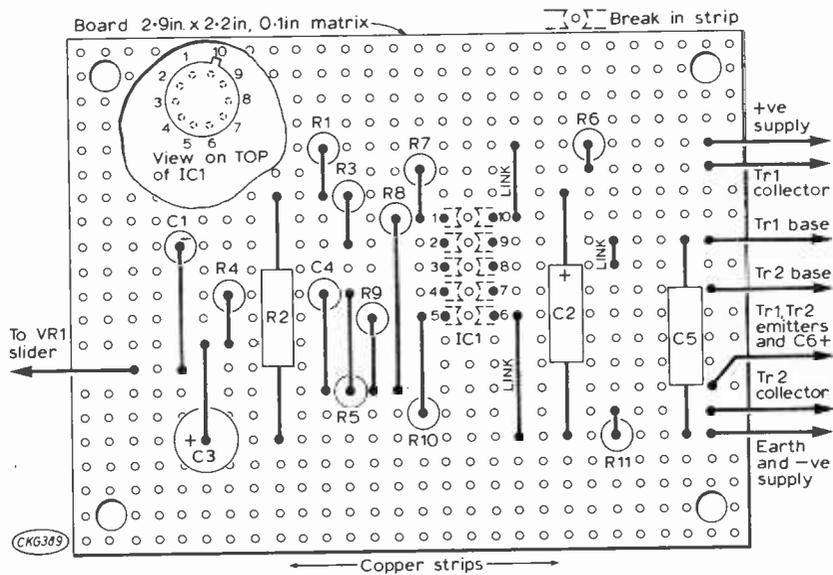
Fig. 3: Component layout on top of veroboard, the copper strips running horizontally underneath.
