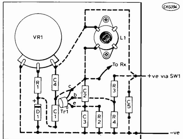
Fig. 2: A suggested component layout on drilled s.r.b.p. board.
