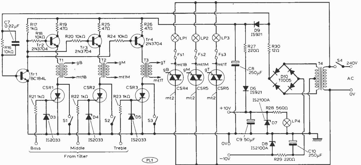
Fig. 12: Zero voltage switching control unit. The positive and negative 10V supply lines are the d.c. supplies to the filter unit (Fig. 9).
