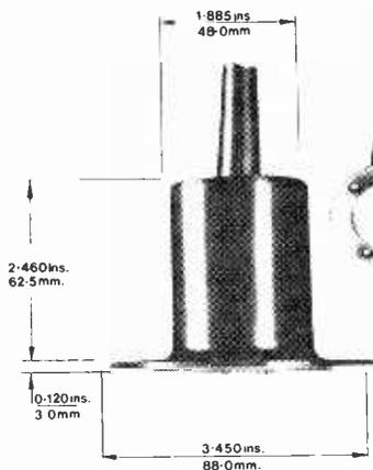
The electro-magnetic transducer for the magnetic log. As the boat moves along, a small e.m.f. is produced and sensed by two probes. This signal is then amplified and displayed in speed and distance units.
