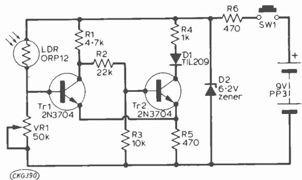
Fig. 1. The complete circuit which is basically a Schmitt trigger.
