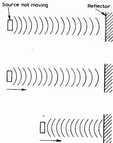
**Fig. 1: The Doppler Principle.**
