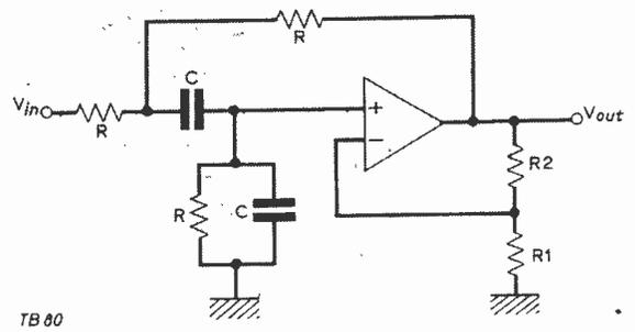
Fig. 8. Basic band pass filter.
