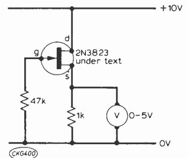
Fig. 6: (left) Complete circuit of the loop matching amplifier. Note that the 2N3823 transistor specified is preferable to the unscreened 2N3823E. Fig. 7: (above) is the circuit of the simple test set-up for checking the characteristics of the f.e.t.'s.
