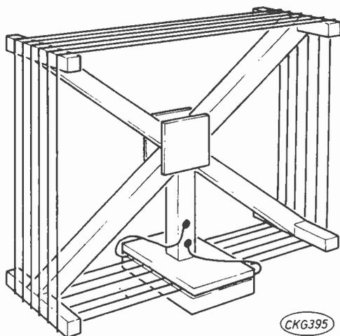
Fig. 1: Configuration of a typical m.w. loop aerial.
