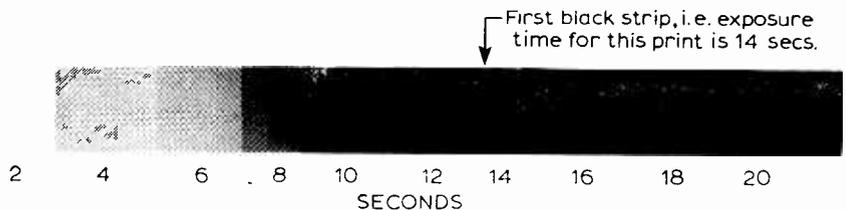
enlarger; all lights in the darkroom are put out except for the enlarger light; the instrument is placed on the easel, SW1 is depressed and VR1 is adjusted so that the diode light just goes from on to off. The reading on the scale is noted. (It is important that the scale reading is always taken from on-to-off since the off-to-on reading is different, owing to hysteresis in the Schmitt trigger.)
