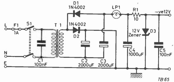
Fig. 11: Suggested power supply for the v.h.f. amplifiers.
