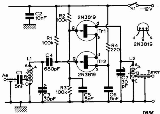
Fig. 2: Circuit of the amplifier using two f.e.t.'s.
