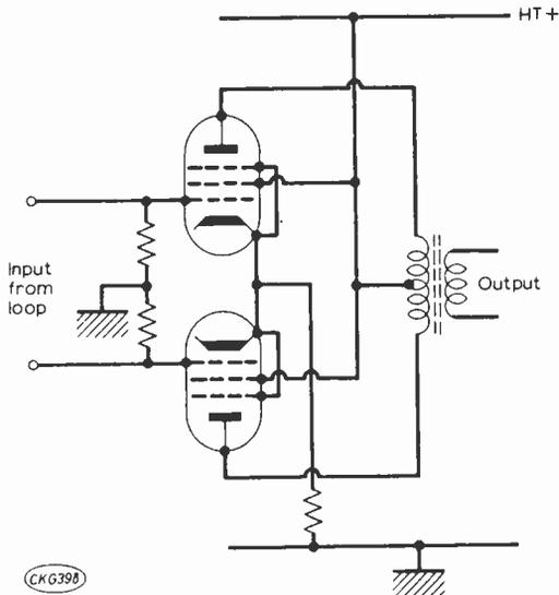
Fig. 5: Basic circuit of an early valve-type balanced input stage.
