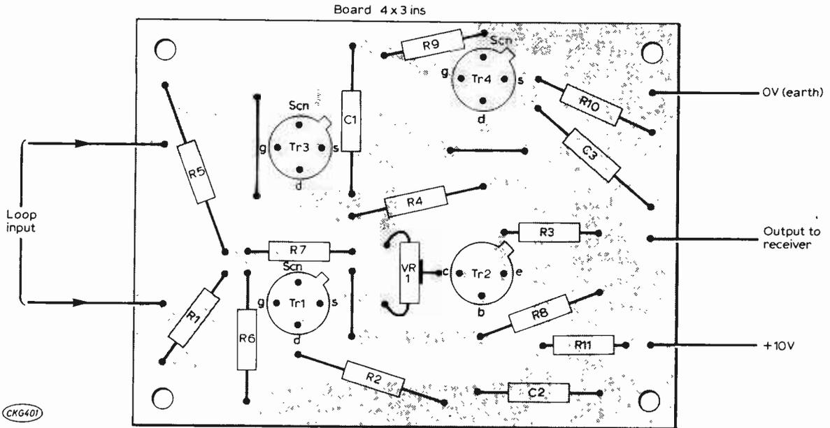
Fig. 8: Full size illustration of the printed circuit board, from the copper side. Small holes are drilled for component leads and the components mounted from the other side of the board.
