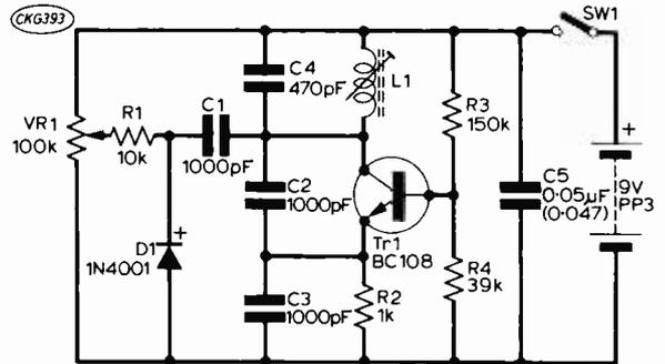
Fig. 1: The circuit - instead of using a conventional variable capacitor, D1 tunes the circuit
