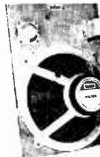
30-14,500 c.p.s. 12in. double cone, woofer and tweeter cone together with a BAKER ceramic magnet assembly having a flux density of 14,000 gauss and a total flux of 145,000 Maxwells. Bass resonance 40 c.p.s. Rated 20 watts. NOTE: 3 or 8 15 ohms must be stated.
