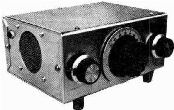
This view of the receiver shows the positioning of the internal loud-speaker and the socket for an external loudspeaker or headphones.
