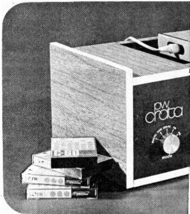
**T**HIS constructional feature describes a stereo-multiplex AM/FM tuner-amplifier providing 10 watts RMS output per channel into 8Ω loads with facilities for incorporating a cassette tape recorder. The integrated unit provides very good results which, although not to true high fidelity standards, will give satisfying listening for a moderate outlay.
