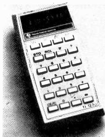
The European Calculator Division of Texas Instruments Ltd. has introduced a hand-held calculator specifically designed for secondary school students. It is designated TI-1270. The 4-function machine features a store and recall "scratch pad" memory and four keys recommended by maths educators for student use: reciprocal, square, square root and  $\pi$ .
