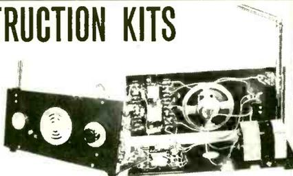
**ECK4** 7 Transistors, 6 tuneable wavebands, MW, LW, Trawler Band, 3 Short Wave Bands. Receiver Kit. With 5" x 3" Loudspeaker. Push/Pull output stage, Gain Control, and Rotary Switch. 7 Transistors and 4 Diodes. 6 section chrome-plated telescopic aerial. 8" Sensitive Ready Wound Ferrite Rod Aerial. Tuning Capacitor, Resistors, Capacitors, etc. Operates from a 9 Volt PP7 Battery (not supplied with kit). Complete kit of parts including construction plans. **£7.25**
