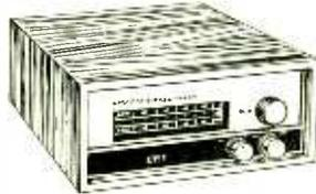
200/240V Mains operated Solid State F/M A/M Stereo Tuner. Covering M.W. A.M. 540-1605KHz VHF/FM 88-108MHz. Built-in Ferrite rod aerial for M.W. Full APC and AGC on AM and FM. Stereo Beacon Lamp Indicator. Built in Pre-amps with variable output voltage adjustable by pre-set control. Max. o/p Voltage 600mV RMS into 20K. Simulated Teak finish cabinet. Will match almost any amplifier. Size 8 1/2" w x 4 1/4" h x 9 1/4" d approx.
