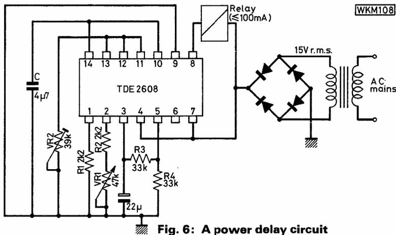
Fig. 6: A power delay circuit
