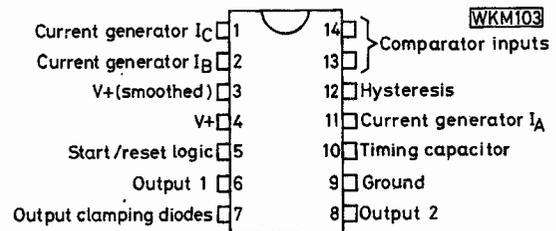
Fig. 1: The connections of the TDE 2608 device
