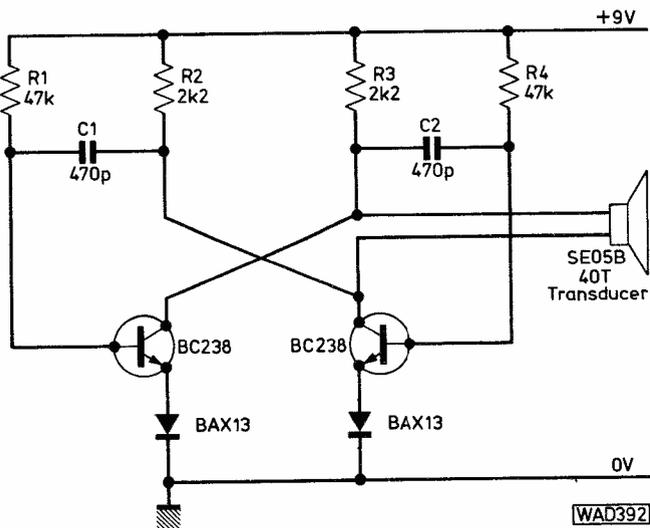
**Fig. 1: Discrete component circuit to provide an ultrasonic signal**
