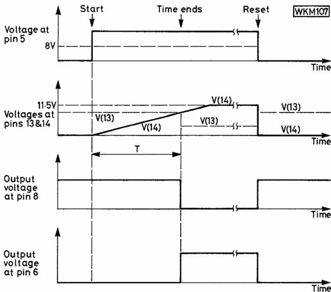
Fig. 5: TDE 2608 timer waveforms
