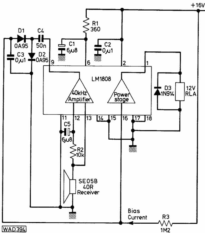
**Fig. 3: Receiver circuit using an LM1808 integrated circuit**
