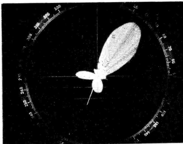
**Fig. 9: Pattern from an experimental high-gain beam aerial, which shows that side lobes are too large and therefore the design is not acceptable**
