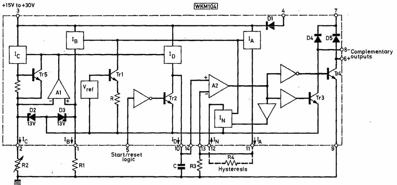
Fig. 2: The internal circuit of the TDE 2608 in block form
