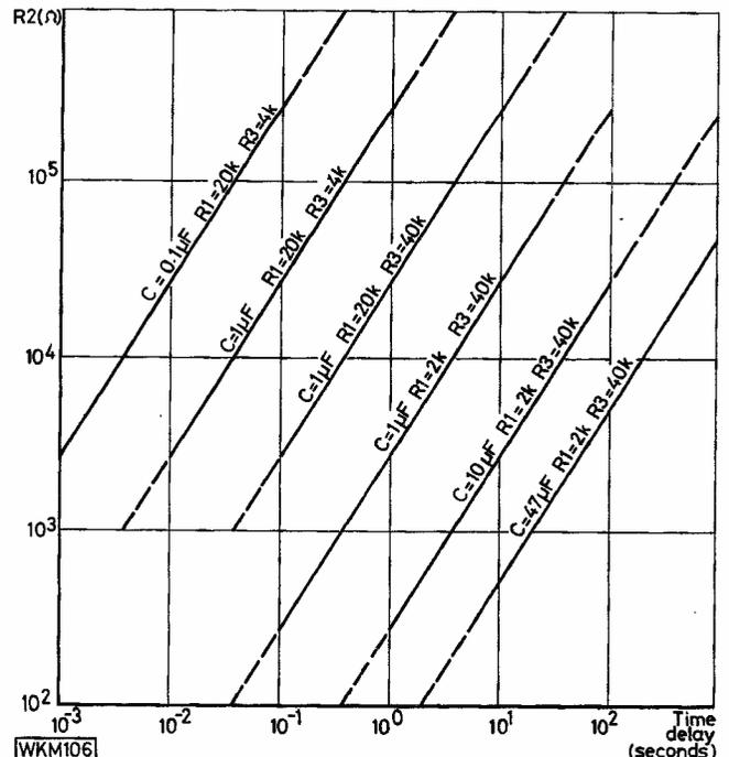
Fig. 4: Time delays available with various component values
