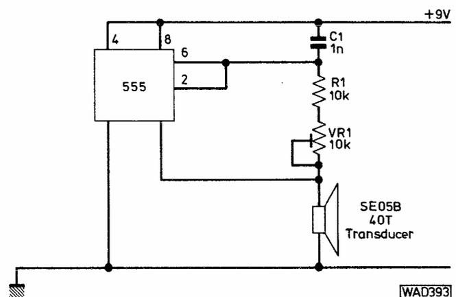
**Fig. 2: Ultrasonic generator circuit using a 555 timer**
