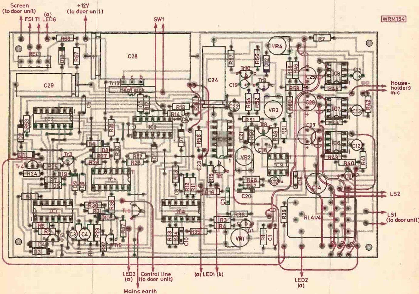
Printed circuit board details for the main unit. The copper track pattern is shown full-size at the top with the component placement drawing underneath. Note: C17 is a non-polarised ceramic capacitor
