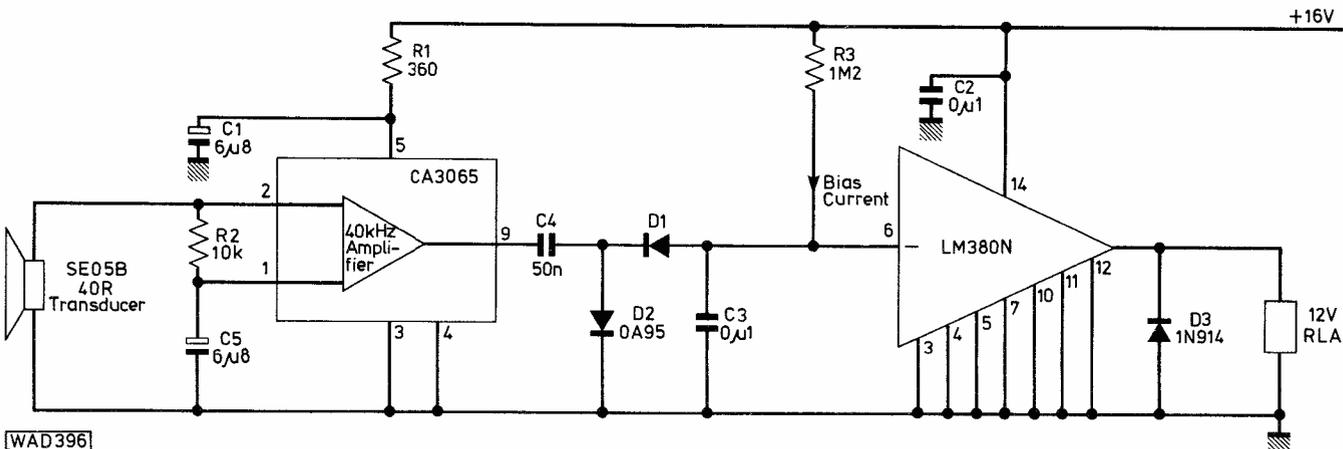
**Fig. 4: Circuit using the 3065 and LM380 integrated circuits**
