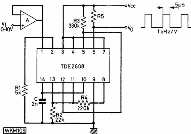
Fig. 8: A voltage-to-frequency converter
