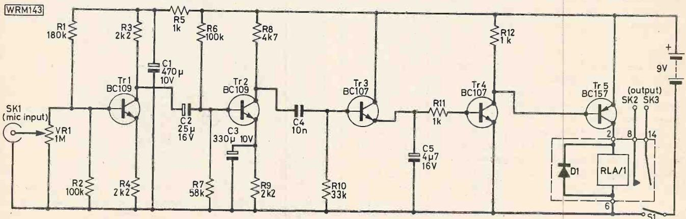
**Fig. 1: Circuit diagram of the telephone bell repeater amplifier. D1 is fitted inside the relay specified but if a different relay is used then a diode (1N4148) must be fitted across the coil**
