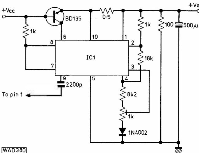
**Fig. 16: Alternative biasing circuit offering a lower internal resistance. IC1 is a 723 voltage regulator. The diode should be mounted in the same manner as shown for D2 in Figs. 5 and 7 (Part 1). All resistors can be ½ watt rating**
