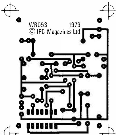
Fig. 2: The printed circuit board copper track pattern is shown full size
