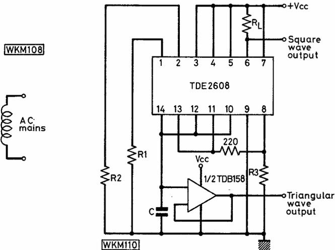
Fig. 7: A waveform generator circuit
