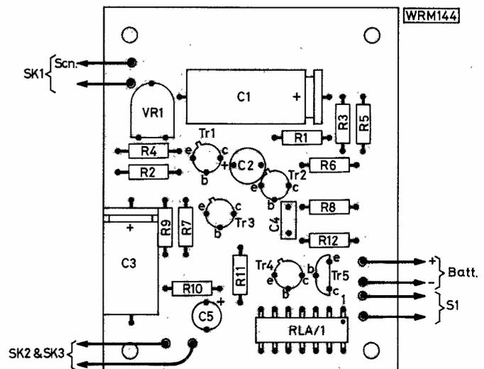
Fig. 3: The component placement for the p.c.b.
