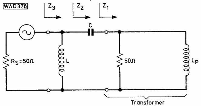
Fig. 14: Low-frequency compensation circuit for input transformer inductance
