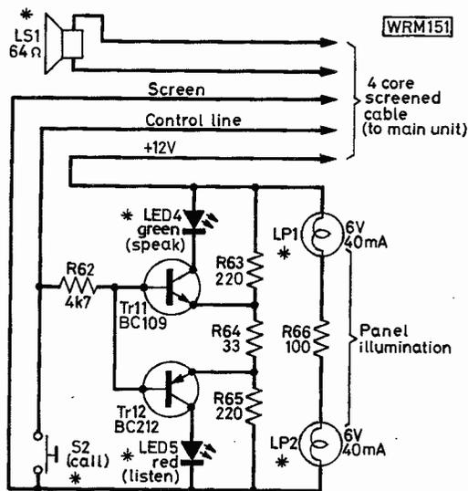
Fig. 2: Circuit of door unit. Starred items are mounted on front panel
