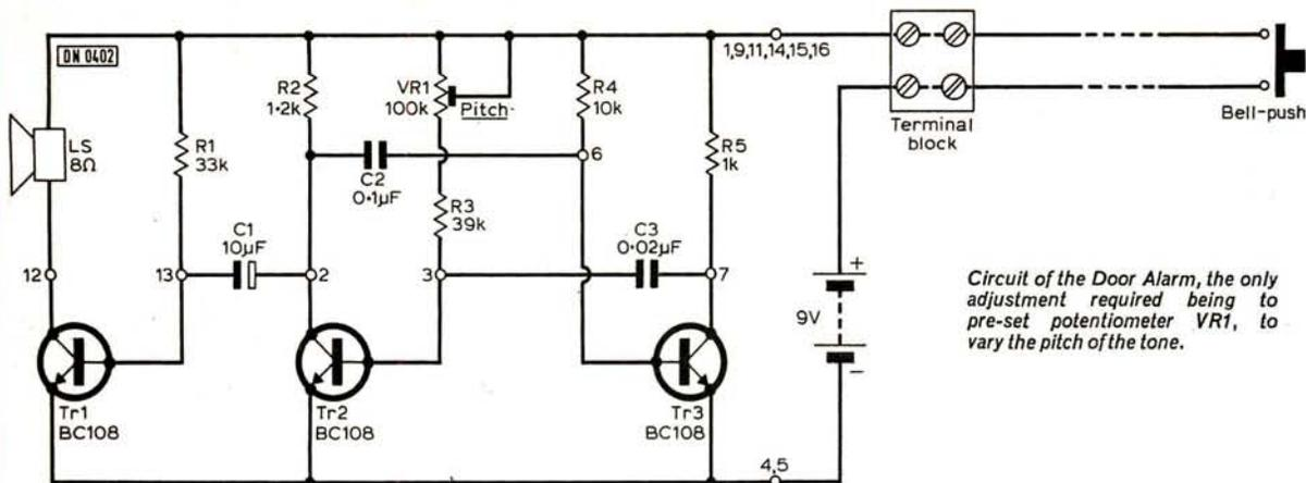
*Circuit of the Door Alarm, the only adjustment required being to pre-set potentiometer VR1, to vary the pitch of the tone.*
