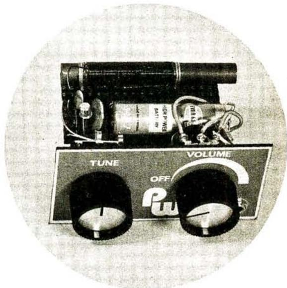
A single silicon integrated circuit provides several functions not normally available in TRF receivers.
