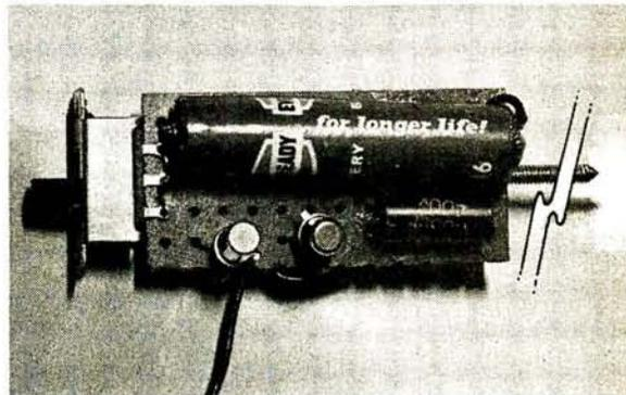
The board is fixed to one set of contacts on the switch by wire passing through holes in the board. The other set of contacts is used for the on-off switch.
