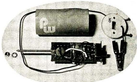
The finished Signal Injector ready to be fitted into its case, preferably a plastic one.
