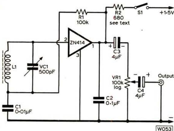
The tuner circuit using the ZN414 IC. Under no circumstances must the supply voltage exceed 1.5V.
