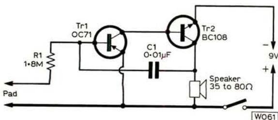
The circuit of the Rain Warning Bleeper could hardly be simpler. Altering the values of R1 and/or C1 will change the tone.
