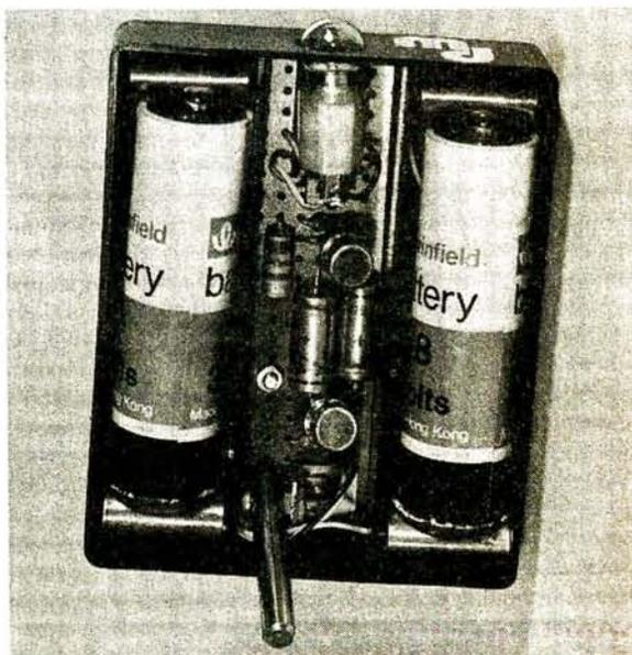
Inside the Memo Reminder showing the board in the centre and the gravity switch at the bottom, lifted up from its normal position to show the fixed contact.
