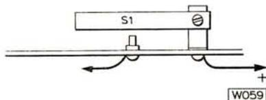
Details of the gravity switch and bracket.
