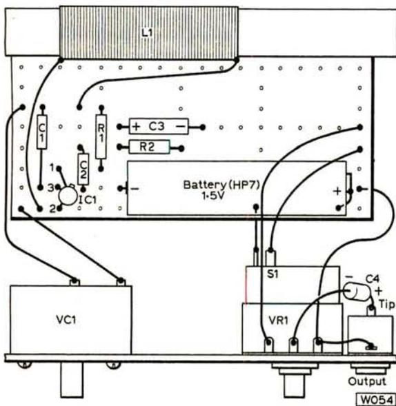
Plan view of the layout of components. The board is connected to VC1 and S1 by heavy copper wires.
