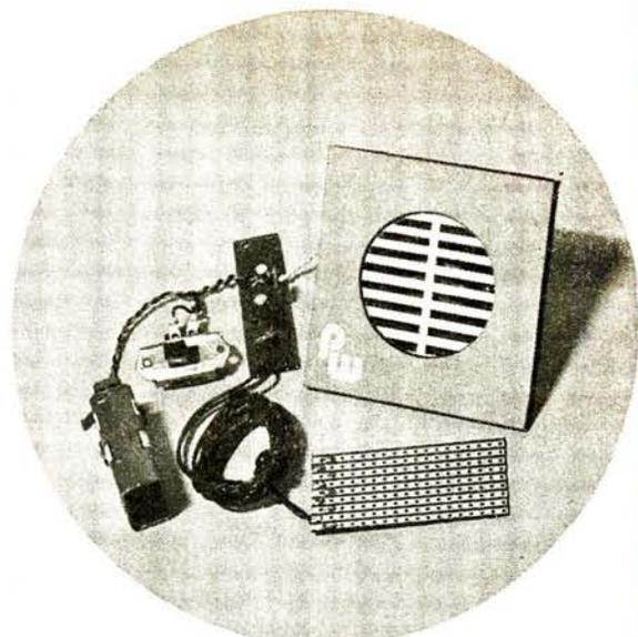
The speaker, circuit board, switch and battery can be fitted into any convenient sized box, leaving the pad to be placed outside in the open.
