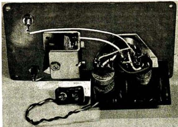
Rear view of the Booster showing circuit board fitted to the front panel via a metal bracket held under the wavechange switch.
