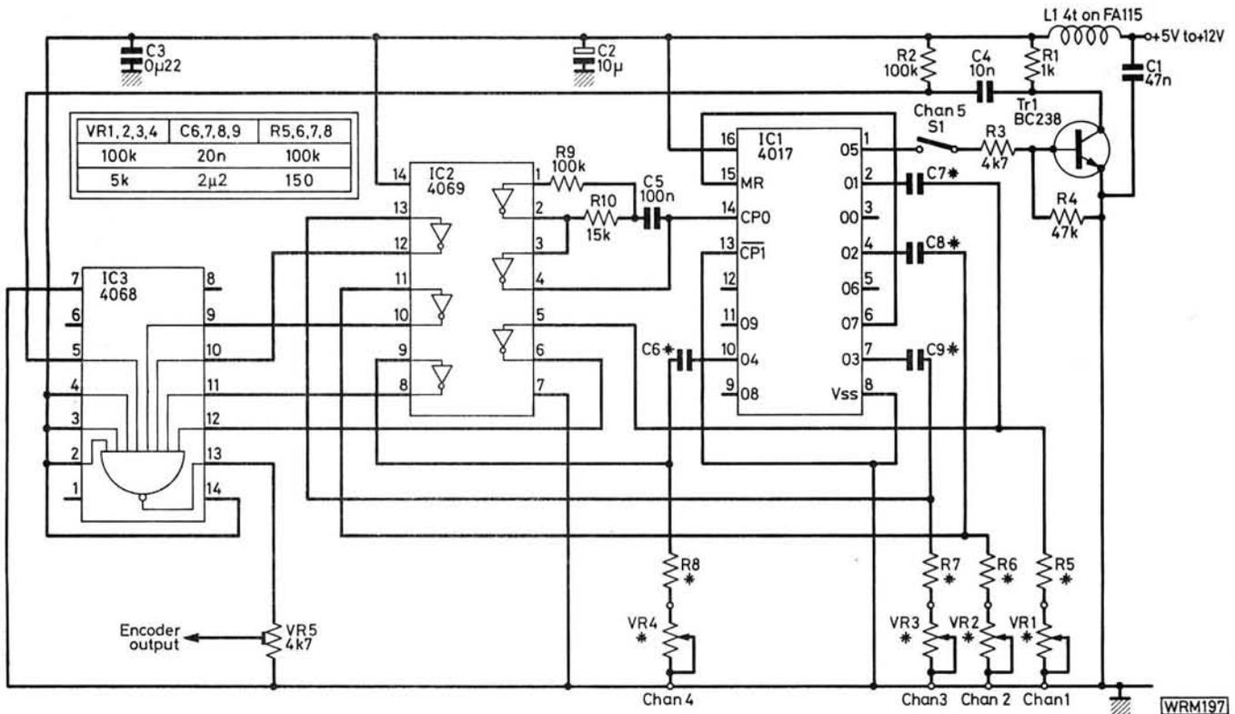
**Fig. 2: Circuit diagram of the encoder.** The components marked with an asterisk fix the timing periods and the values depend on the total track resistance of the control stick potentiometers. For 5kΩ pots the capacitors should be 2·2μF tantalums with the positive lead connected to the appropriate pin of IC1.
