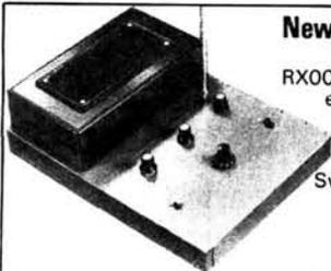
8 Transistors and Four Diodes. Multiband AM Receiver.
