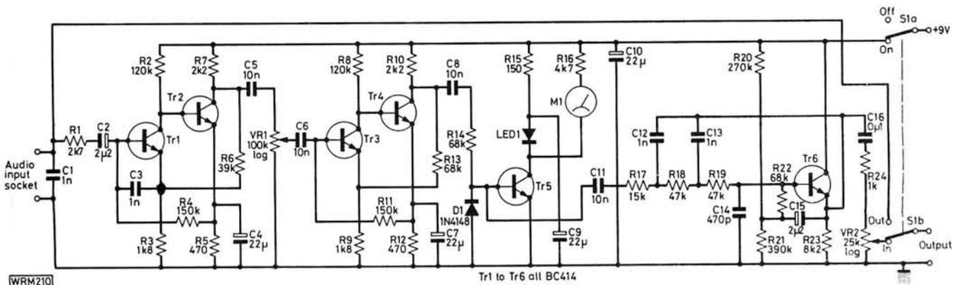
Fig. 6: Circuit diagram. Components R16, M1 and LED1 are not p.c.b. mounted
