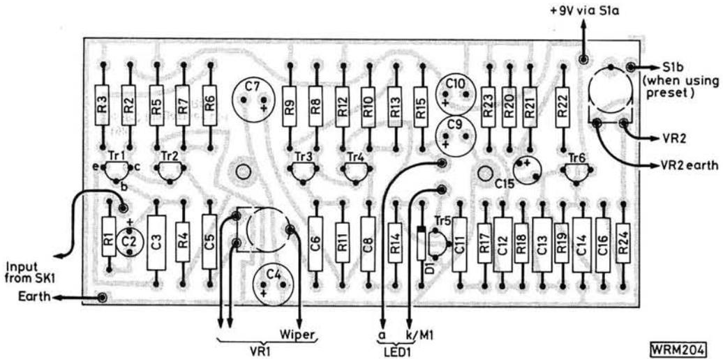
Fig. 9: Copper pattern and component layout shown full size
