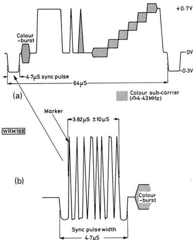
**Fig. 1(a): Test signal without sound-in-syncs. Fig 1(b) shows how the encoded audio is inserted into the sync pulse**
