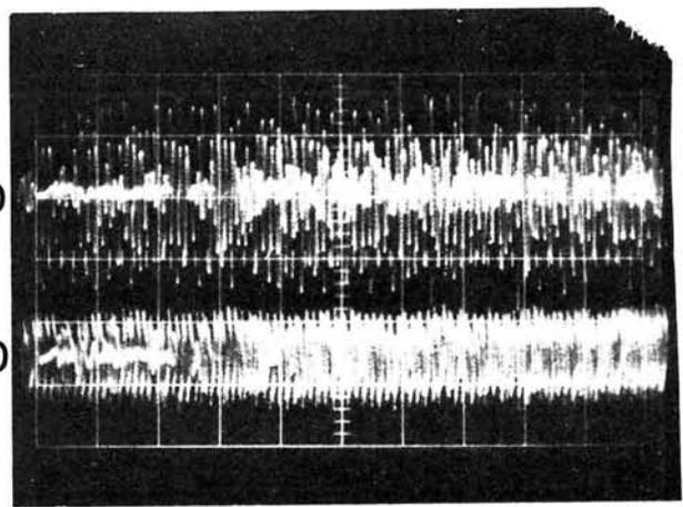
Fig. 5: The word "Hello" before and after processing
