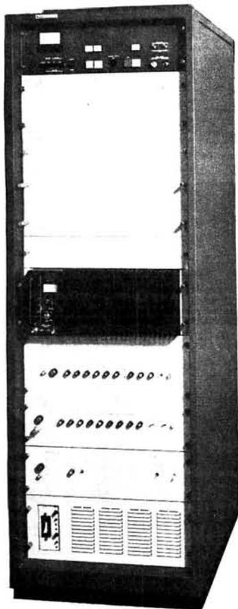
**Marconi B7303 u.h.f. transmitter of the type used throughout the system**
