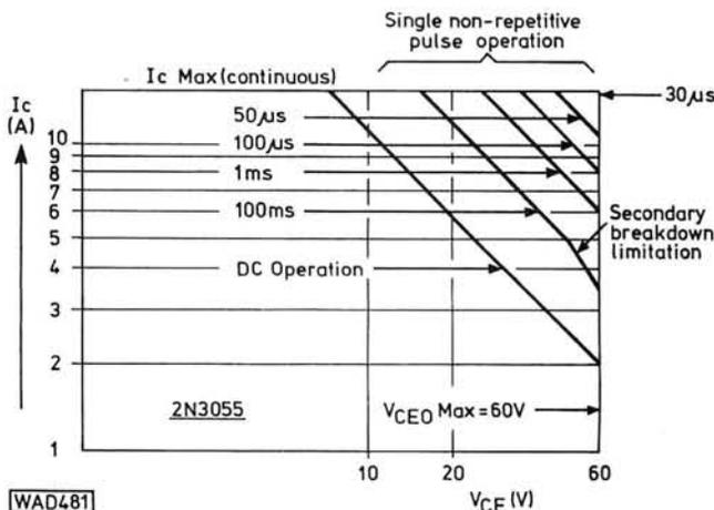
**Fig. 2: A power transistor Safe Operating Area (SOA) graph**
