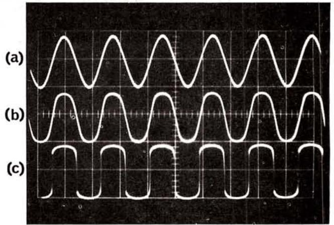
**Fig. 3: Traces (a), (b) and (c) show the output wave shape of the basic circuit for inputs 0dB, 6dB and 20dB above the diode conduction point**
