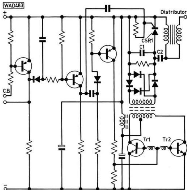
Fig. 4: Circuit of an electronic ignition system, with critical components identified
