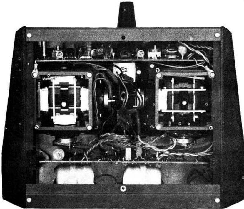
The photograph on the left shows the completed transmitter with both boards and the control sticks correctly positioned. The transmitter board is shown at the top and the encoder board below the case
