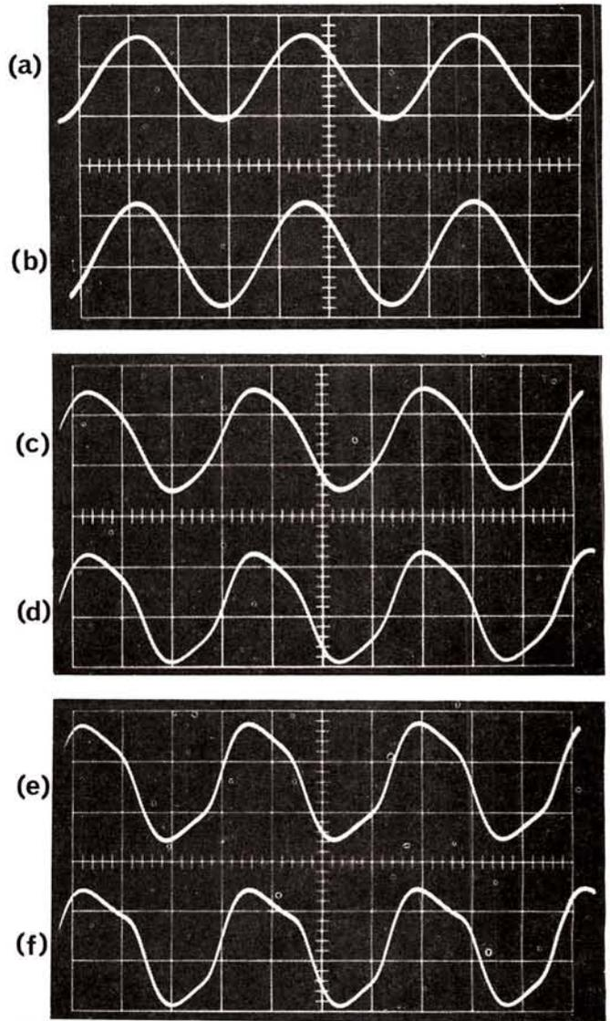
**Fig. 4: The traces show the processor output for increasing input signal voltage. (a) and (b) are the outputs below and at the limiting threshold, (c)–(f) are those for inputs 6dB, 12dB, 18dB and 24dB above it**
