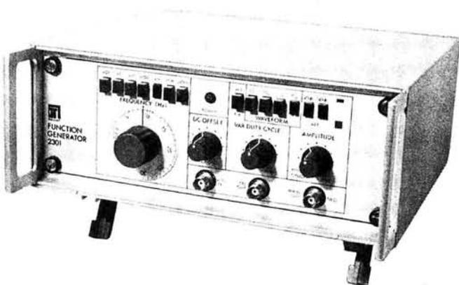
A function generator is of much more use in a lab than a simple sine wave oscillator. The ability to produce a wide variety of different shaped waveforms gives the user the means with which to test the correct functioning of most of the projects he is likely to build.
