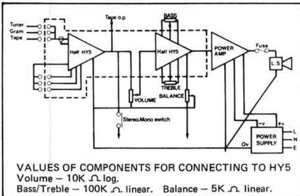
The HY5 pre-amp is compatible with all I.L.P. amplifiers and P.S.U.'s. It is contained within a single pack 50 x 40 x 15 mm, and provides multi-function equalisation for Magnetic/Ceramic/Tuner/Mic and Aux (Tape) inputs, all with high overload margins. Active tone control circuits; 500 mV out. Distortion at 1KHz - 0.01%. Special strips are provided for connecting external pots and switching systems as required. Two HY5's connect easily in stereo. With easy to follow instructions.
