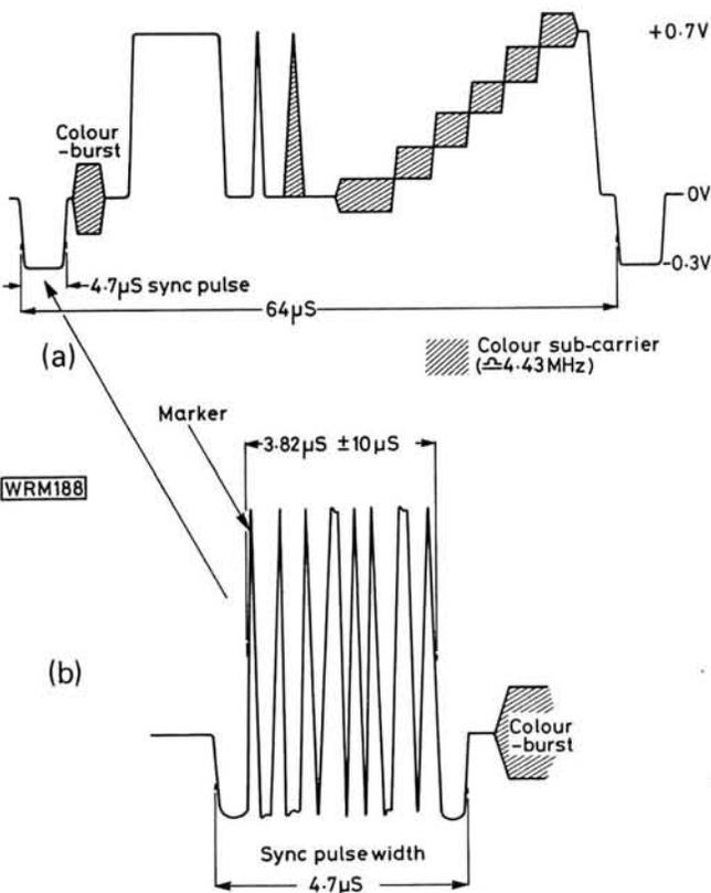
**Fig. 1(a): Test signal without sound-in-syncs. Fig 1(b) shows how the encoded audio is inserted into the sync pulse**
