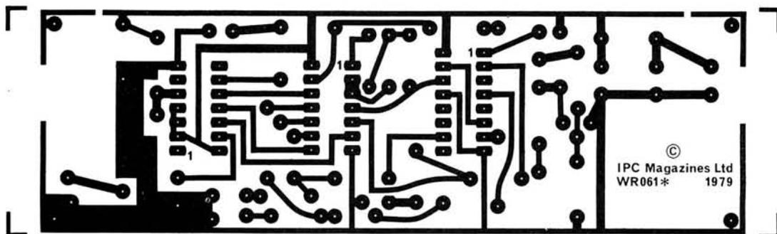
Fig. 4 (top): The component placement for the encoder board. Fig. 5 (above): The copper track layout is shown full size
