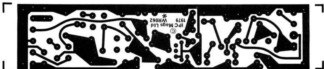
Figs. 6 and 7: The component placement and copper track plan for the transmitter board shown here full size. Care must be taken to ensure that the lead-outs of Tr1 and Tr2 are checked carefully
