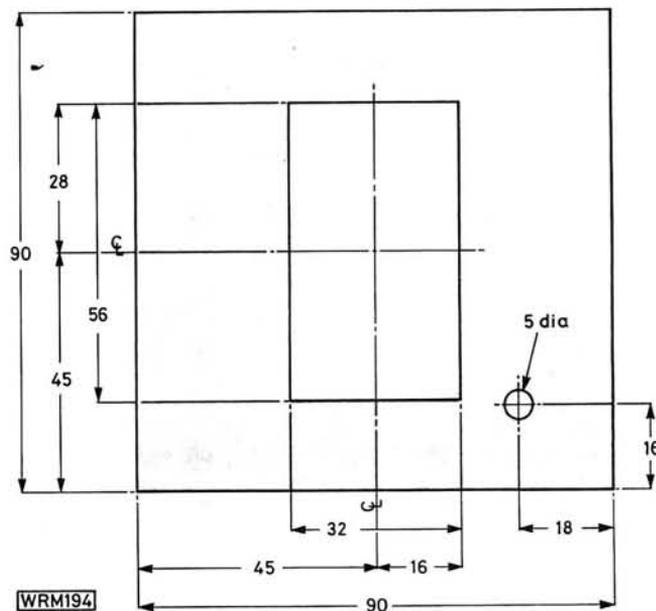
Fig. 3: Front panel details
