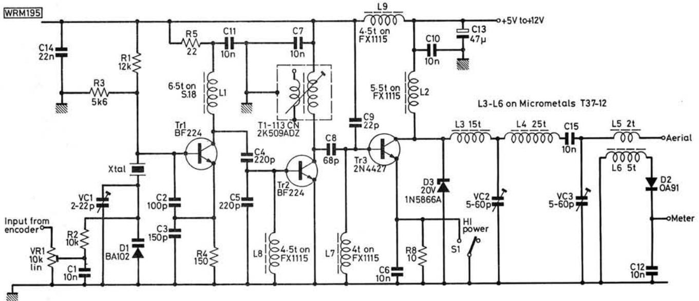
**Fig. 3: Circuit diagram of the transmitter.** The value of R8 can be changed to alter the power output of the transmitter when S1 is switched to Low Power
