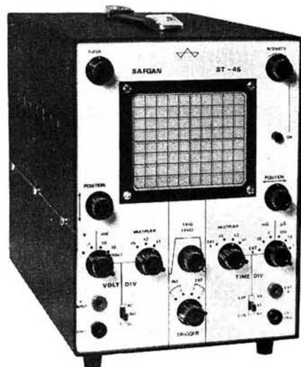
Brimar Group and has a very bright, clear, well defined display even at the fastest sweep speed of 200ns/div. The instrument is mains powered with a power consumption of approx. 10 watts. Overall dimensions of the black p.v.c. finished aluminium case are 216 x 165 x 280mm deep and the cream-white front panel is silk-screened with black annotations.
