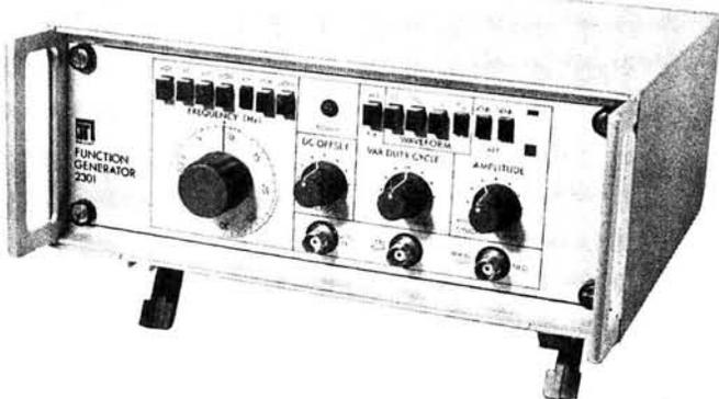
A function generator is of much more use in a lab than a simple sine wave oscillator. The ability to produce a wide variety of different shaped waveforms gives the user the means with which to test the correct functioning of most of the projects he is likely to build.
