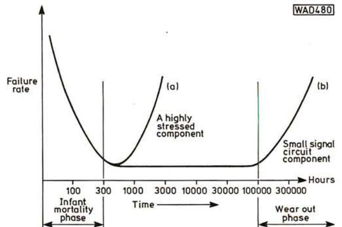
Fig. 1: General pattern of component failure, the familiar "bathtub" curve
