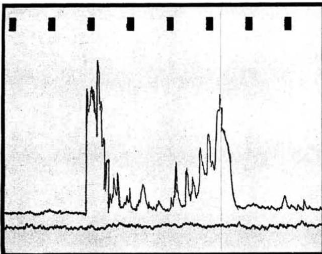
Fig. 1: Four minute solar burst recorded by the author at 146MHz at midday on October 5. The lower trace is the normal receiver noise level recorded on the 4th
