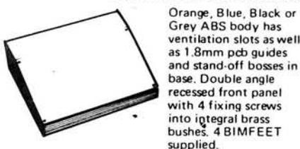
Orange, Blue, Black or Grey ABS body has ventilation slots as well as 1.8mm pcb guides and stand-off bosses in base. Double angle recessed front panel with 4 fixing screws into integral brass bushes. 4 BIMFEET supplied.
