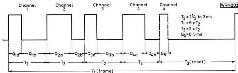
**Fig. 1: The encoder output waveform showing the fixed frame length, the reset or synchronising pulse and the individual channel pulses (Q1a etc). Channel 5 is non-proportional and is intended for such applications as retracting under-carriages**
