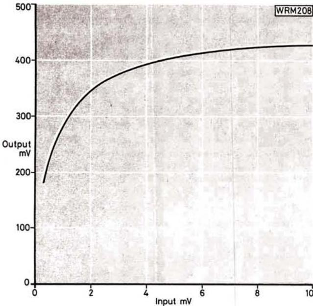
**Fig. 2: The output signal voltage is progressively limited as the input voltage is increased**
