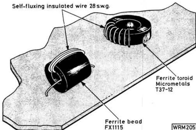
**Fig. 9: The correct method of winding the r.f. chokes and toroidal inductors**
