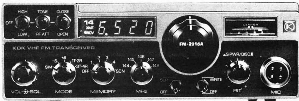
The KDK FM-2016E is a 12V DC two metre FM transceiver for mobile and base station use. It has been compactly designed with emphasis on maintenance and ease of use by using the latest CMOS IC digital PLL circuitry. Rx 144.000-148.995MHz and Tx 144.000-145.995MHz. Direct readout of operating frequencies by large size LEDs.
