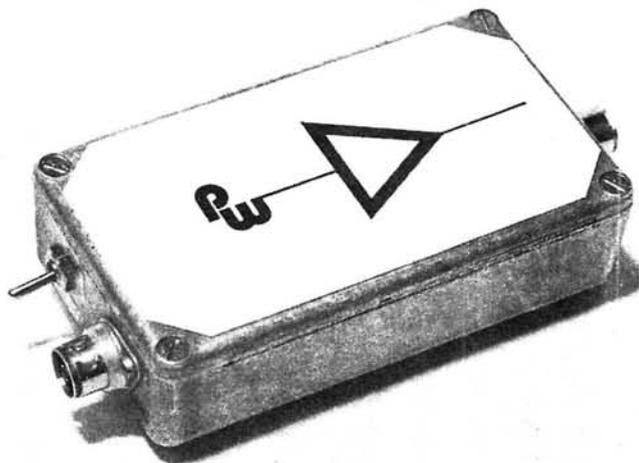
and this, together with the very high transition frequency (2GHz at 10mA collector current) of the specified transistor, ensures a flat response over a very wide frequency range. Signals are capacitively coupled into and out of the stage; the values of coupling capacitor were chosen so that low frequency roll-off occurs at approximately 200kHz.
