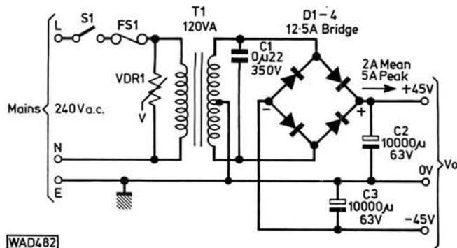
Fig. 3: Circuit of a typical high-current power supply, such as might be used in an audio amplifier
