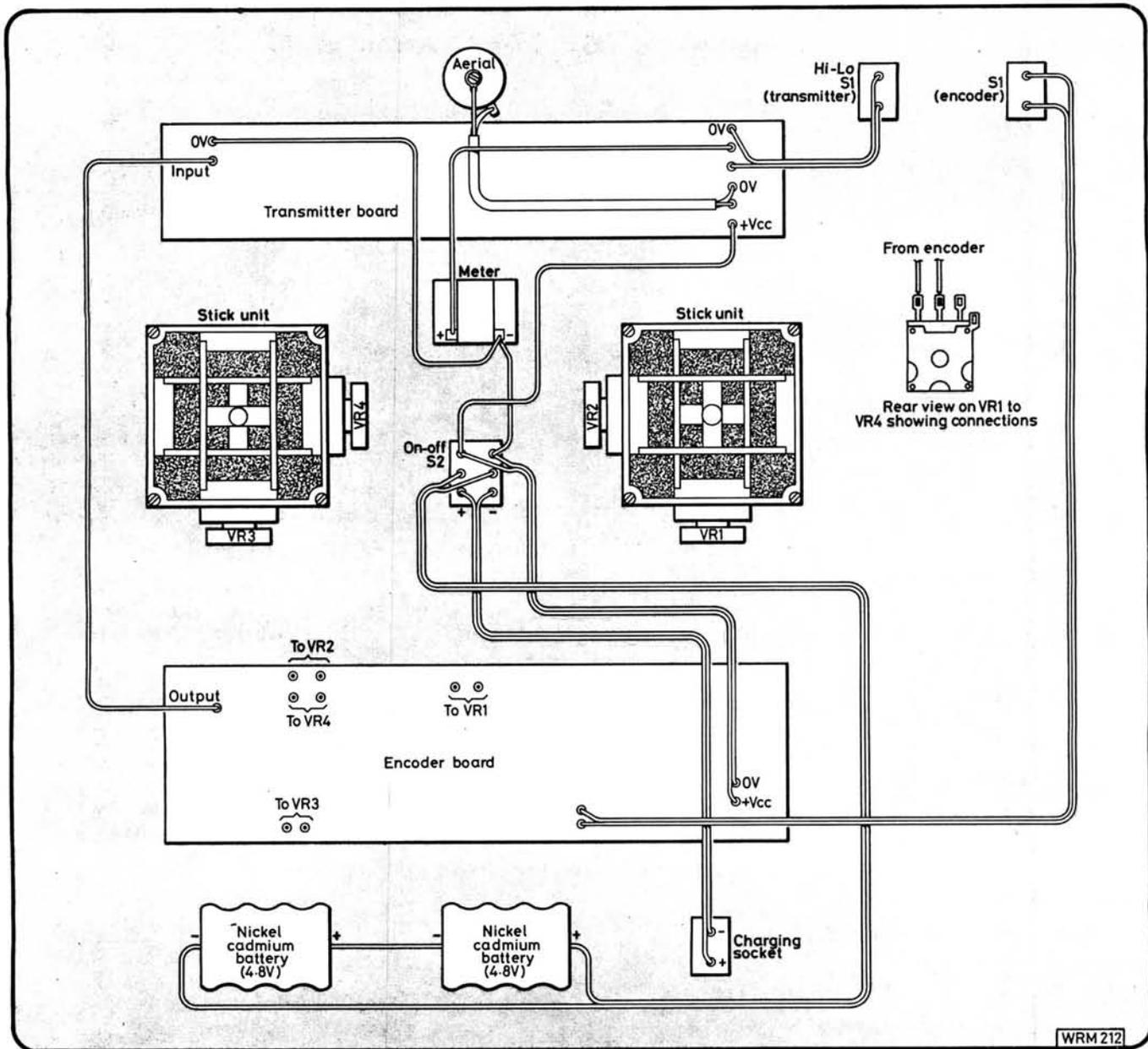
**Fig. 8: The wiring layout of the complete transmitter and encoder. Care must be taken not to short out the battery terminals. The stick unit pots VR1 to VR4 must be set to 1.5kΩ before connecting wires are attached**
