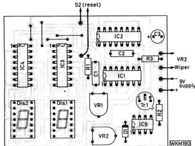
Fig. 3: Layout of the components on the p.c.b.
