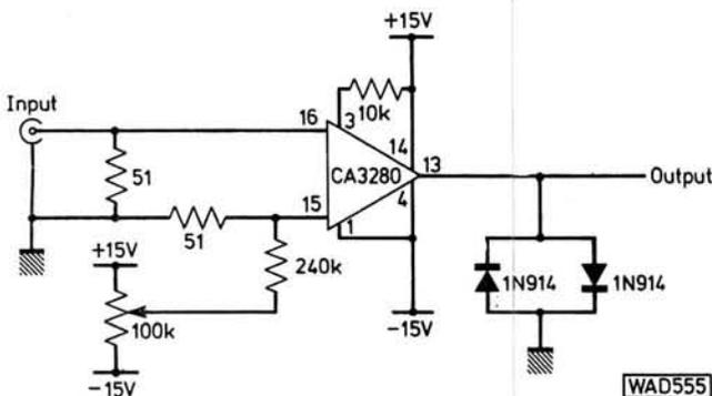
Fig. 7: Fast comparator circuit
