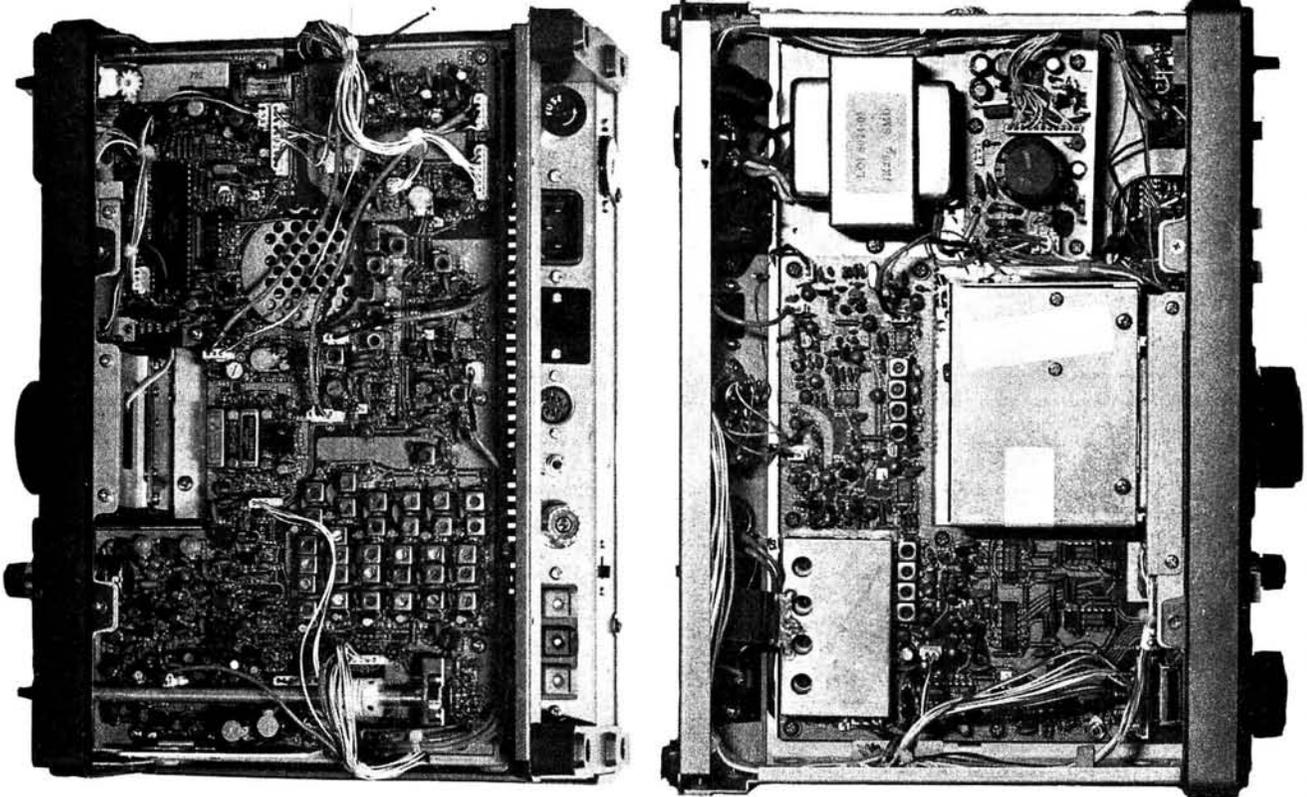
A bottom view, showing the p.i.l. synthesiser board, v.f.o. and power supply. All p.c.b.-mounted component references are marked on the board
