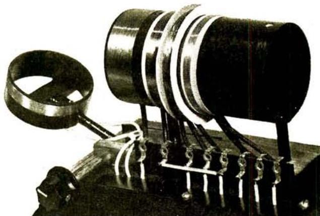
Fig. 5: Coil winding details. The main tuning coil with the swinging reaction coil is shown above with L1 shown below
