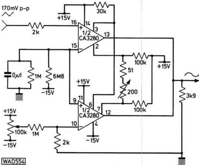
Fig. 6: Triangle-sine converter
