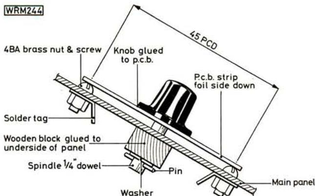
Fig. 3: Constructional details of the stud switches. Further details can be seen in the photograph below
