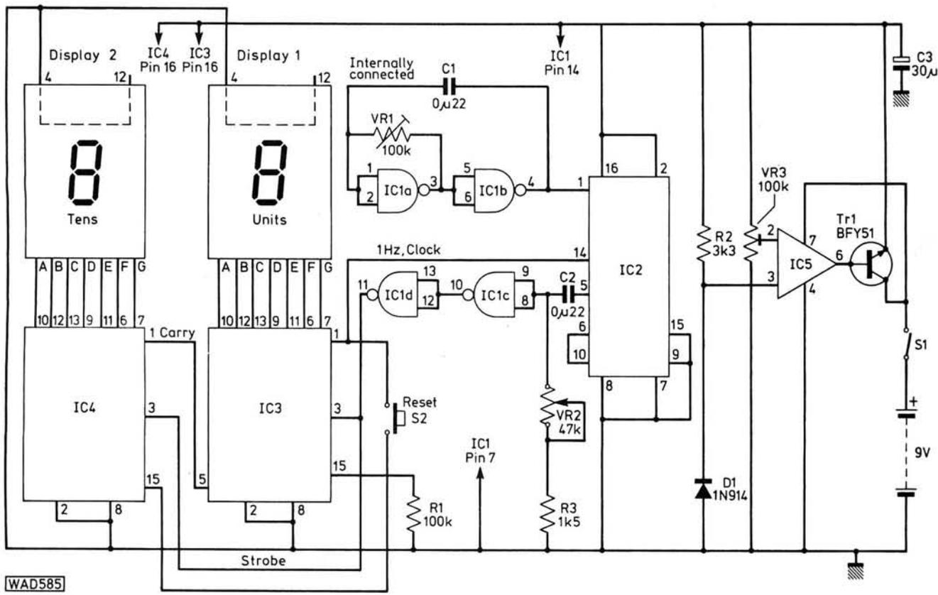
Fig. 1: The complete circuit diagram
