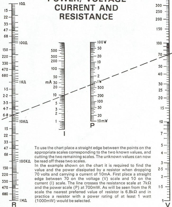
To use the chart place a straight edge between the points on the appropriate scales corresponding to the two known values, and cutting the two remaining scales. The unknown values can now be read off these two scales.
